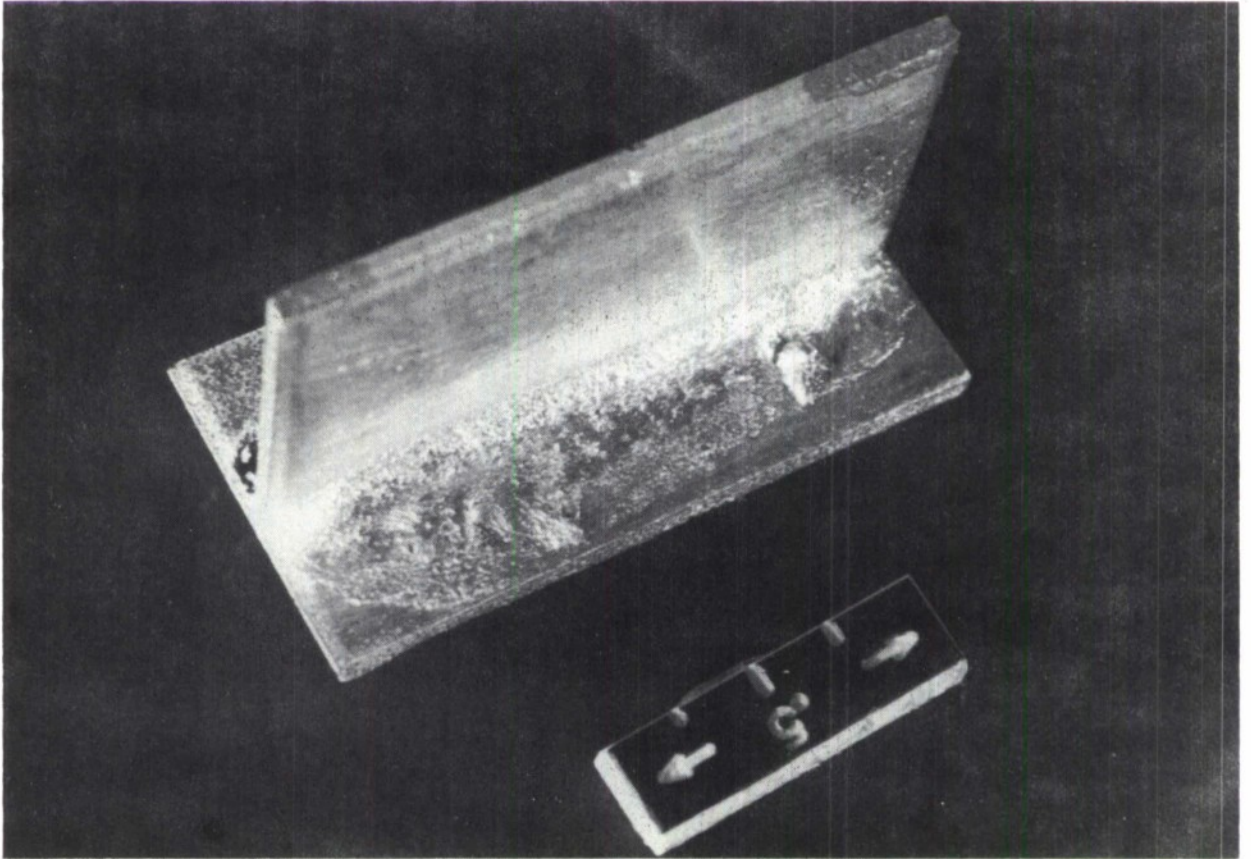
Figure 12. Y-97407 T-Joint of Al-Si-Ge Alloy No. 9 and 6061 Base Metal (The brazing was performed at 1020°F for 2-1/2 min. Excellent flow is evident.)
