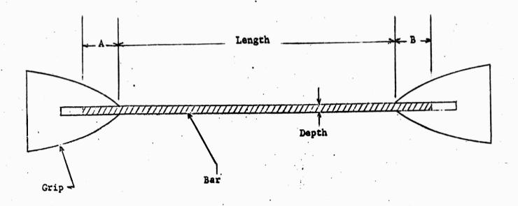
Labels A and B indicate the length of the bar was used for the gripping. These values will be given below each remaining group of tables.
