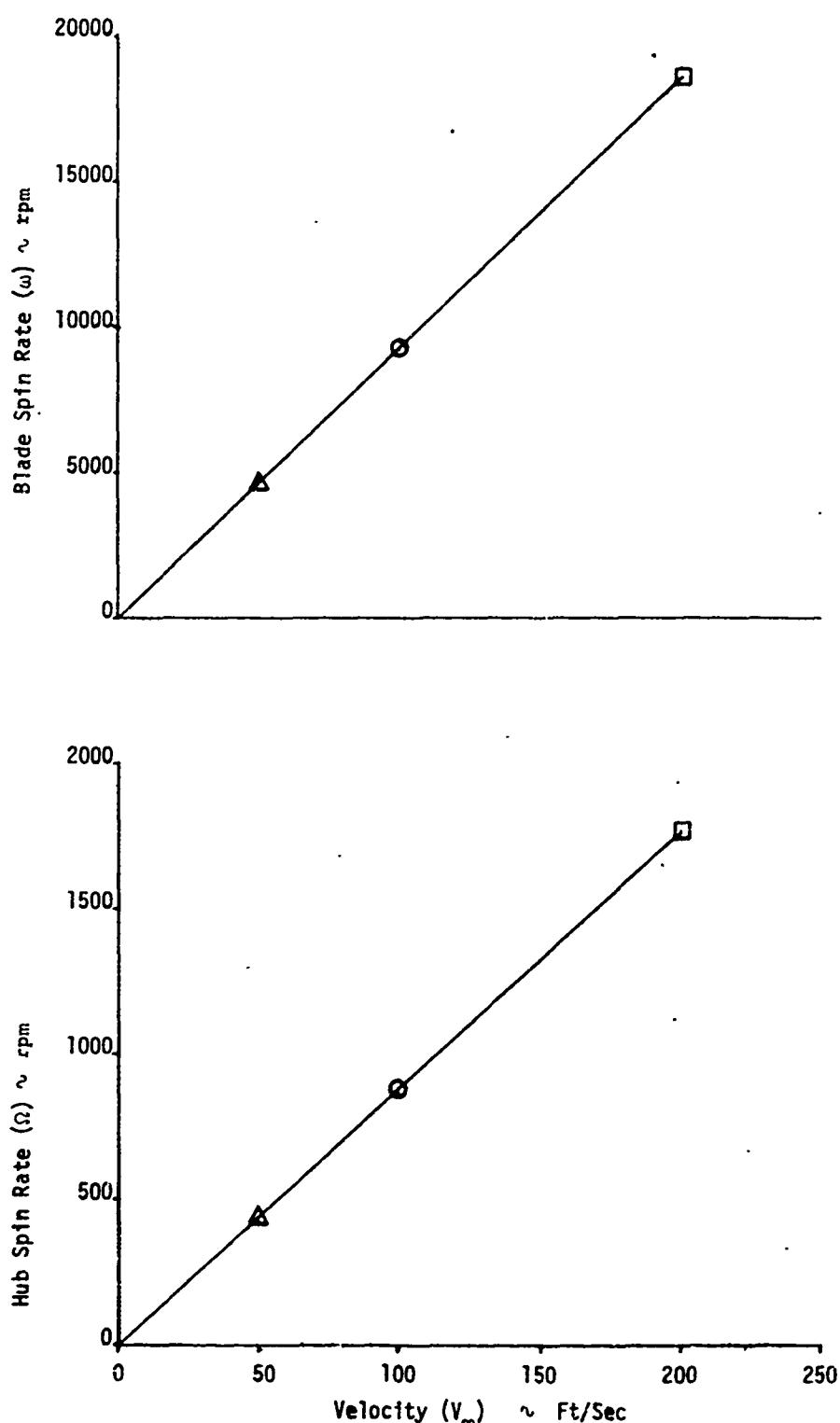
Figure 64. Effect of Free Stream Velocity on Steady State Blade Spin Rate and Hub Spin Rate
