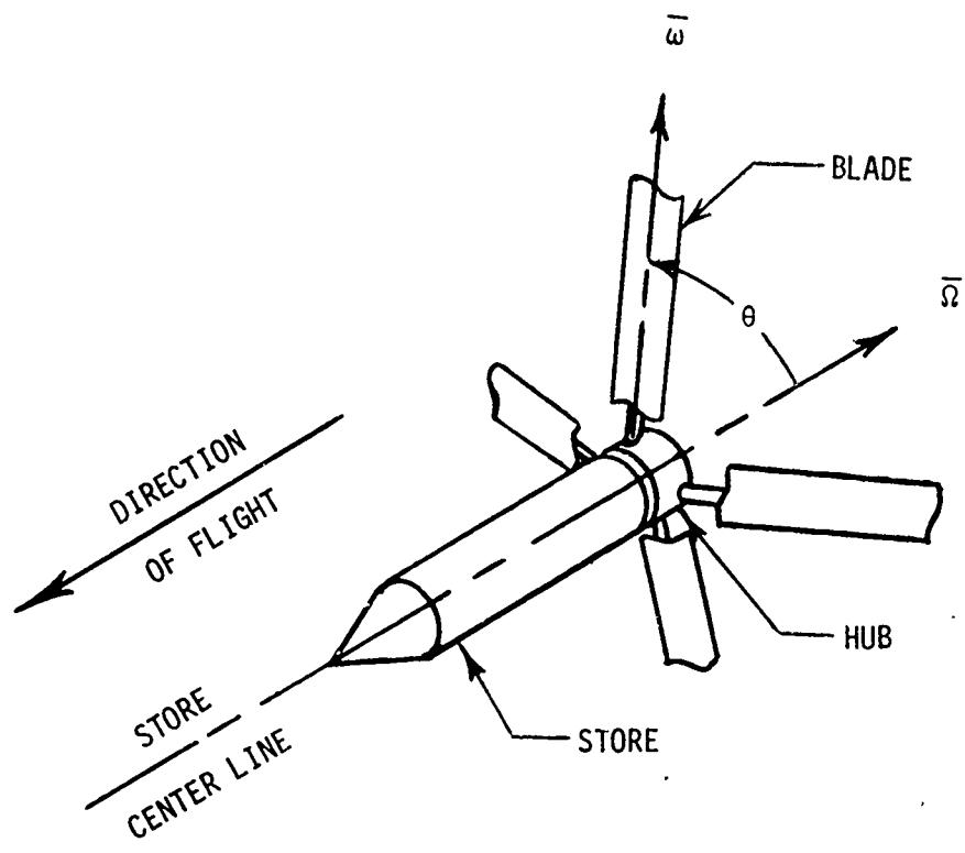
Figure 1. General Configuration of Articulated Autorotor Decelerator System
