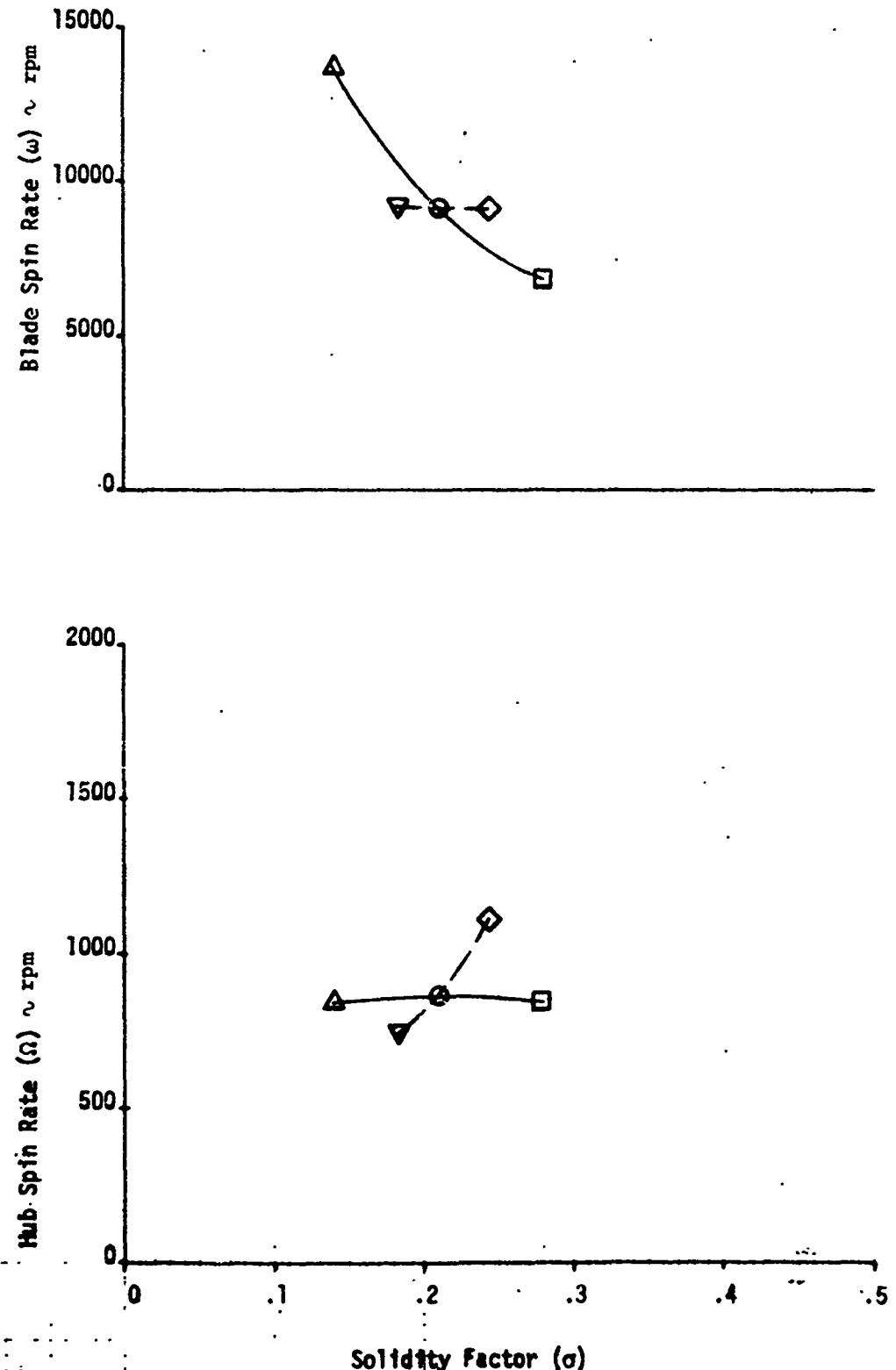
Figure 60. Effect of Solidity Factor on Steady State Blade Spin Rate and Hub Spin Rate
