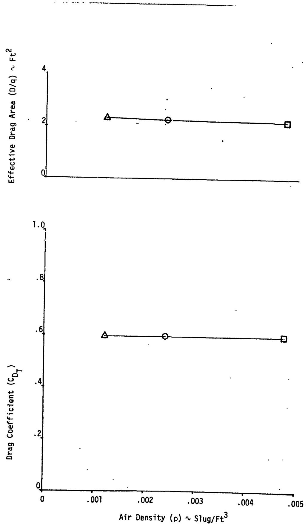
Figure 69. Effect of Air Density on Steady State Effective Drag Area and Drag Coefficient
