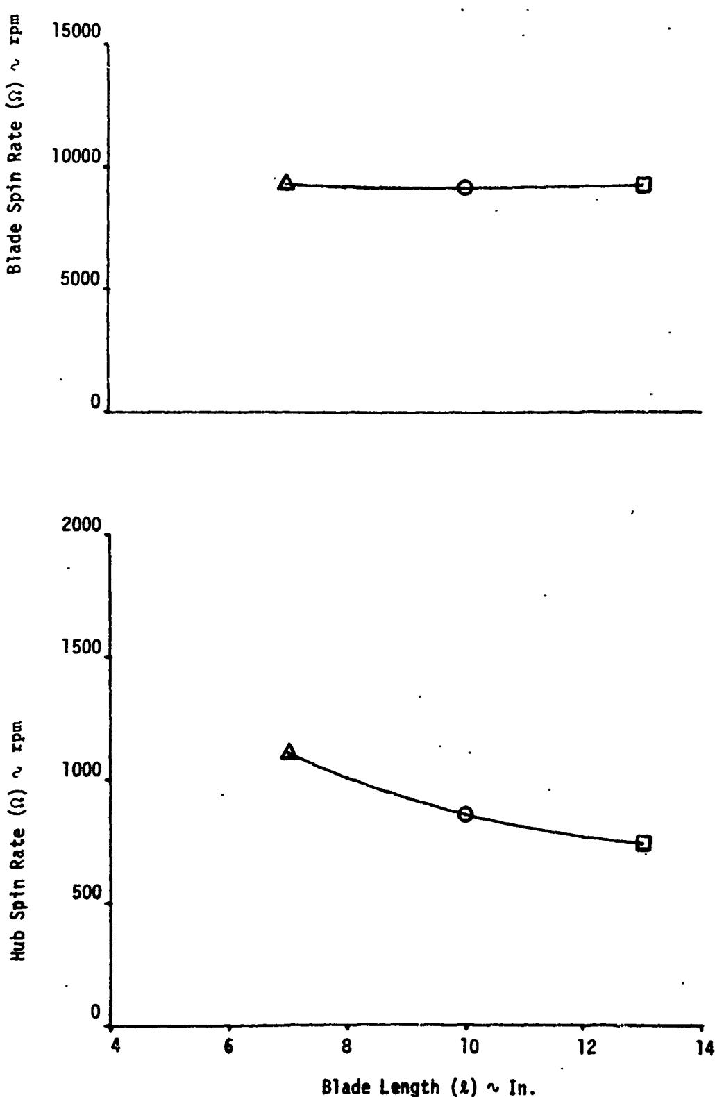
Figure 52. Effect of Blade Length on Steady State Blade Spin Rate and Hub Spin Rate
