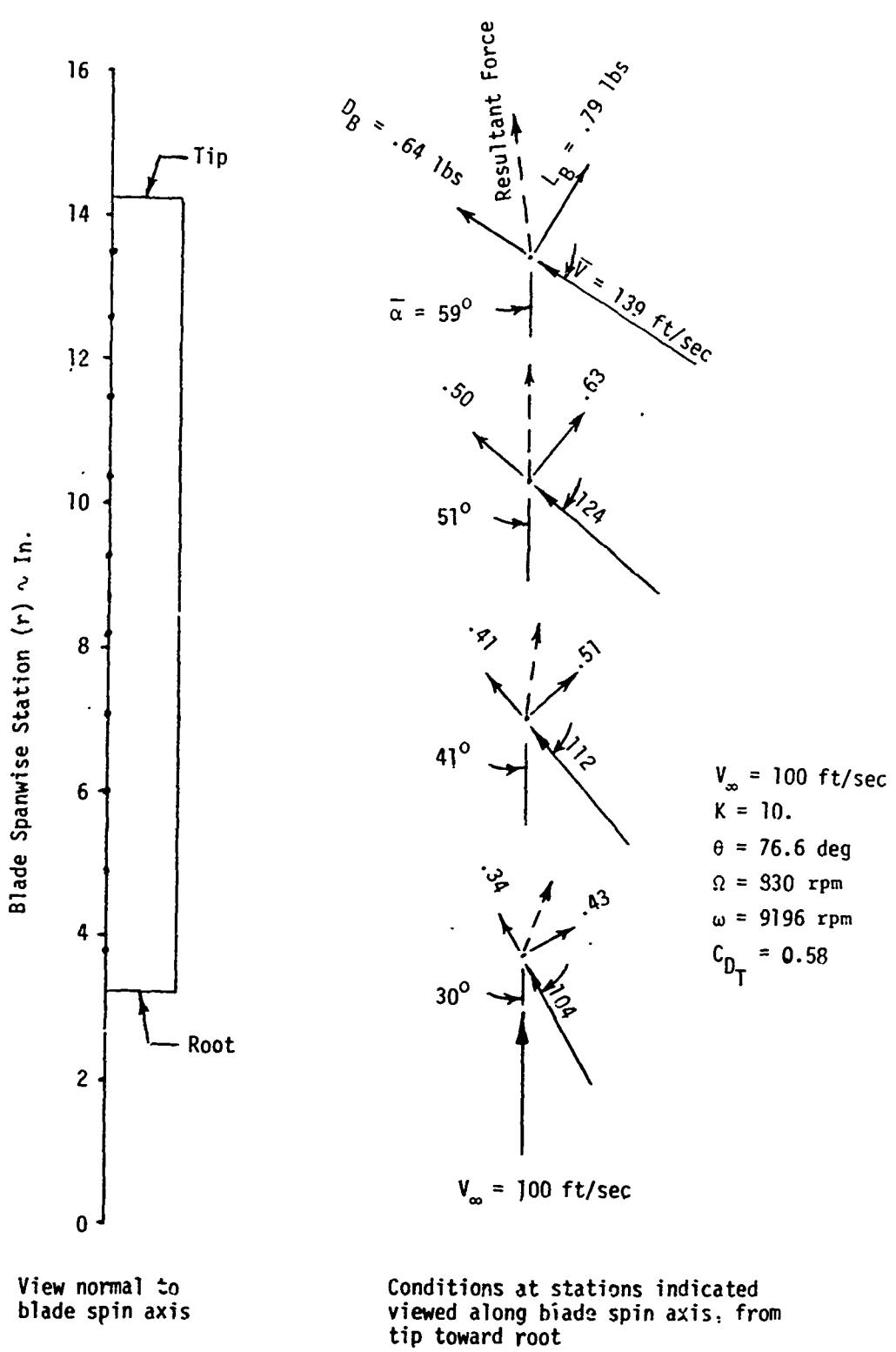
Figure 42. Aerodynamic Conditions at Various Blade Spanwise Stations at Steady
