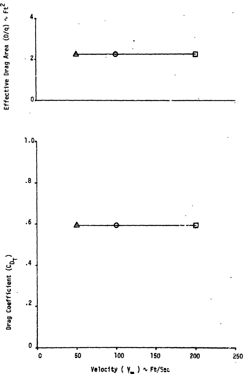
Figure 65. Effect of Free Stream Velocity on Steady State Effective Drag Area and Drag Coefficient
