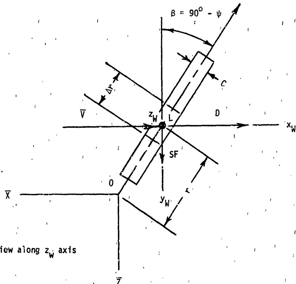
Figure 6. Details of Blade Element Terminology
