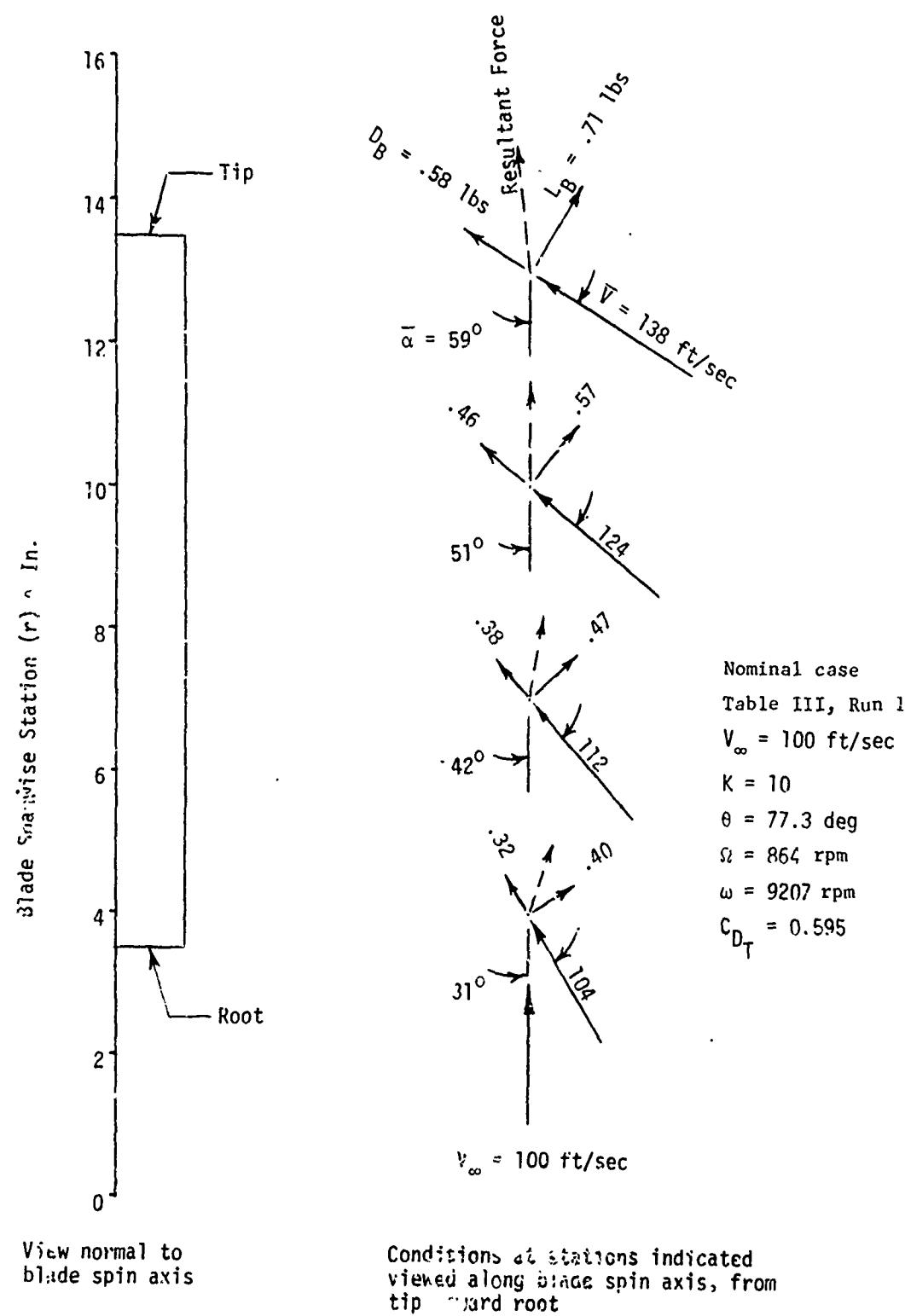
Figure 8c. Steam; State Aerodynamic Conditions at Various Blade Stations for the Nominal Case
