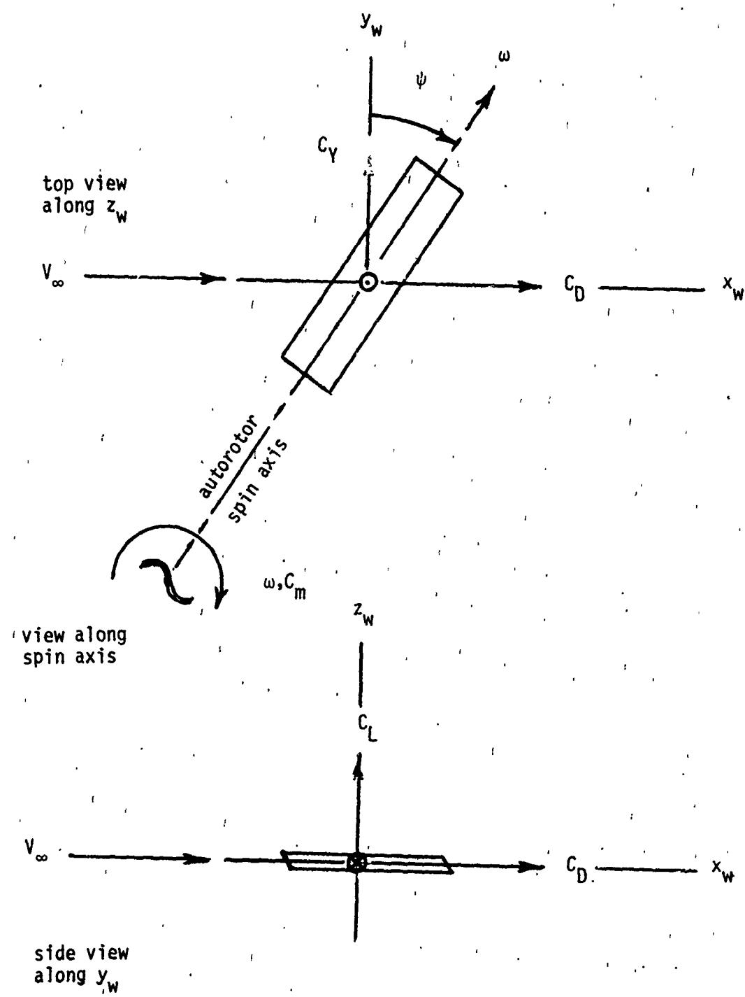
Figure 14. Definitions of Wind Tunnel Axes Systems and Aerodynamic Nomenclature
