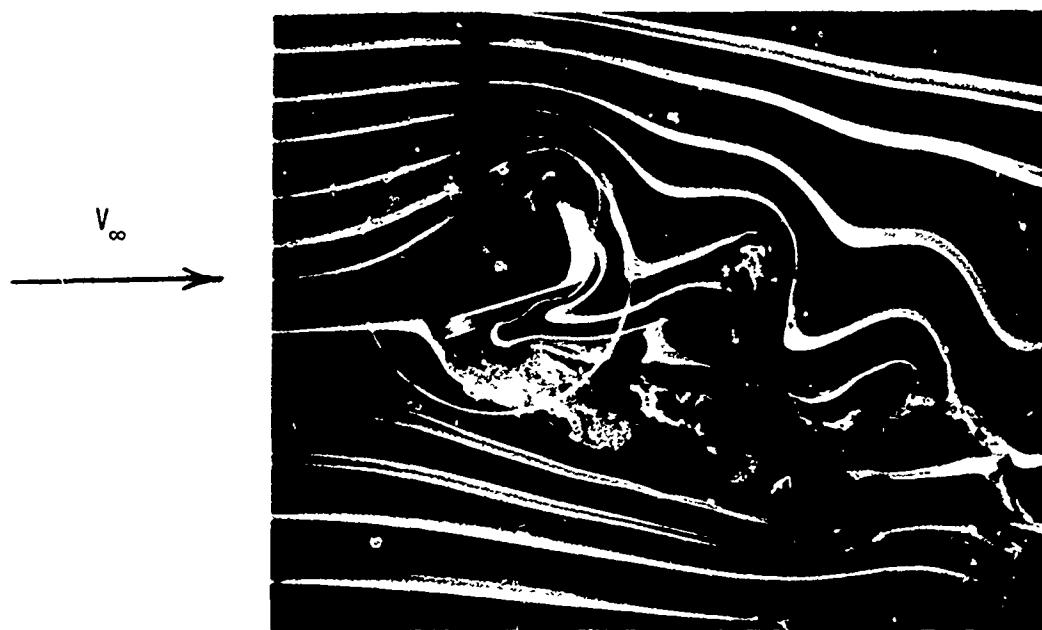
Figure 38. Typical Flow Field Around a Single Autorotor
