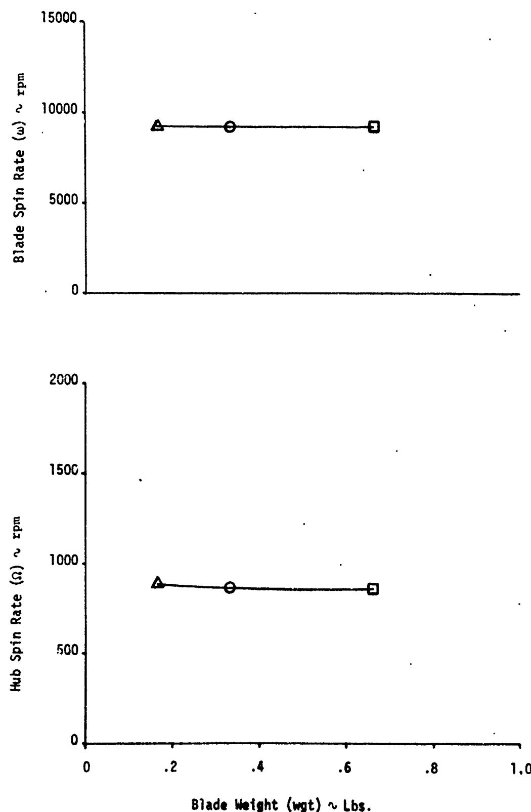
Figure 48. Effect of Blade Weight on Steady State Blade Spin Rate and Hub Spin Rate
