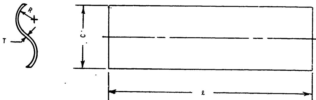
Figure 11. S-Section Autorotor Configuration
