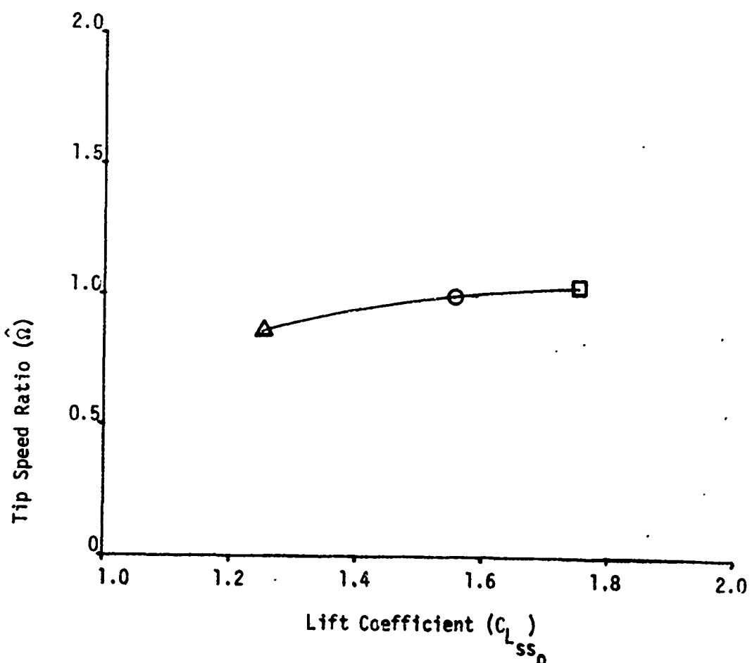
Figure 74. Effect of Blade Sectional Maximum Lift Coefficient on Steady State Tip Speed Ratio
