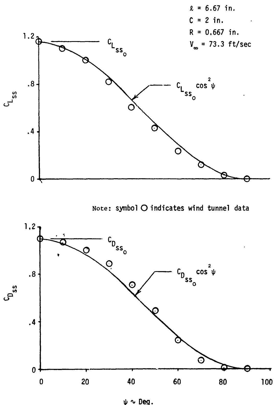
Figure 15. Aerodynamic Characteristics as a Function of Angle of Attack
