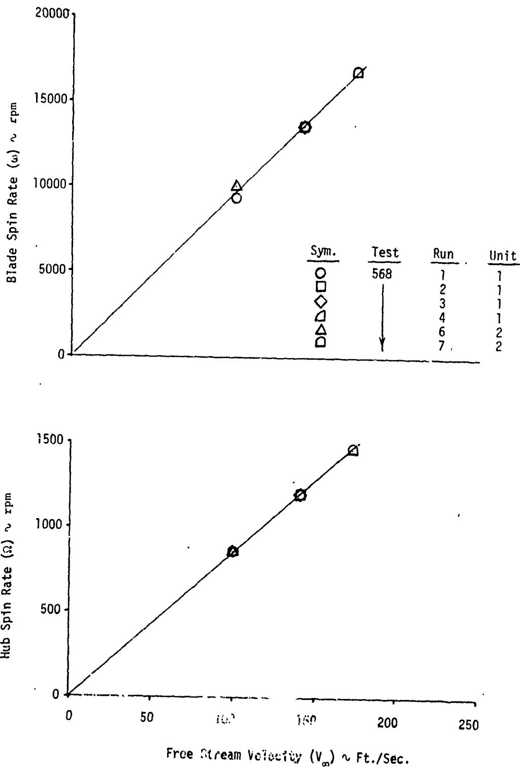
Figure 34. Steady State Blade and Hub Spin Rates as Determined From Wind Tunnel Tests on a Full-Scale Autorotor Accelerator
