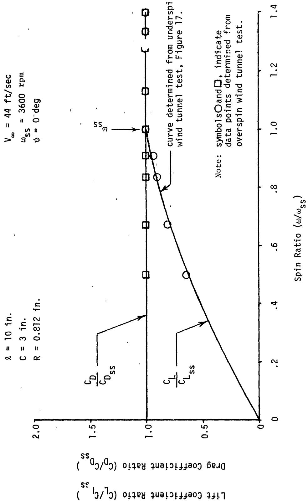
Figure 22. Results From Wind Tunnel Test to Determine Effect of Autorotor Overspin on the Lift and Drag Coefficients
