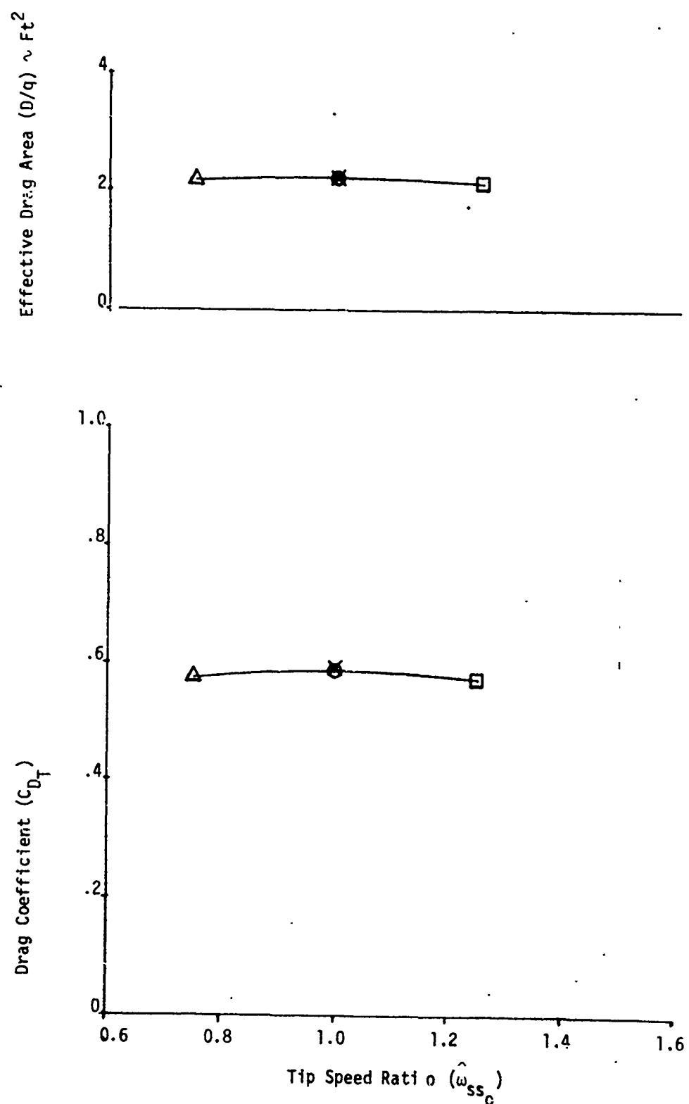
Figure 73. Effect of Blade Sectional Steady State Tip Speed Ratio on Steady State Effective Drag Area and Drag Coefficient
