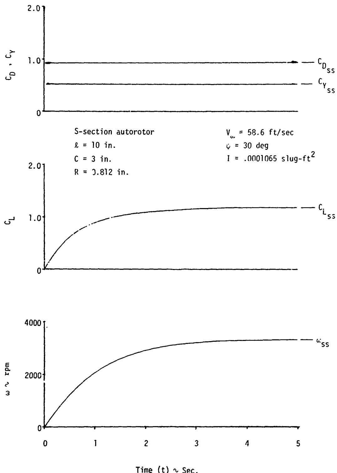
Figure 16. Typical Autorotor Aerodynamic Characteristics During Spinup Transient
