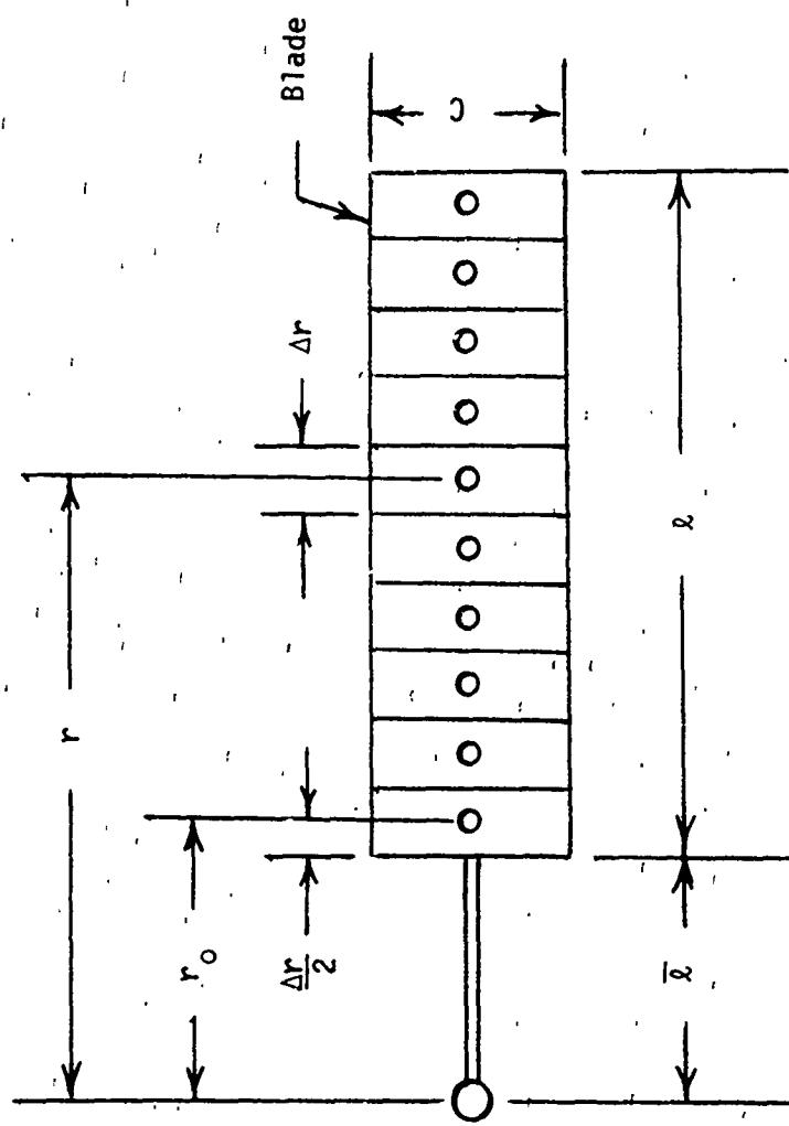
Figure 28. Definitions of Terms Used in Blade Element Method
