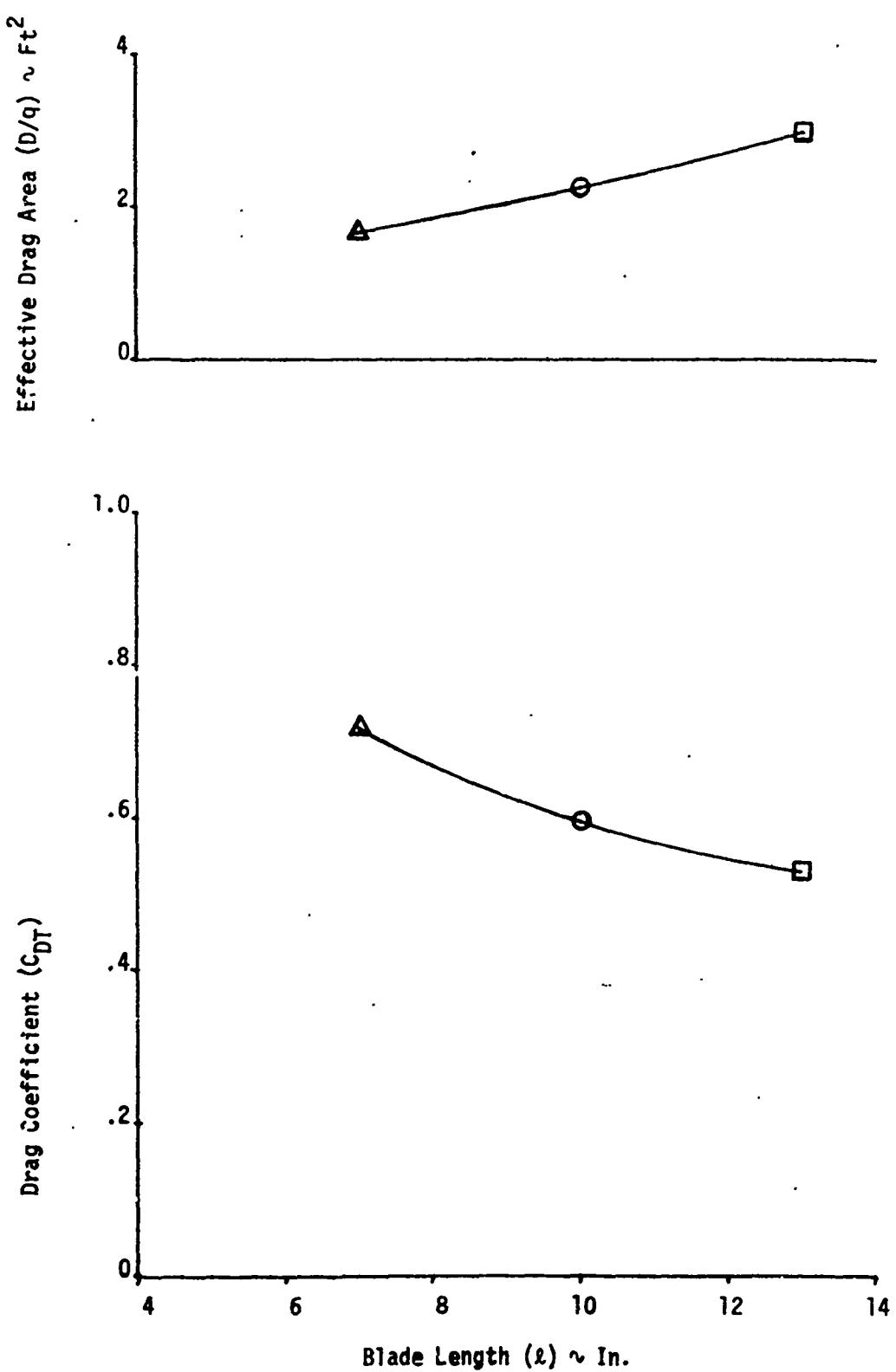
Figure 53. Effect of Blade Length on Steady State Effective Drag Area and Drag Coefficient
