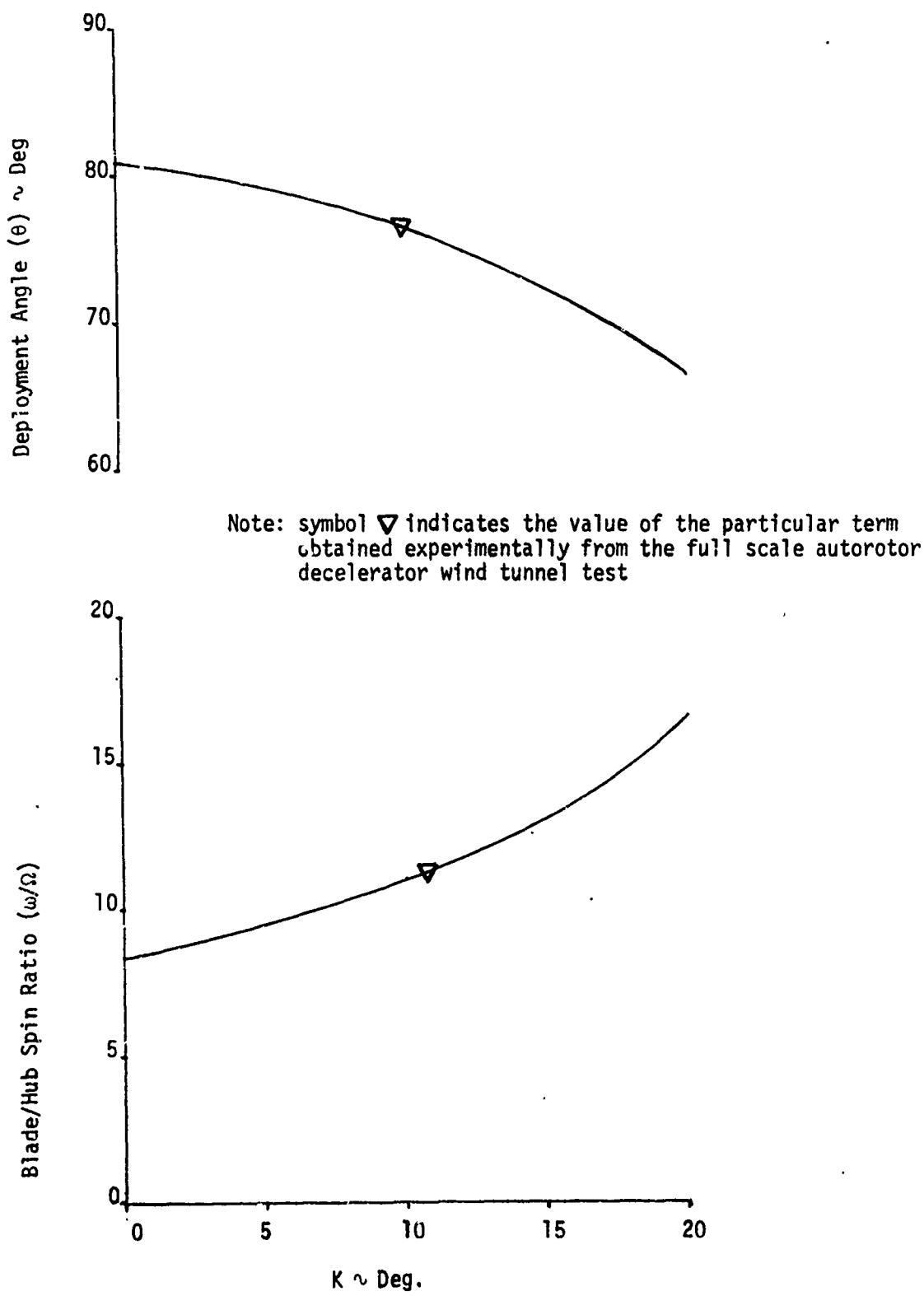
Figure 40. Steady State Performance of Full-Scale Autorotor Decelerator Computed as a Function of Interference Factor ( $K$ ) for a Free Stream Velocity of 141 Ft/Sec
