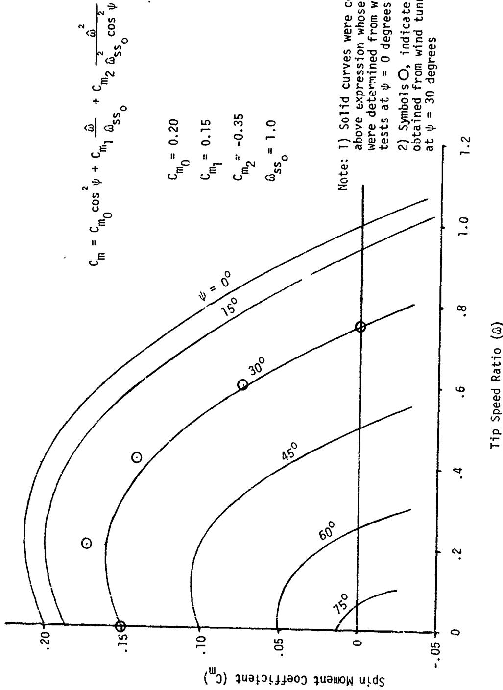
Figure 20. Spin Moment Coefficient as a Function of Tip Speed Ratio and Yaw Angle for an S-Section Autorotor
