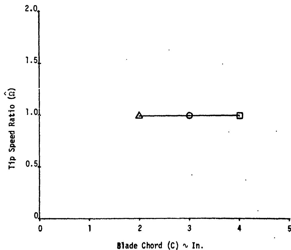
Figure 54. Effect of Blade Chord on Steady State Tip Speed Ratio
