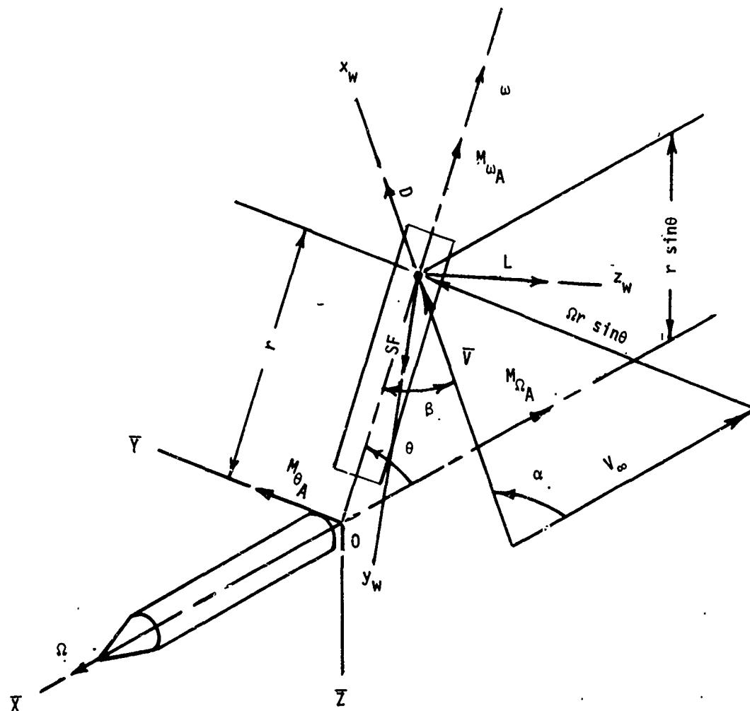
Figure 5. Aerodynamic Conditions at a Typical Blade Element
