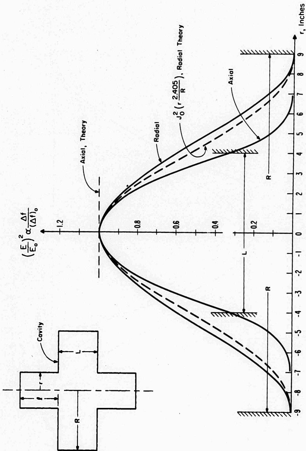
$R = 9''$ ,  $L = 8''$ ,  $r = 2.75''$ ,  $f = 8.375''$ ,  $f_0 = 509 \text{ MHz}$ ,  $(\Delta f)_0 = 59 \text{ kHz}$
