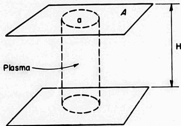
Figure C-3. THE CAVITY-PLASMA ANALOGUE
