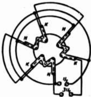
Figure 1-1. A schematic showing the connections of the windings of a "cable" pulse transformer with the transformation ratio n = 3 .
