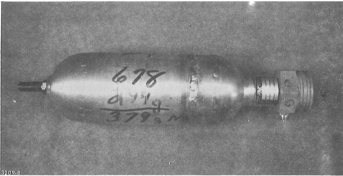
Figure 25. Cylinder for Polystyrene Foam Solution Equipped with Automatic Dump Valve
