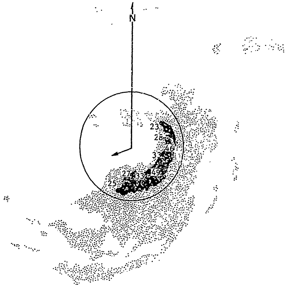
Figure K-7. Hurricane Inez, 4 October 1966, 0750 EST, UM/10-cm PPI with IEC; heights in k ft from MPS-4; circle includes eyewall precipitation; eye diameter 20 miles.
