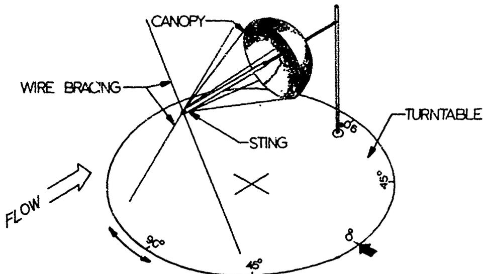
FIG D-7. TEST SECTION ASSEMBLY WITH STING ONLY, NO DRAG LINK
