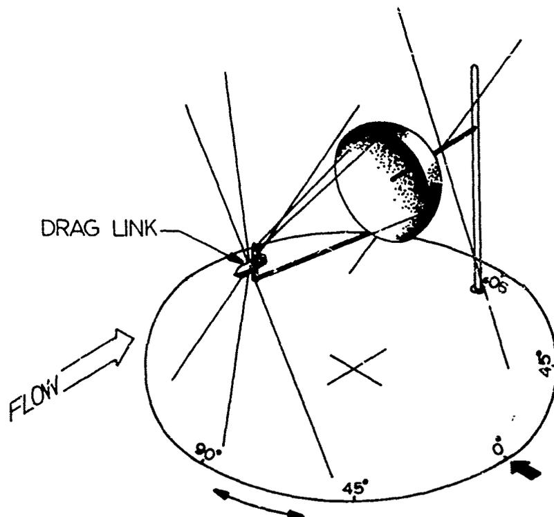
FIG D-3. TEST SECTION ASSEMBLY WITH DRAG LINK, NO STING
