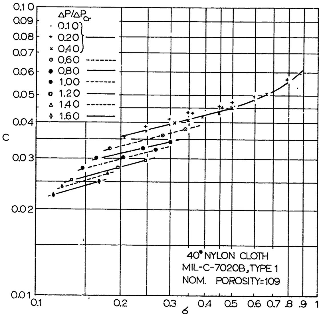
FIG 8. EFFECTIVE POROSITY VERSUS DENSITY RATIO (REF. 1)
