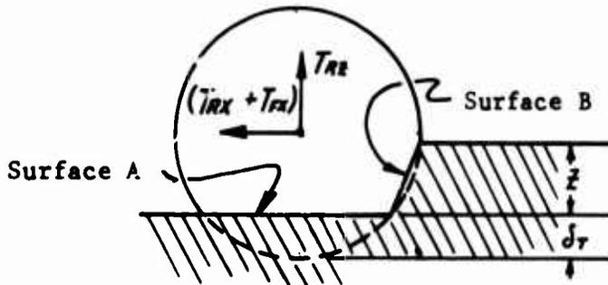
The tire forces associated with surface A are those defined in Paragraph 3.4.1 as  $T_R$  and  $T_{FX}$ . Three additional tire forces,  $T_{Sz}$ ,  $T_{RTx}$ , and  $T_{ix}$  result from the soft terrain.
