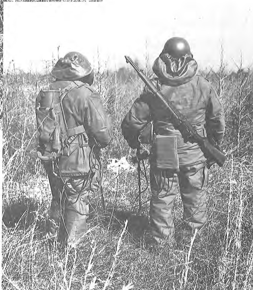
FIG. 11 MINE CLEARANCE ARMOR WORN UNDER THE COLD-WET UNIFORM AND WITH TWO TYPES OF MINE DETECTORS. THE INSET SHOWS THE ARMOR AND KIT BEING USED IN THE PRONE POSITION.
