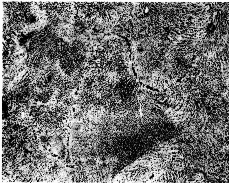
Figure 25. MAR M 509 "+". IMT 112, -8/+14 mesh, cleaned. HIP @ 2175°F, 15,000 psi, 1 hour. As pressed. Etched. 100X.
