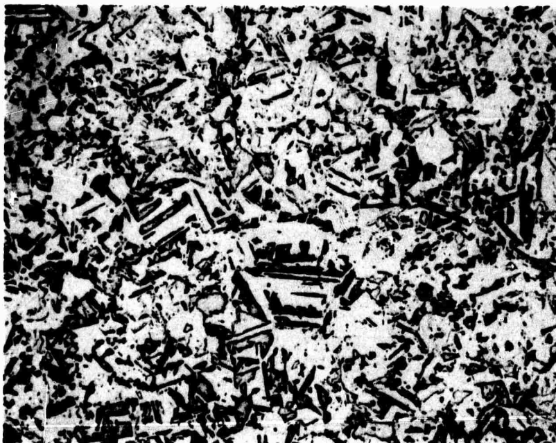
Figure 22. VM-300. Nuclear Metals, -35 mesh. HIP @ 2200°F, 14,500 psi, 1 hour. As pressed. Etched. 100X.
