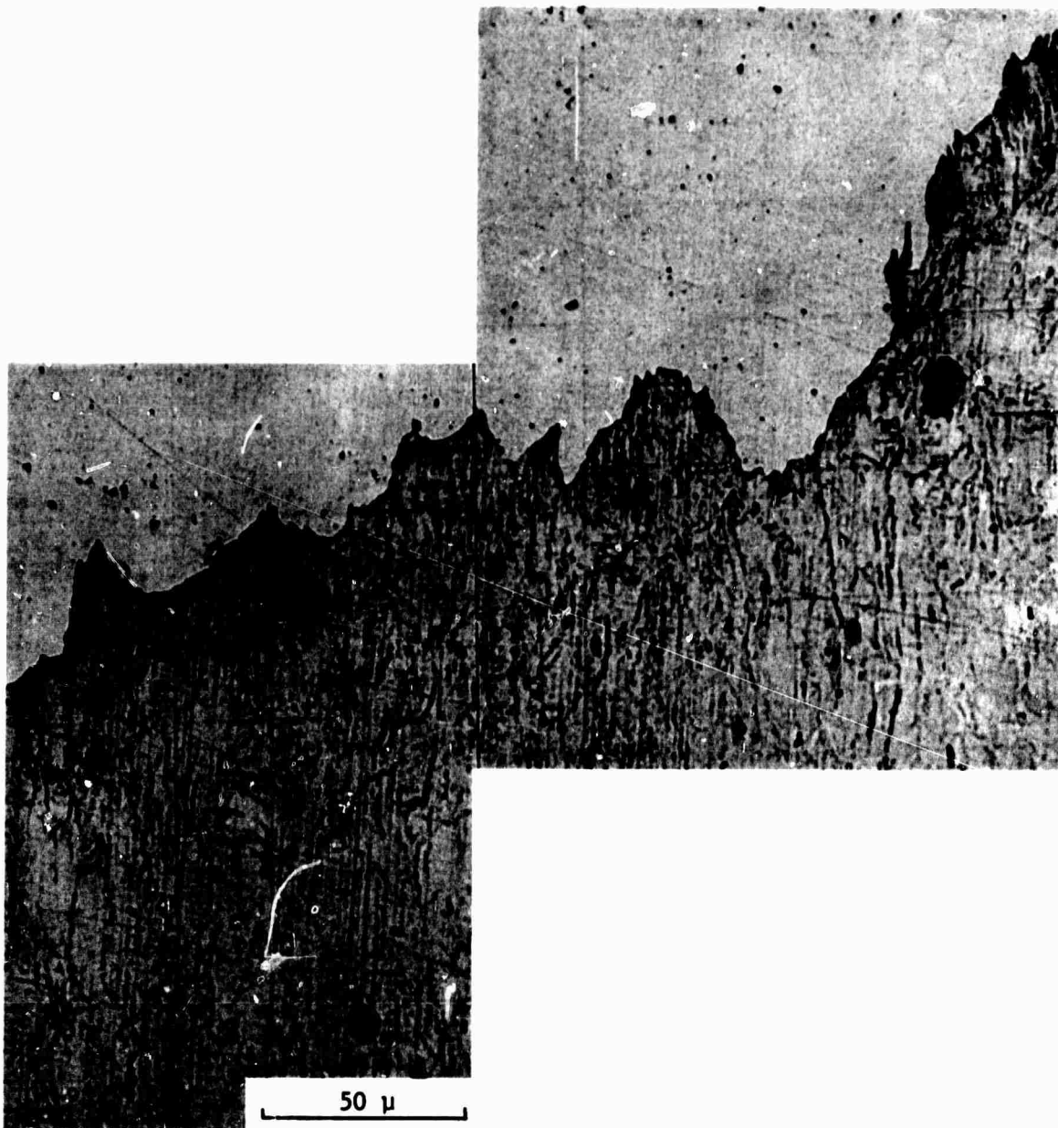
Fig. 9 Fracture surface profile of Specimen #1 of Vascom3x 300 alloy showing both the large titanium-carbide inclusions, and much smaller inclusions.
