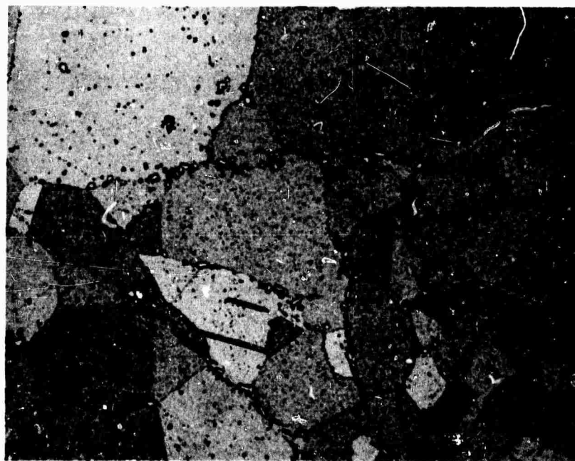
Figure 16. IN-100. Homogeneous Metals, -20/+40 mesh. HIP @ 2300 o F, 25,000 psi, 2 hours + 2200 o F solution, 4 hours. A.C. Etched. 500X.
