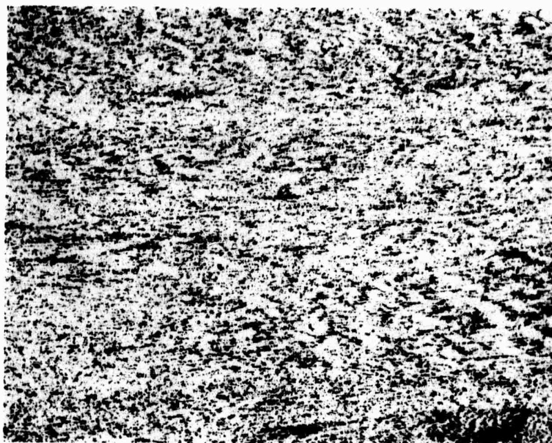
Figure 35. MAR M 509. HIP compact No. 12, Table III. Extruded 15.2 x @ 2000°F. As extruded. Longitudinal section. Etched. 100X.
