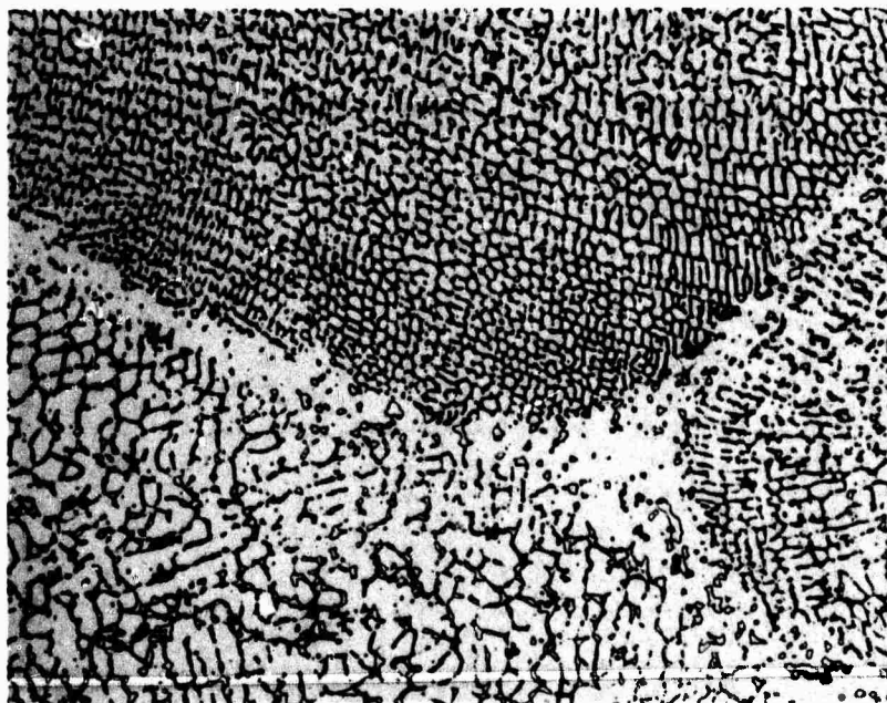
Figure 24. MAR M 509. IMT 111, -8/+14 mesh, cleaned. HIP @ 2175°F, 15,000 psi, 1 hour. As pressed. Etched. Interparticle boundaries. 500X.
