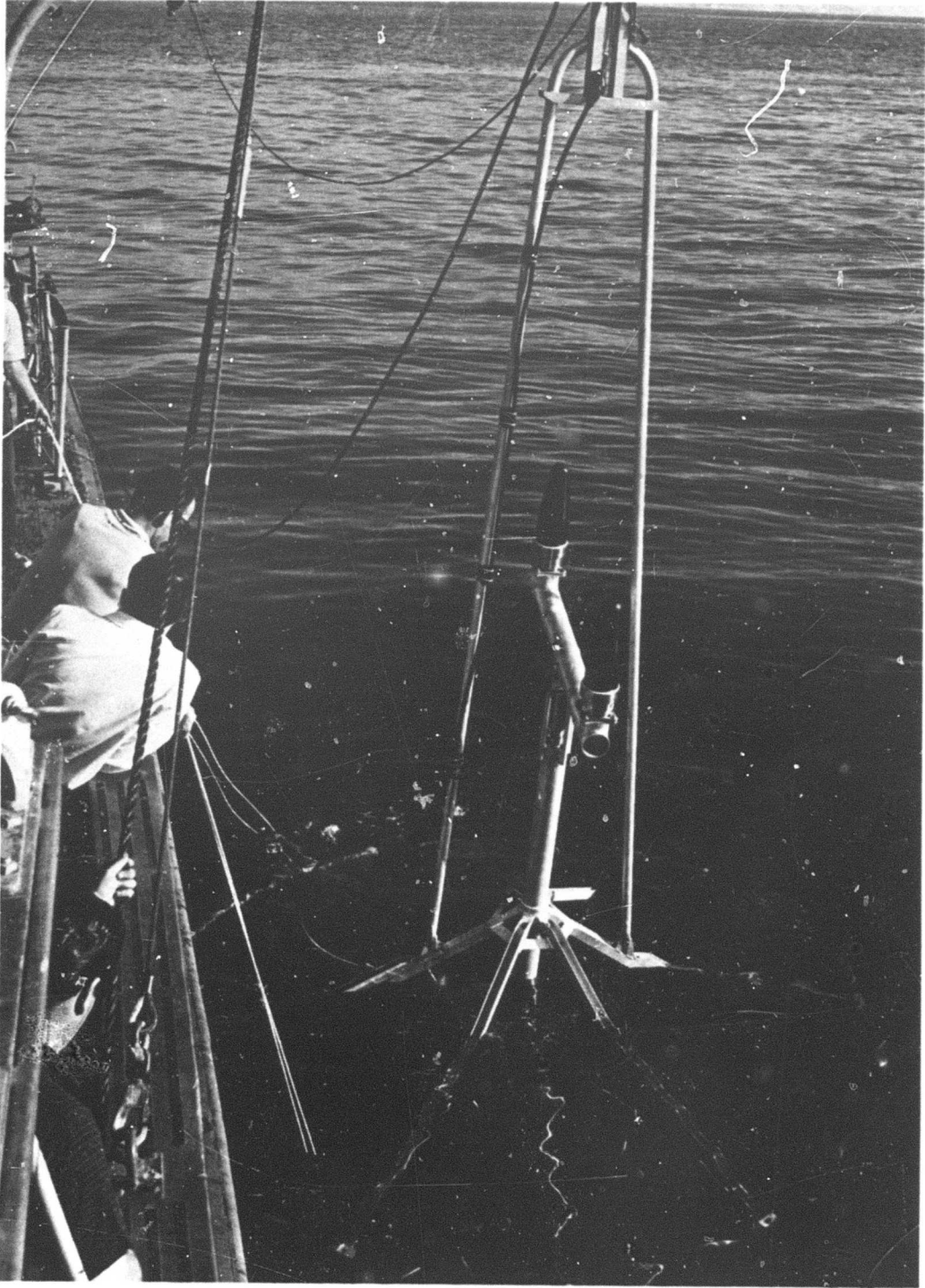
Figure 7. Typical dual hydrophone structure, SCARF range. (From Momsen, 1970. Photo courtesy of AC Electronics.)
