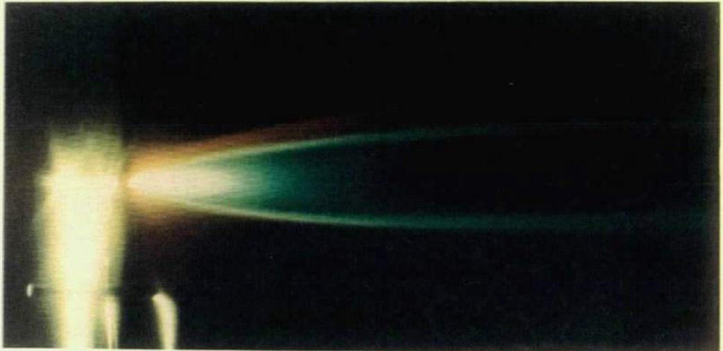
Fig. 26 Photograph of Plume for Condition IB, Tunnel M, He Plume, A_0/A^* = 25 , d^* = 0.030 in., and p_c = 450 psia
