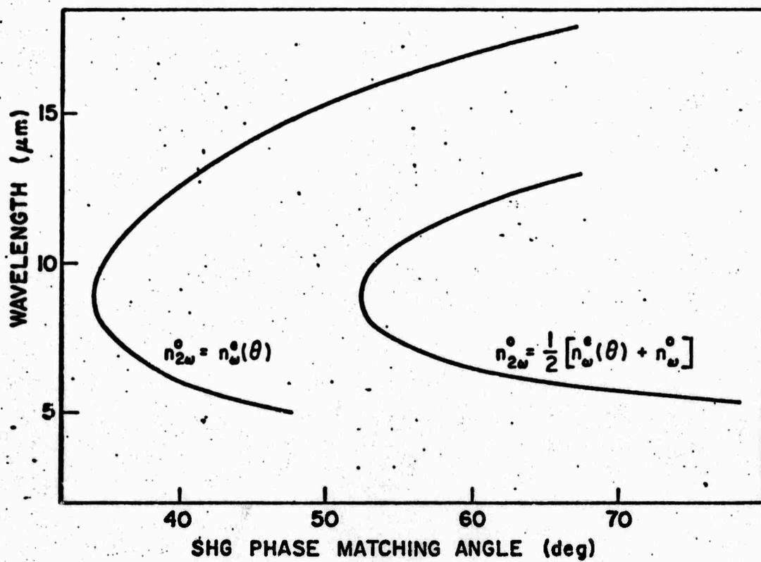
Fig. 10--PHASE MATCHING ANGLE FOR SHG IN CdGeAs<sub>2</sub>
