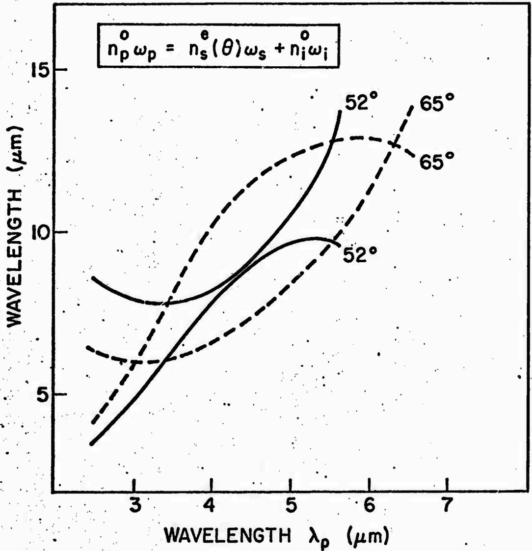
Fig. 6-- THEORETICAL TUNING CURVES FOR CdGeAs<sub>2</sub> WHEN THE PHASE MATCHING ANGLE IS FIXED
