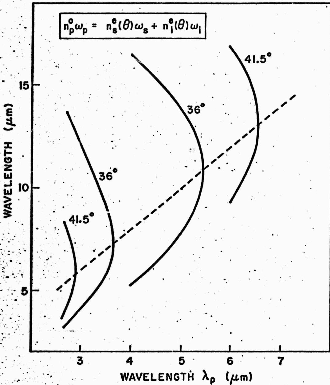
Fig. 7--THEORETICAL TUNING CURVES FOR CdGeAs<sub>2</sub> WHEN THE PHASE MATCHING ANGLE IS FIXED
