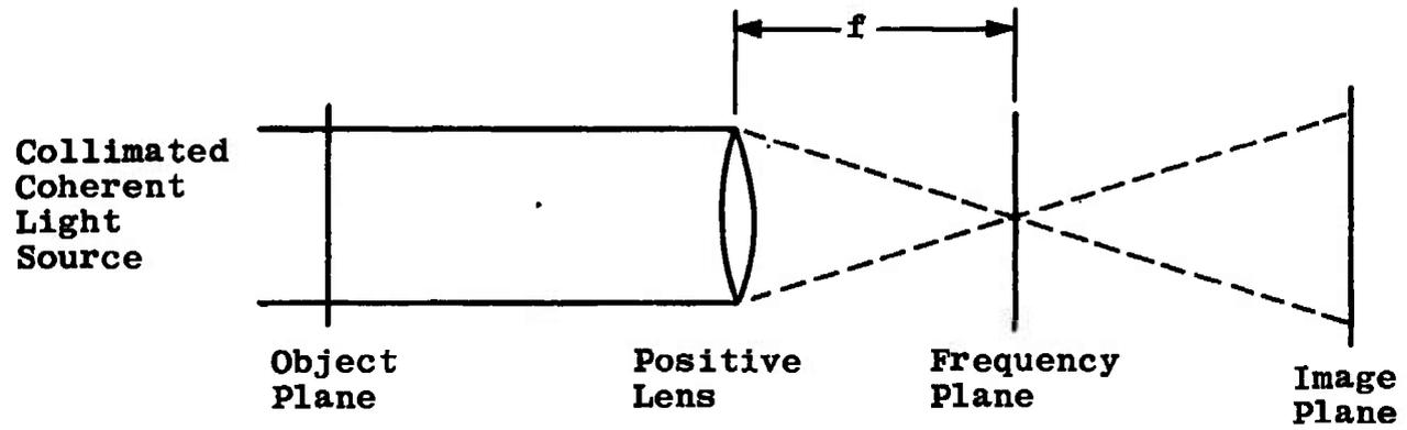
Figure 1. A simple coherent optical data processing system.
