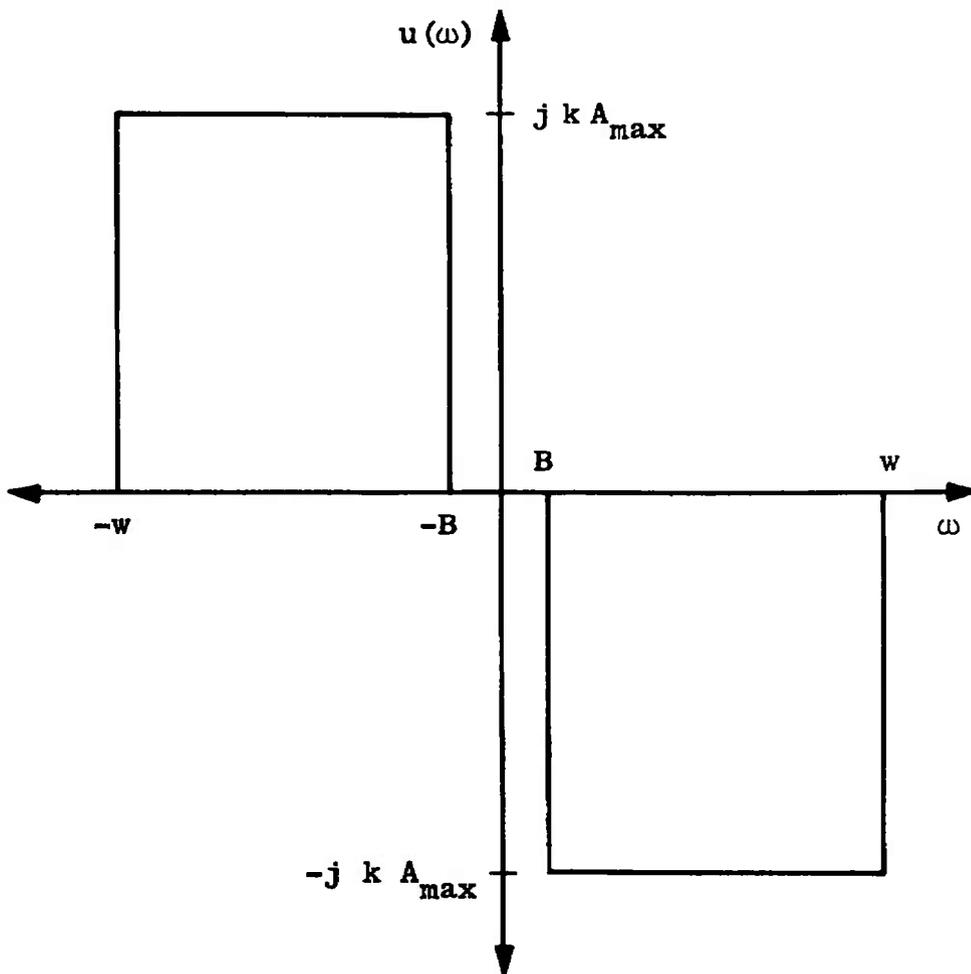
Figure 23. The frequency spectrum for the step function filtered by the filter  $A'(\omega)$ .
