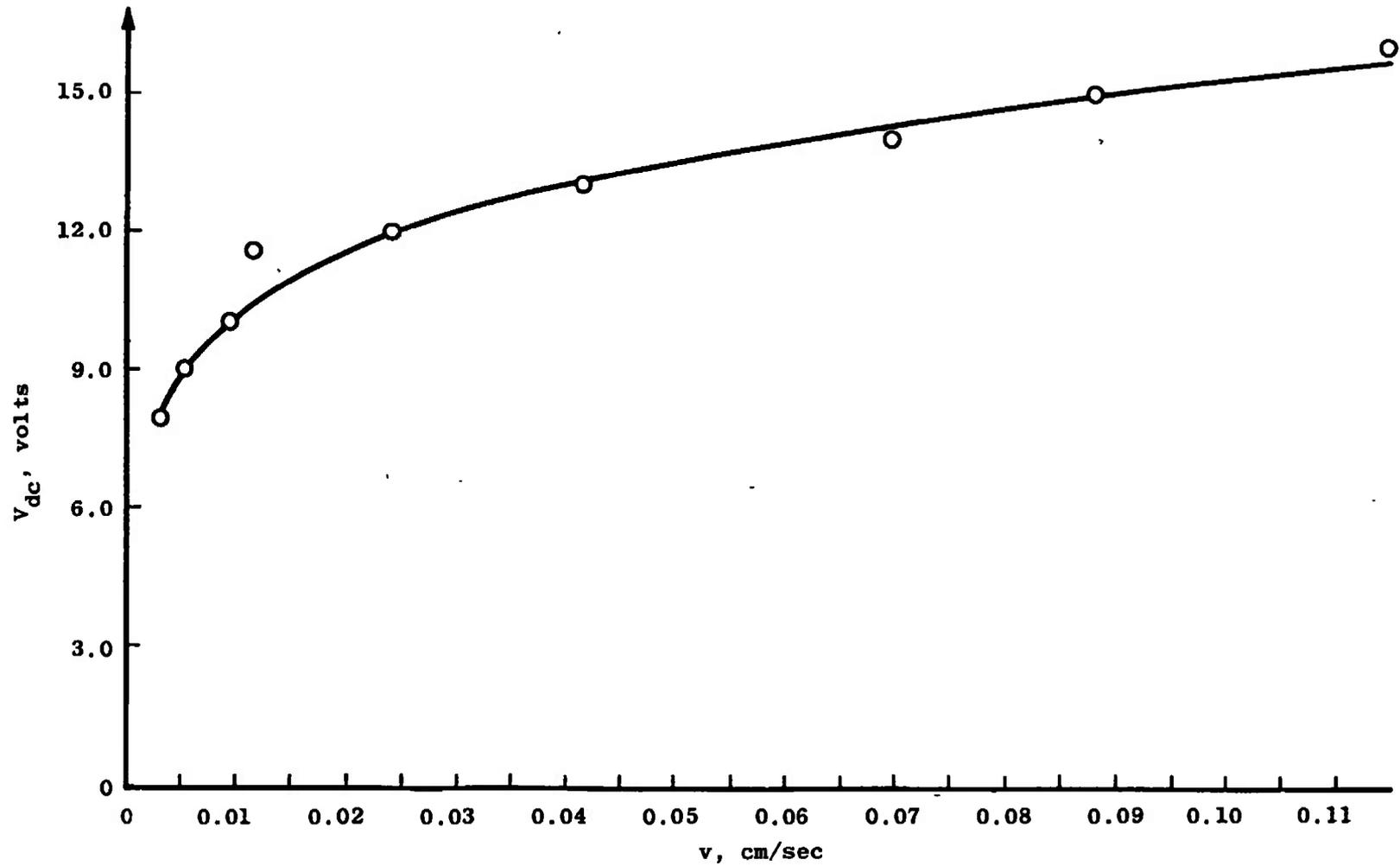
Figure 11. Input voltage versus edge velocity for pulse motor control.
