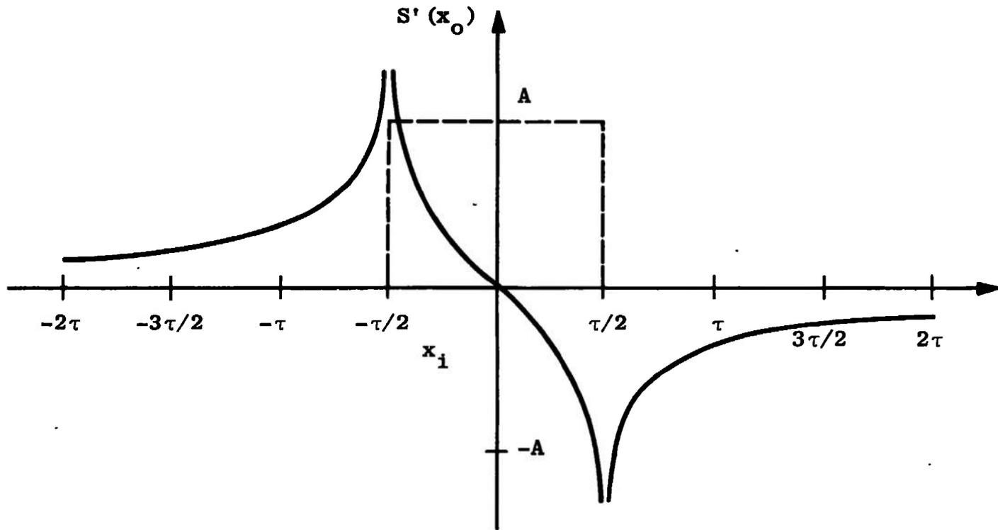
Figure 25. The plot of  $A/\pi \ln \left| x_i - \frac{\tau}{2} / x_i + \frac{\tau}{2} \right|$
