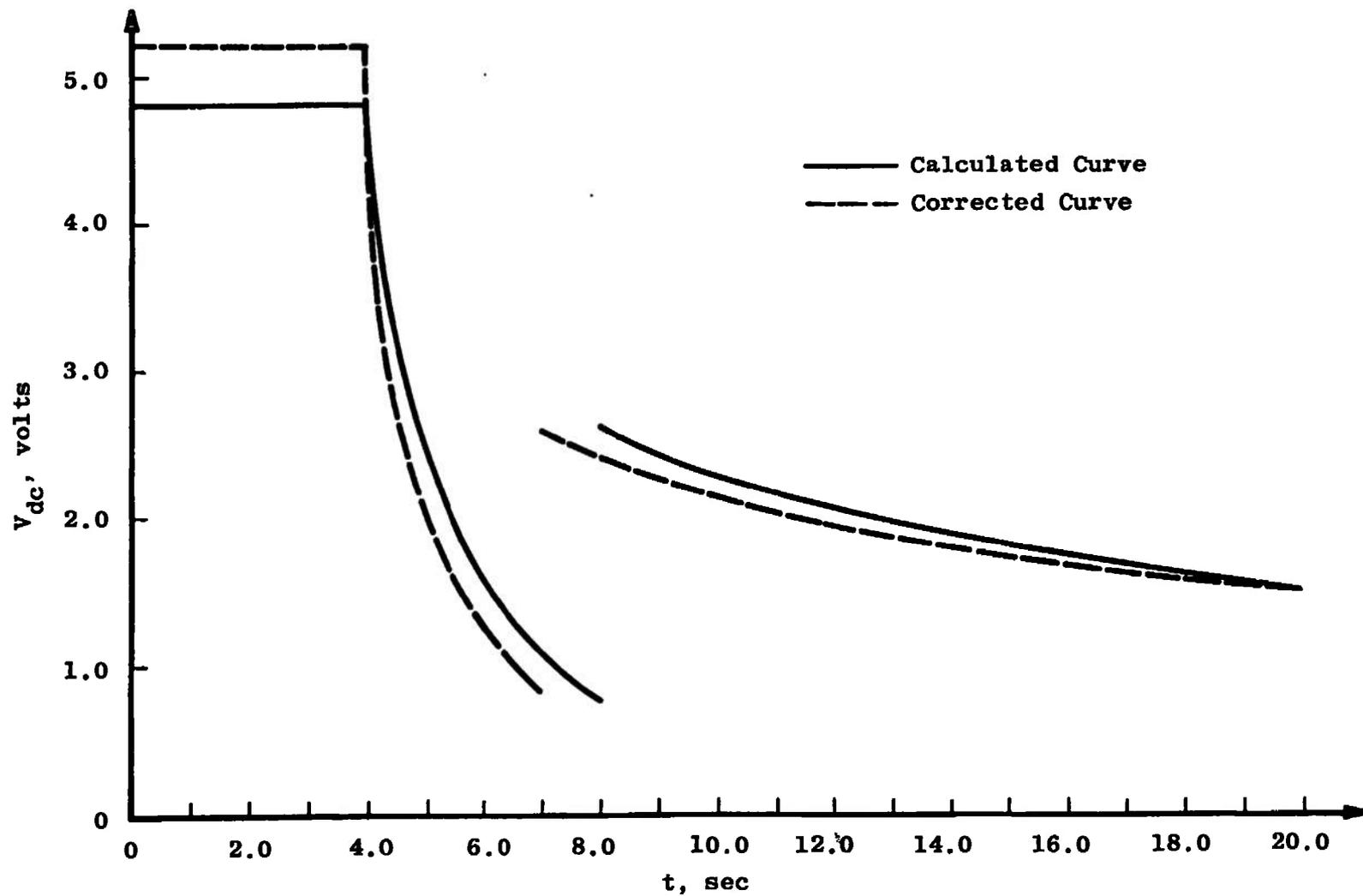
Figure 12. Voltage-exposure curve for fabrication of the filter A'(x<sub>f</sub>).
