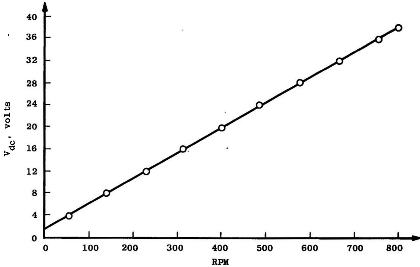
Figure 10. Velocity characteristics of the D. C. motor.
