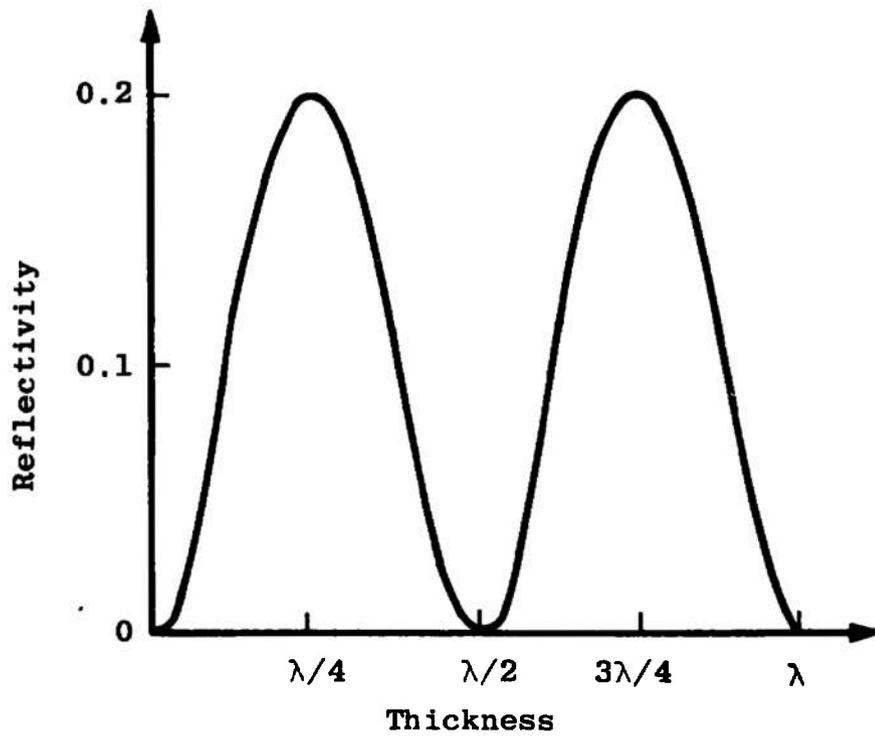
Figure 16. The reflectivity of a dielectric coating on glass for  $n_b = 2.0$ .
