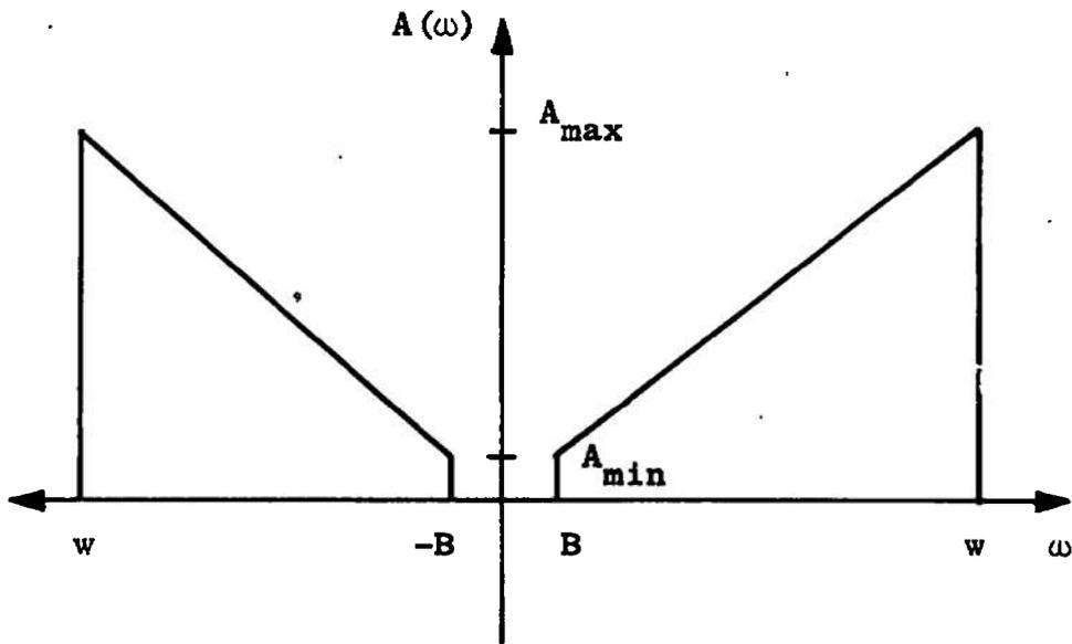
Figure 4. The linear amplitude filter  $A'(\omega)$ .
