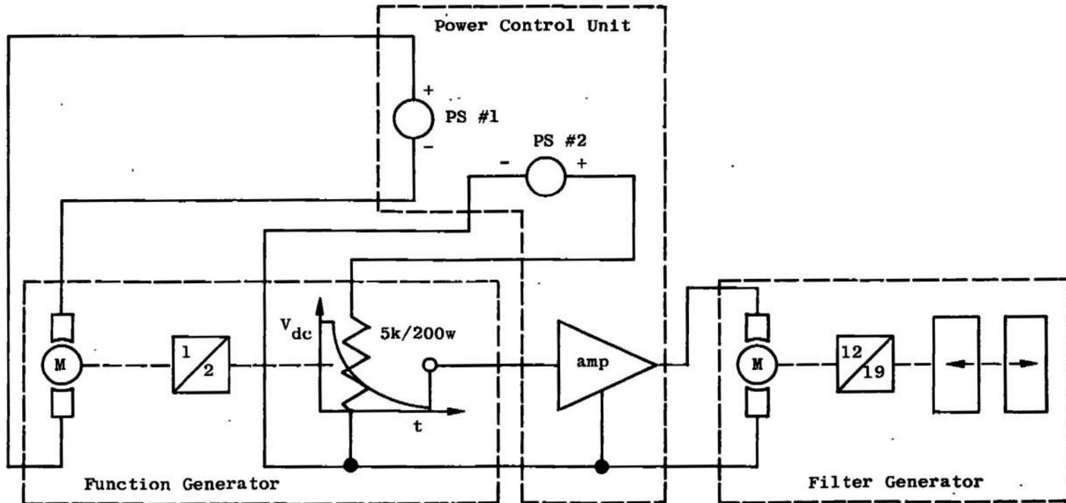
Figure 14. Block diagram of apparatus used for generating the filter  $A'(x_f)$ .
