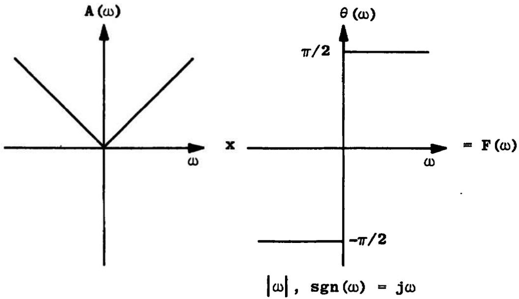
Figure 2. The differential filter.
