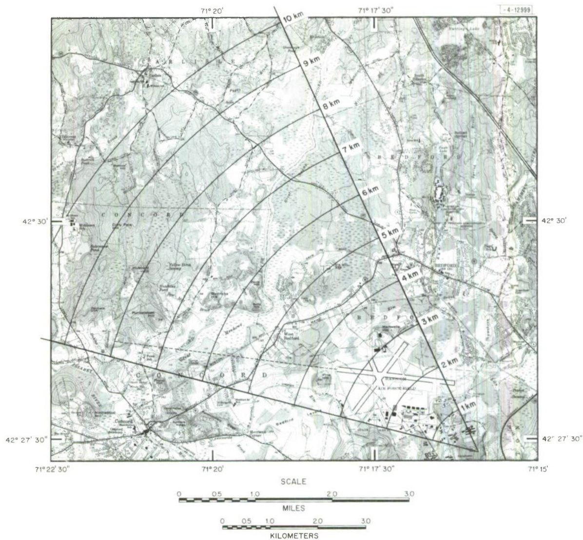
Fig. 1(b). Surveillance coverage diagram of MTI radar showing ILS Runway 11 at L. G. Hanscom Field.
