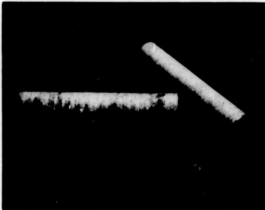
Figure 1: Westerly granite specimens used in this investigation
