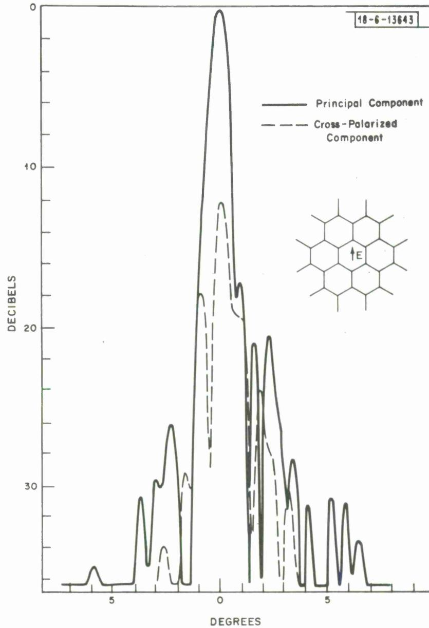
Fig. 9. Superimposed principal and cross-polarized H-plane pattern.
