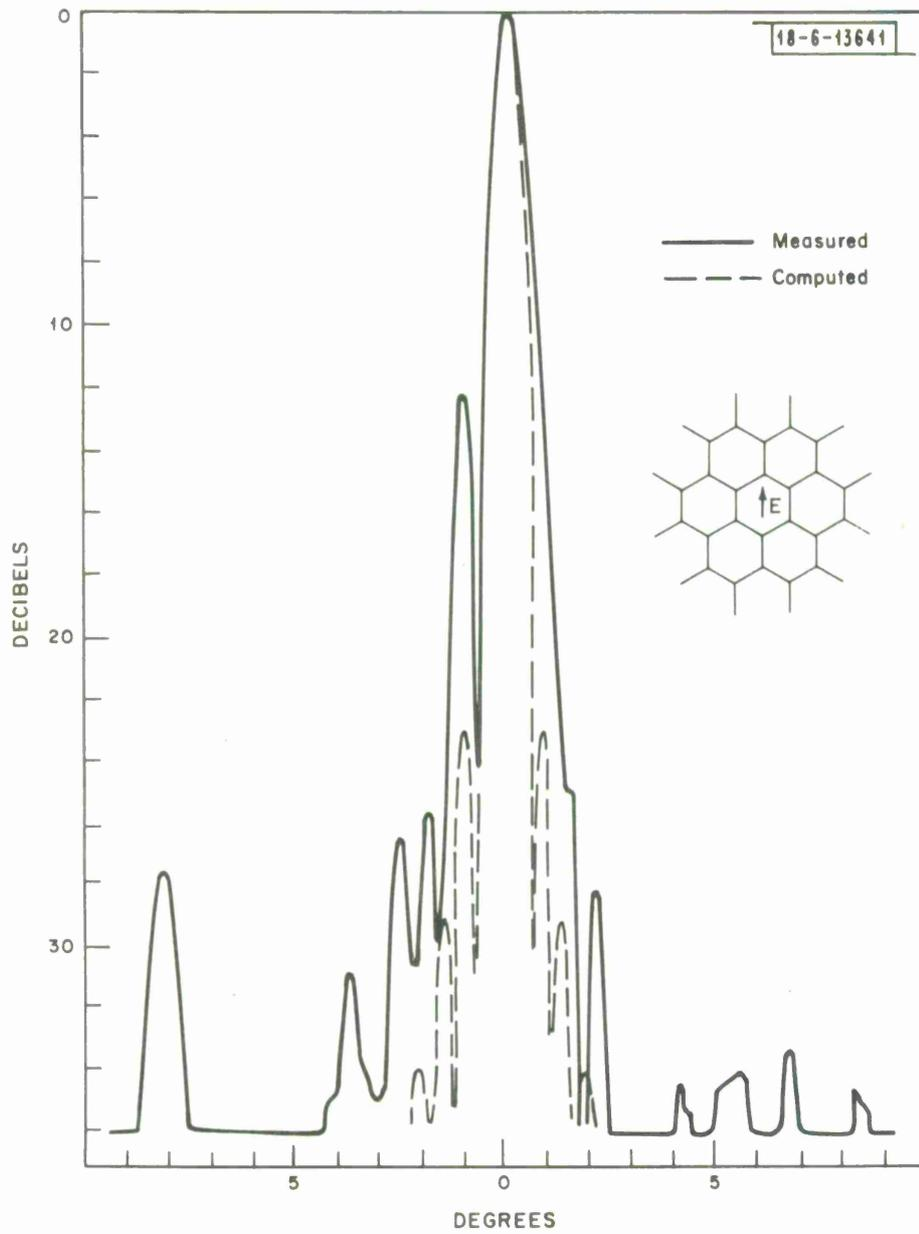
Fig. 7. E-plane pattern of EHF lens antenna.
