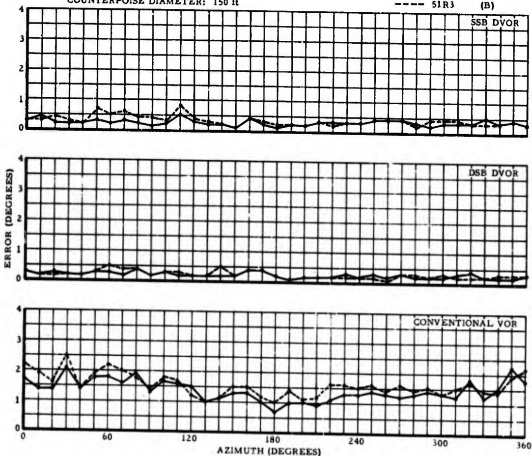
Figure 82. MAXIMUM SCALLOPING PER 10° SECTOR WITH TYPE MN-85FA (A) AND 51R3 (B) RECEIVERS, 150-FOOT COUNTERPOISE
