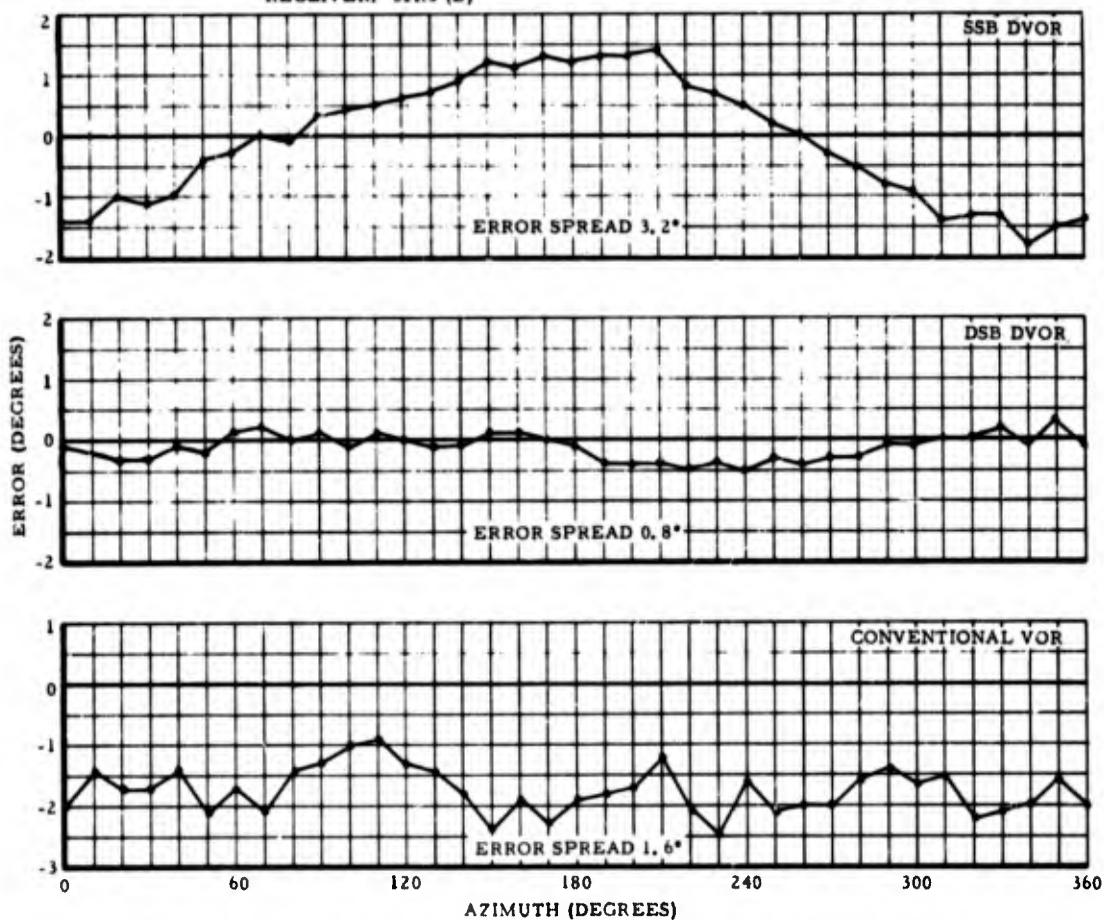
**Figure 70. INDICATED STATION ERROR WITH TYPE 51R3 (B) RECEIVER, 100-FOOT COUNTERPOISE**
