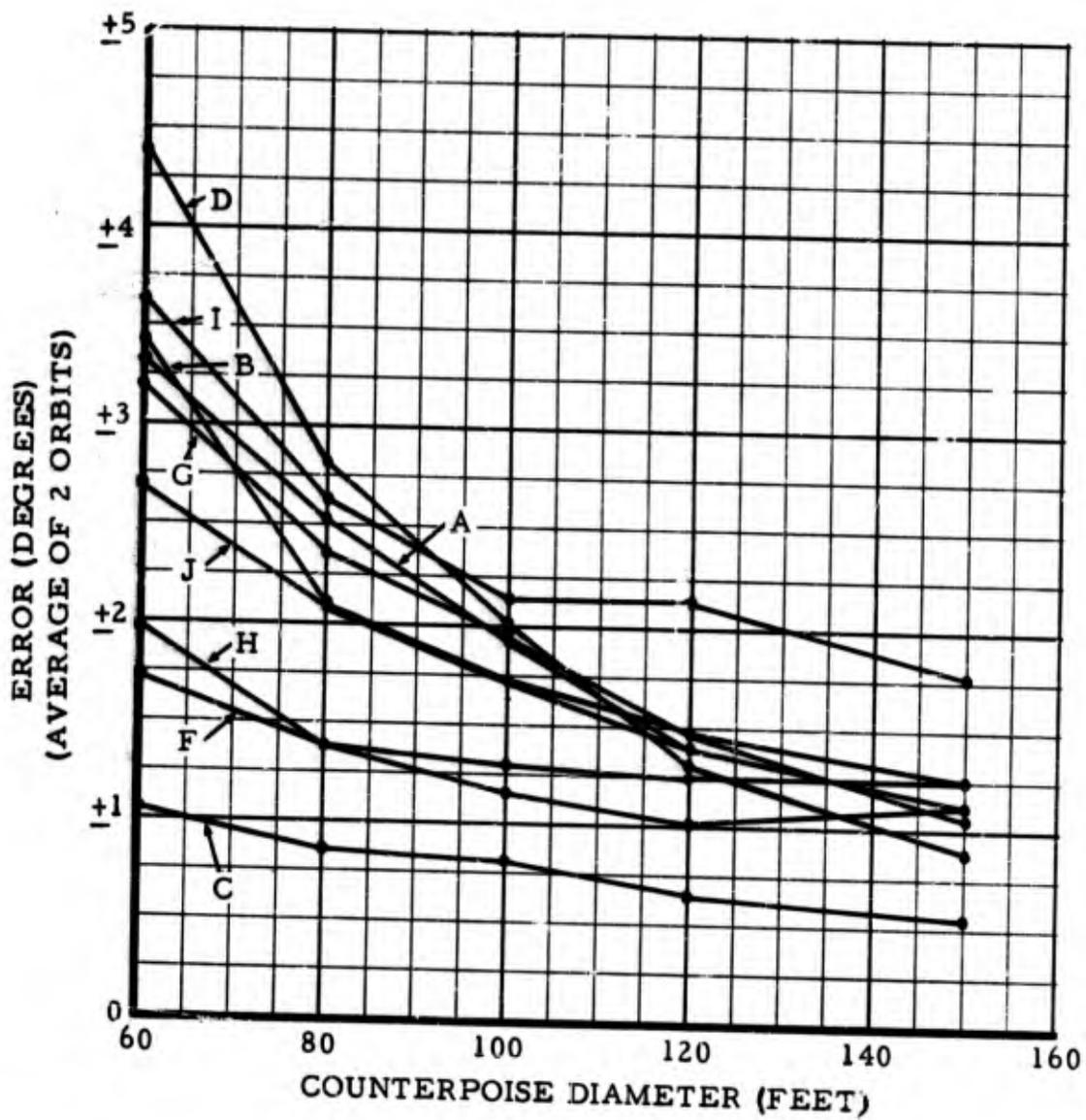
Figure 79. COMPOSITE INDICATED STATION ERROR WITH SSDVOR, VARIOUS COUNTERPOISE DIAMETERS
