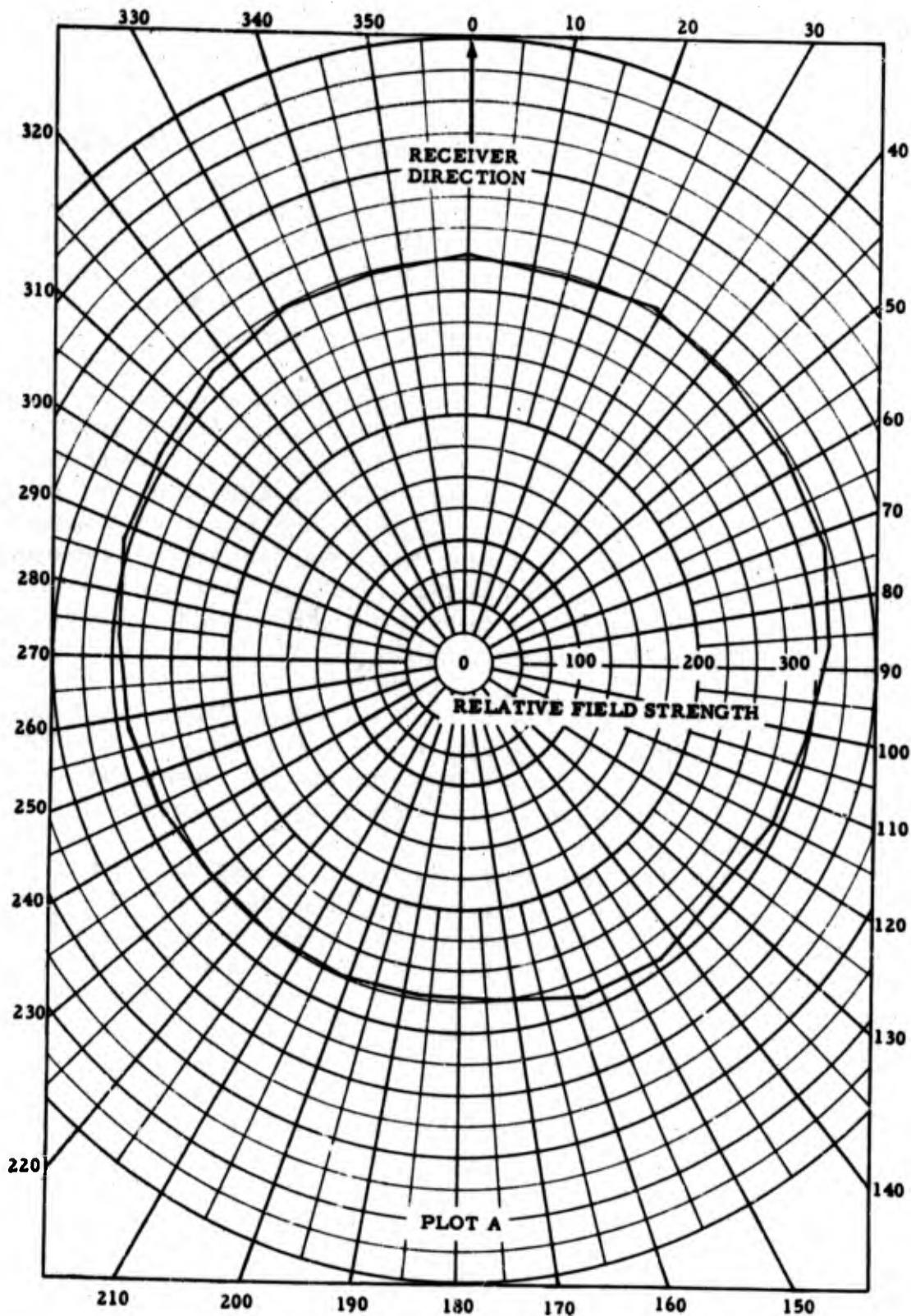
Figure 13. VARIATION IN FIELD STRENGTH OF ONE ANTENNA CAUSED BY ECCENTRICITY EFFECT OF 150-FOOT DIAMETER COUNTERPOISE
