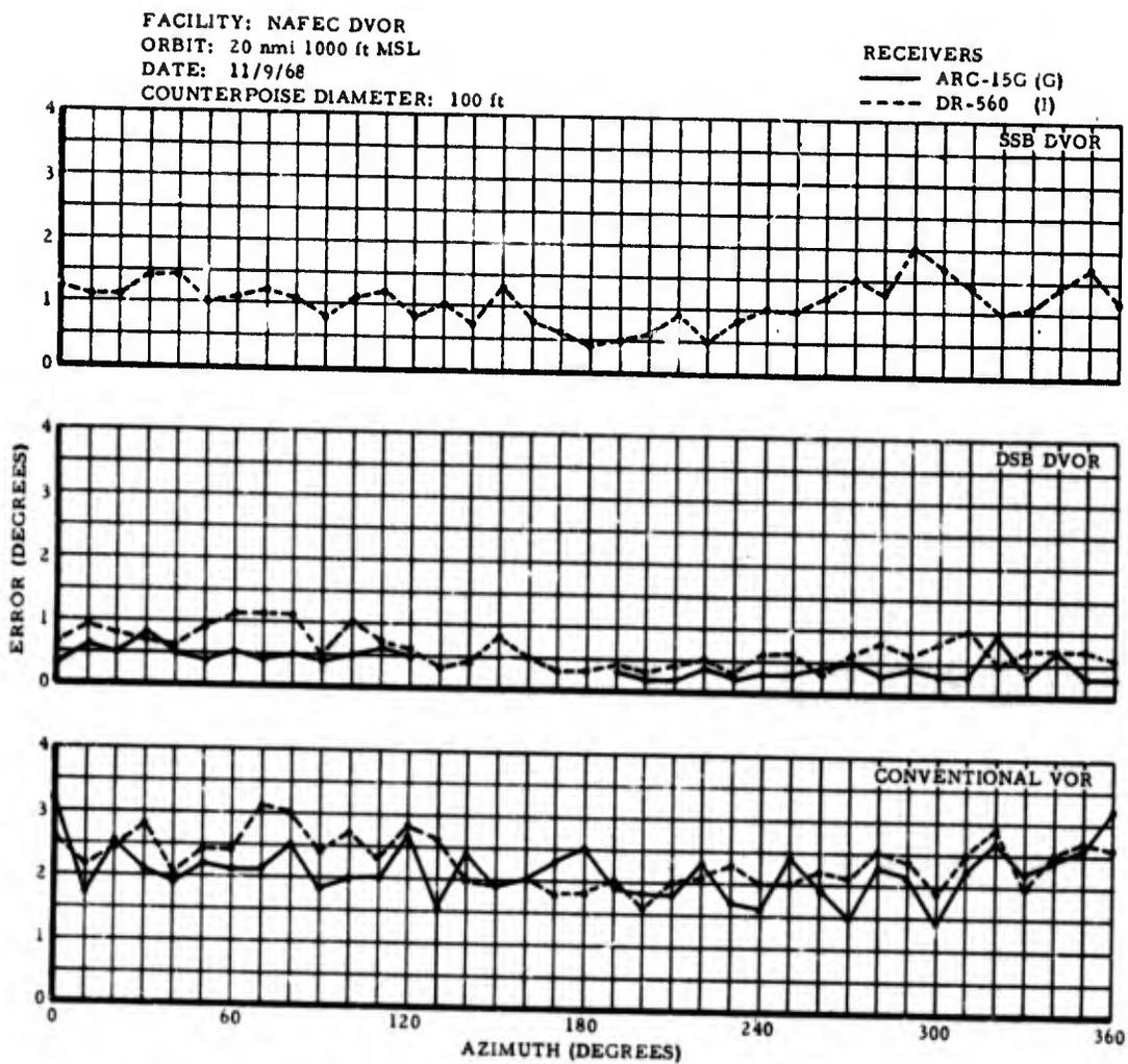
Figure 89. MAXIMUM SCALLOPING PER 10° SECTOR WITH TYPE ARC-15G (G) AND DR-560 (I) RECEIVERS, 100-FOOT COUNTERPOISE
