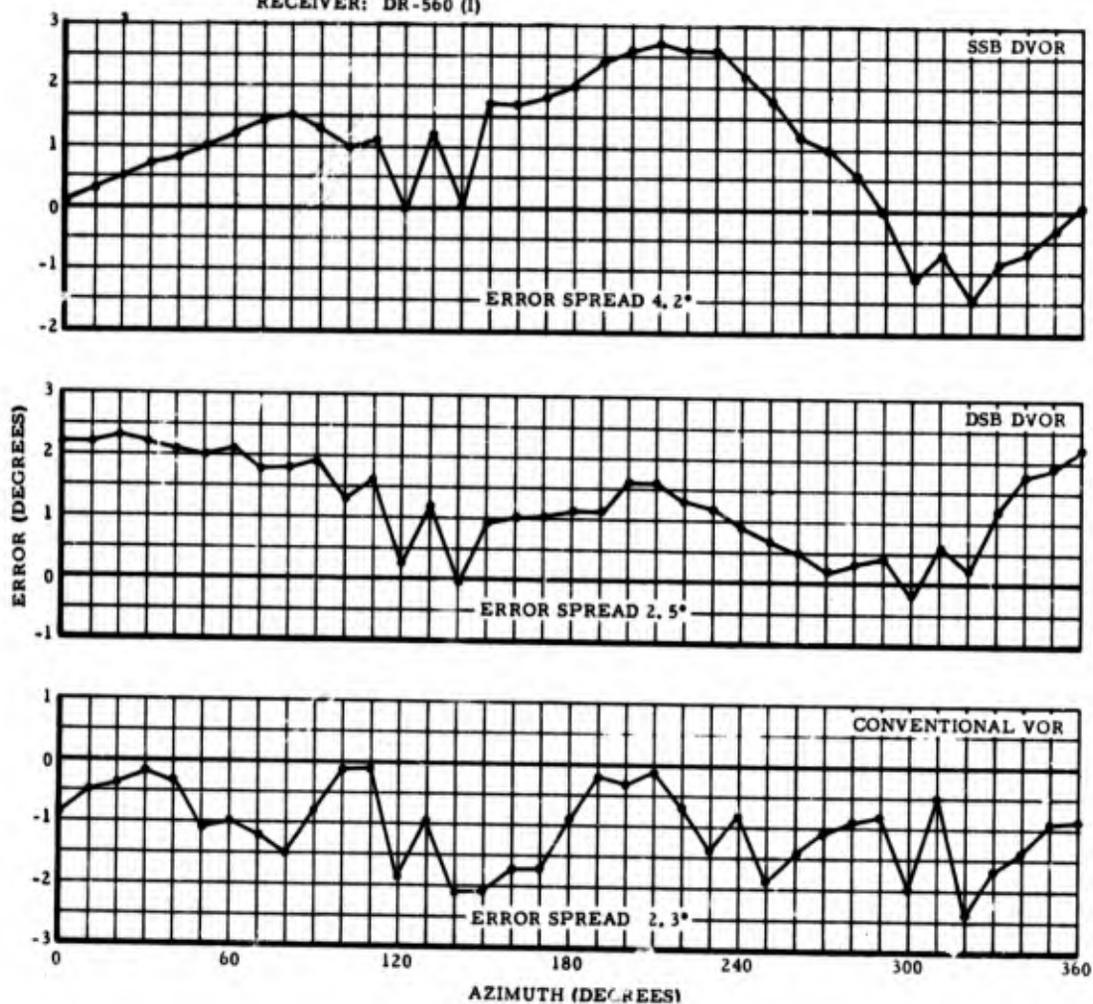
Figure 77. INDICATED STATION ERROR WITH TYPE DR-560 (I)
