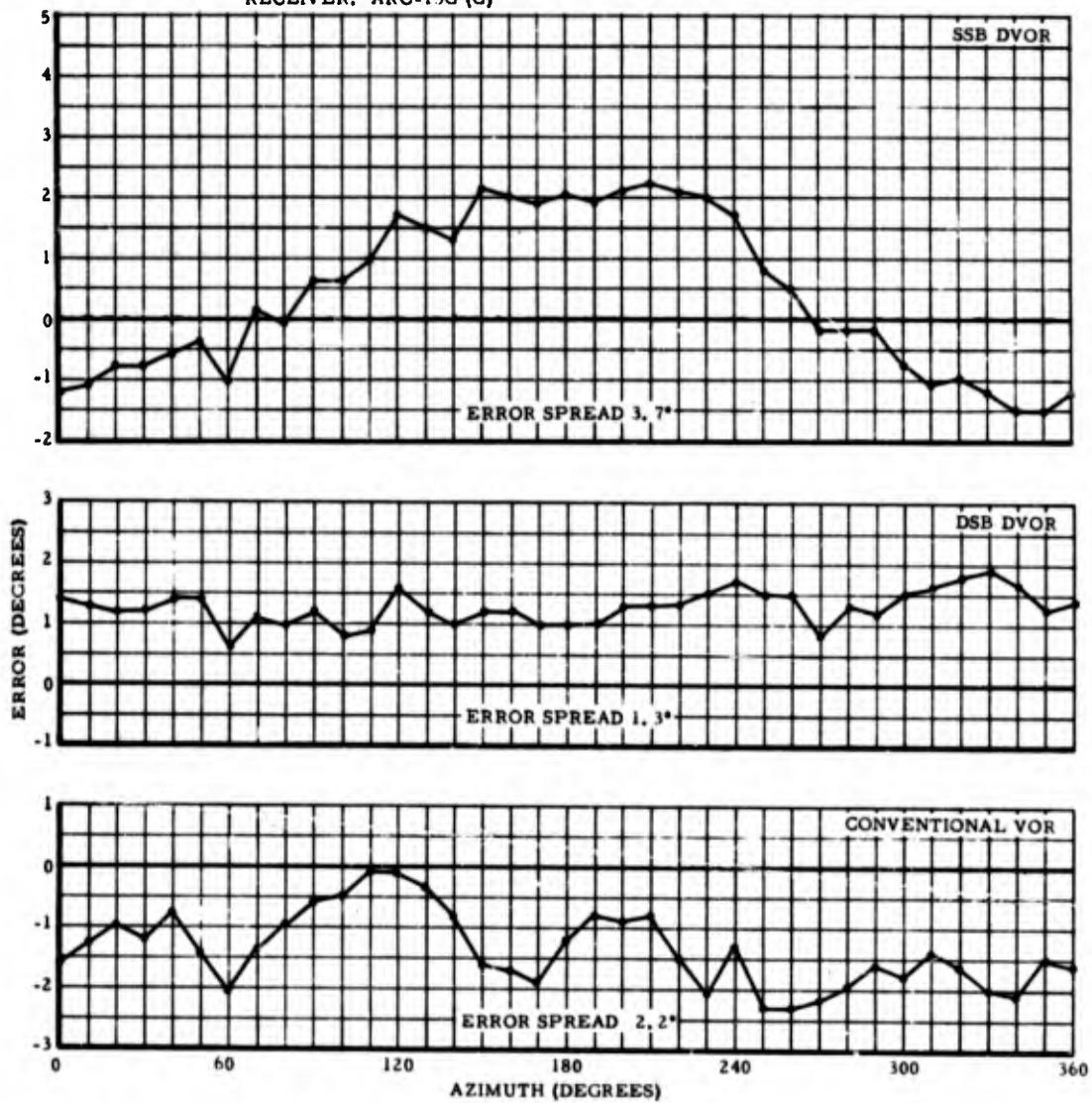
**Figure 75. INDICATED STATION ERROR WITH TYPE ARC-15G (G) RECEIVER, 100-FOOT COUNTERPOISE**
