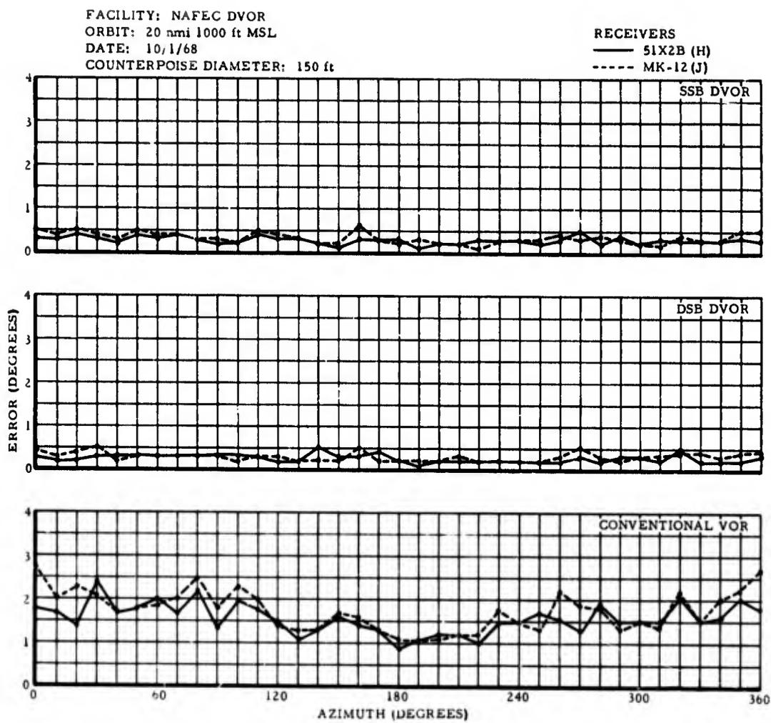
Figure 85. MAXIMUM SCALLOPING PER 10° SECTOR WITH TYPE 51X2B (H) AND MK-12 (J) RECEIVERS, 150-FOOT COUNTERPOISE
