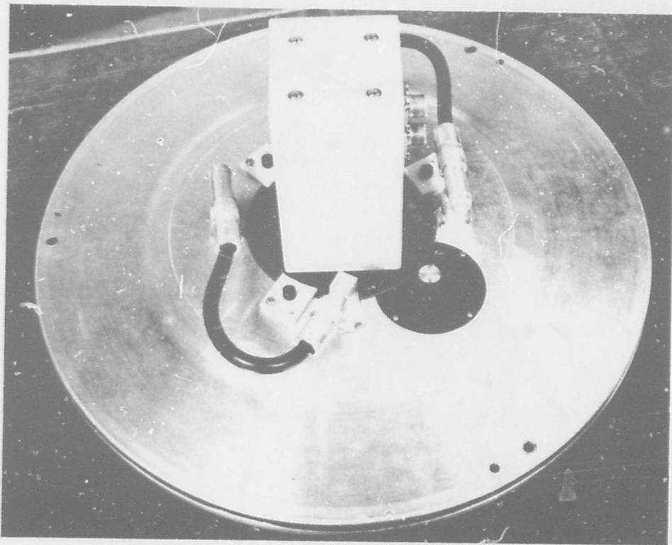
Figure 109. VOR DISTRIBUTOR, TOP COVER WITH GONIOMETER ATTACHED
