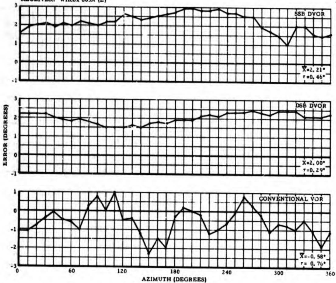
Figure 98. INDICATED STATION ERROR WITH TYPE 805A (E) RECEIVER, 150-FOOT COUNTERPOISE
