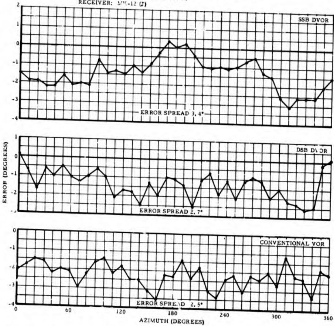
Figure 78. INDICATED STATION ERROR WITH TYPE MK-12 (J)
