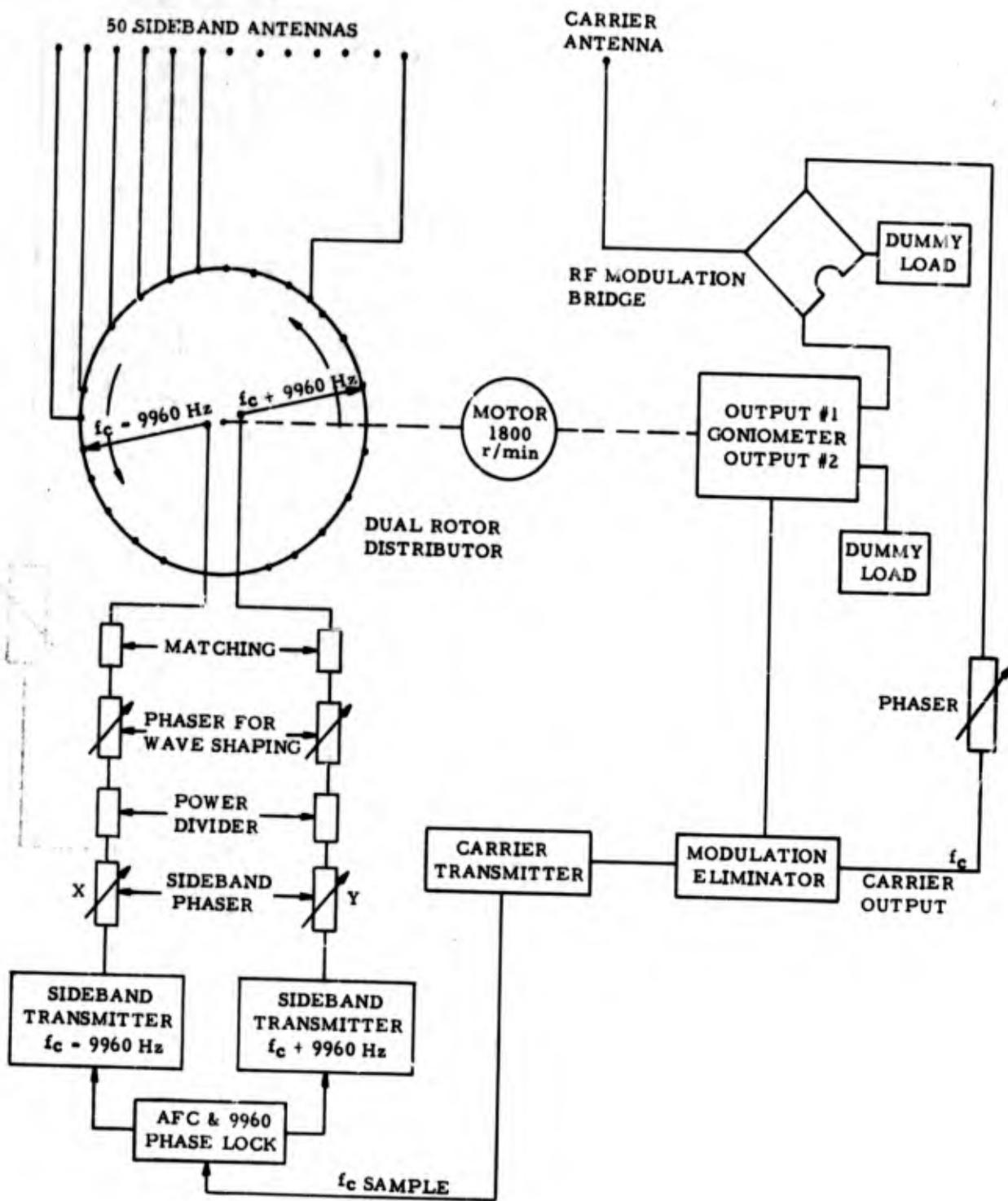
Figure 15. SIMPLIFIED BLOCK DIAGRAM OF DSDVOR SYSTEM
