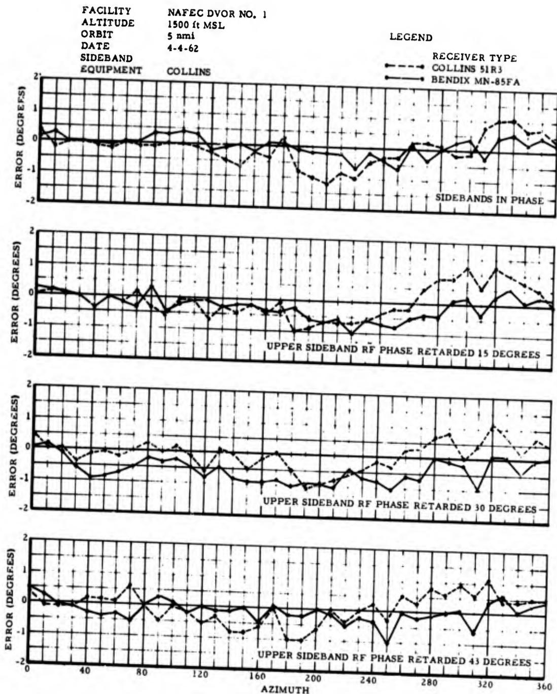
Figure 22. COMPARISON OF INDICATED STATION ERROR AS RF PHASE OF UPPER SIDE BAND IS RETARDED (COLLINS 51R3 AND BENDIX MN-85FA)
