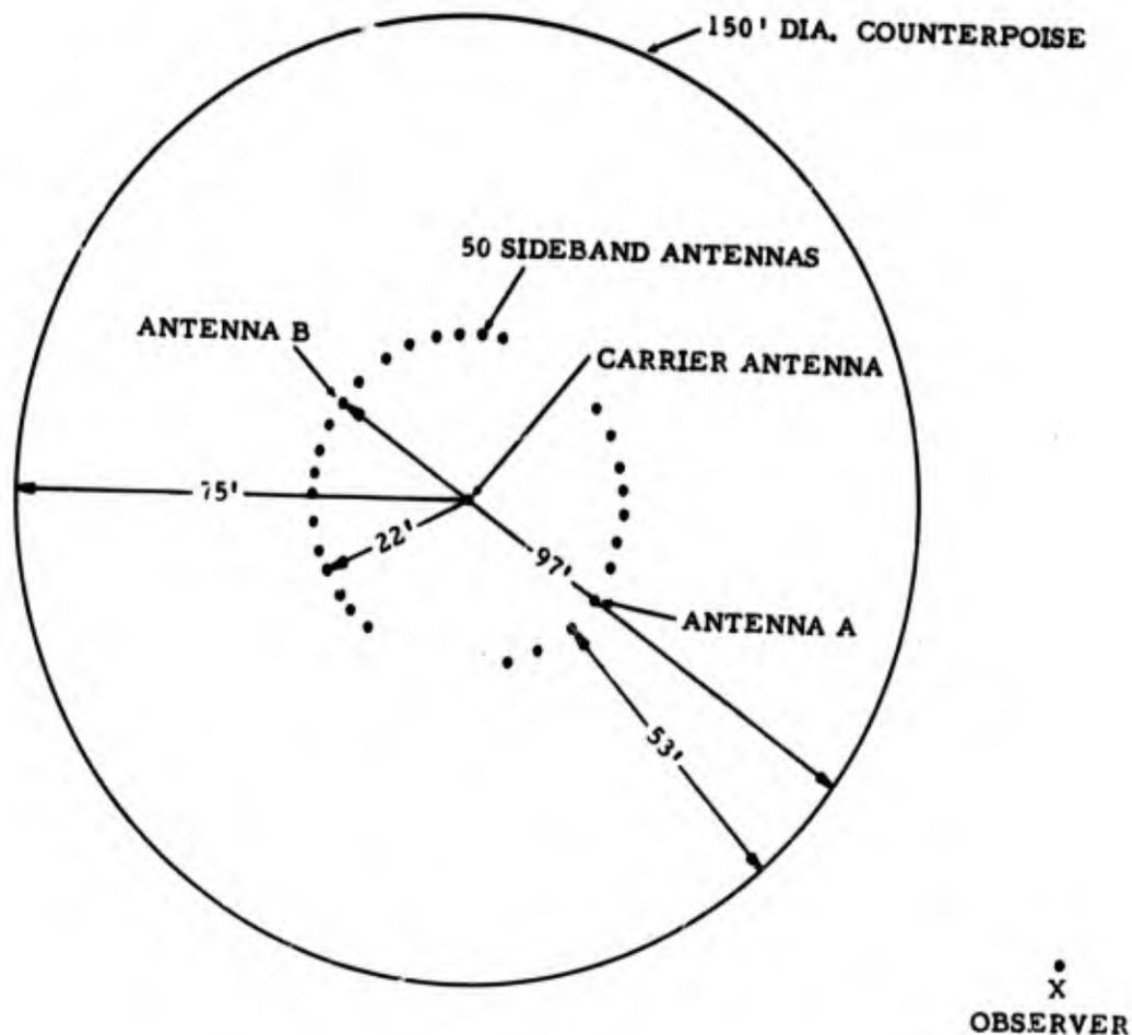
Figure 12. ILLUSTRATION OF COUNTERPOISE MODULATION DUE TO THE CHANGE IN THE EFFECTIVE COUNTERPOISE SIZE
