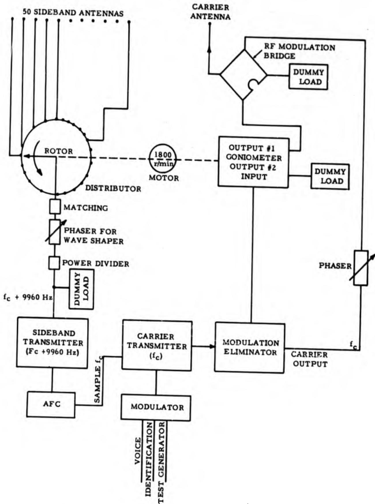
Figure 16. SIMPLIFIED BLOCK DIAGRAM OF SSDVOR SYSTEM
