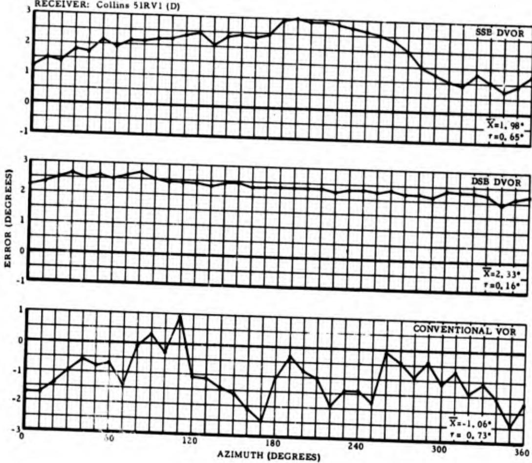
Figure 97. INDICATED STATION ERROR WITH TYPE 51RV1 (D) RECEIVER, 150-FOOT COUNTERPOISE
