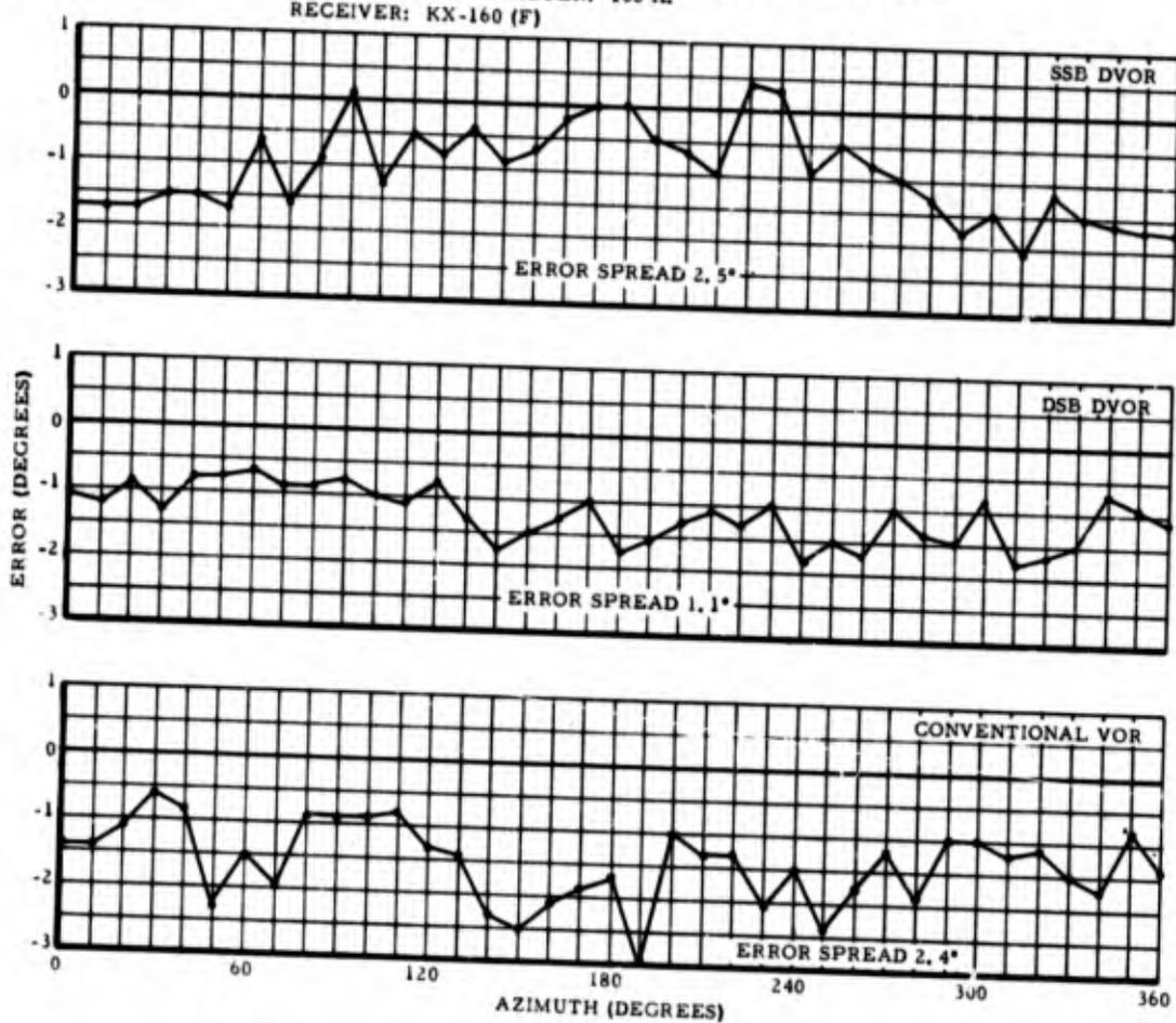
Figure 74. INDICATED STATION ERROR WITH TYPE KX-160 (F) RECEIVER, 100-FOOT COUNTERPOISE
