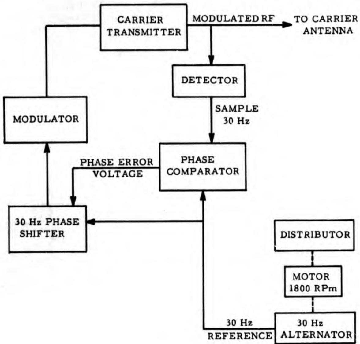
Figure 105. SIMPLIFIED BLOCK DIAGRAM OF AUTOMATIC PHASE CONTROL UNIT OF THE 30 HZ REFERENCE
