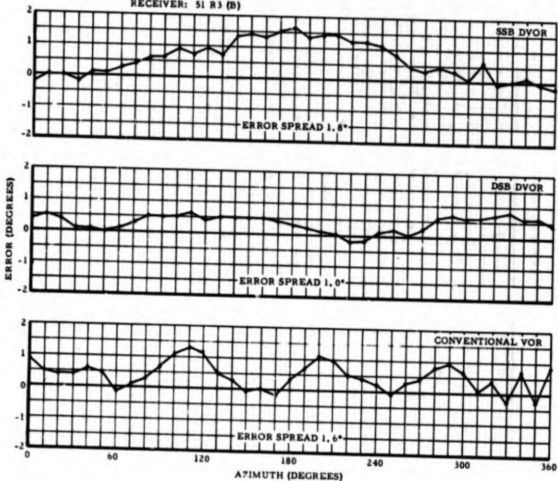
Figure 60. INDICATED STATION ERROR WITH TYPE 51R3 (B) RECEIVER,
