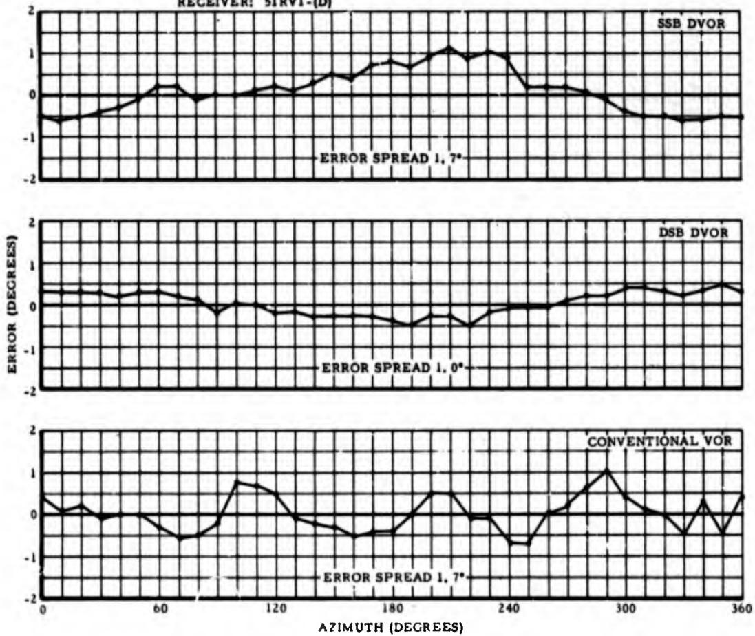
Figure 62. INDICATED STATION ERROR WITH TYPE 51RV1 (D)
