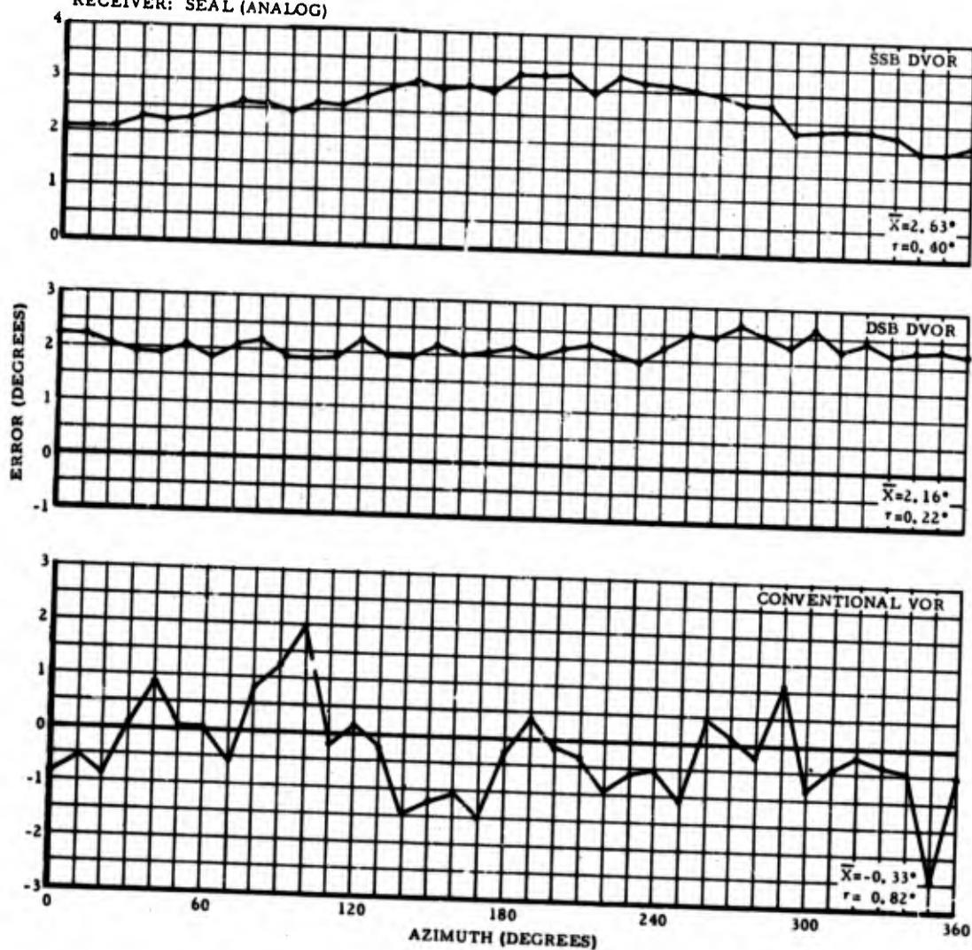
Figure 100. INDICATED STATION ERROR WITH ANALOG OUTPUT OF SEAL RECEIVER, 150-FOOT COUNTERPOISE
