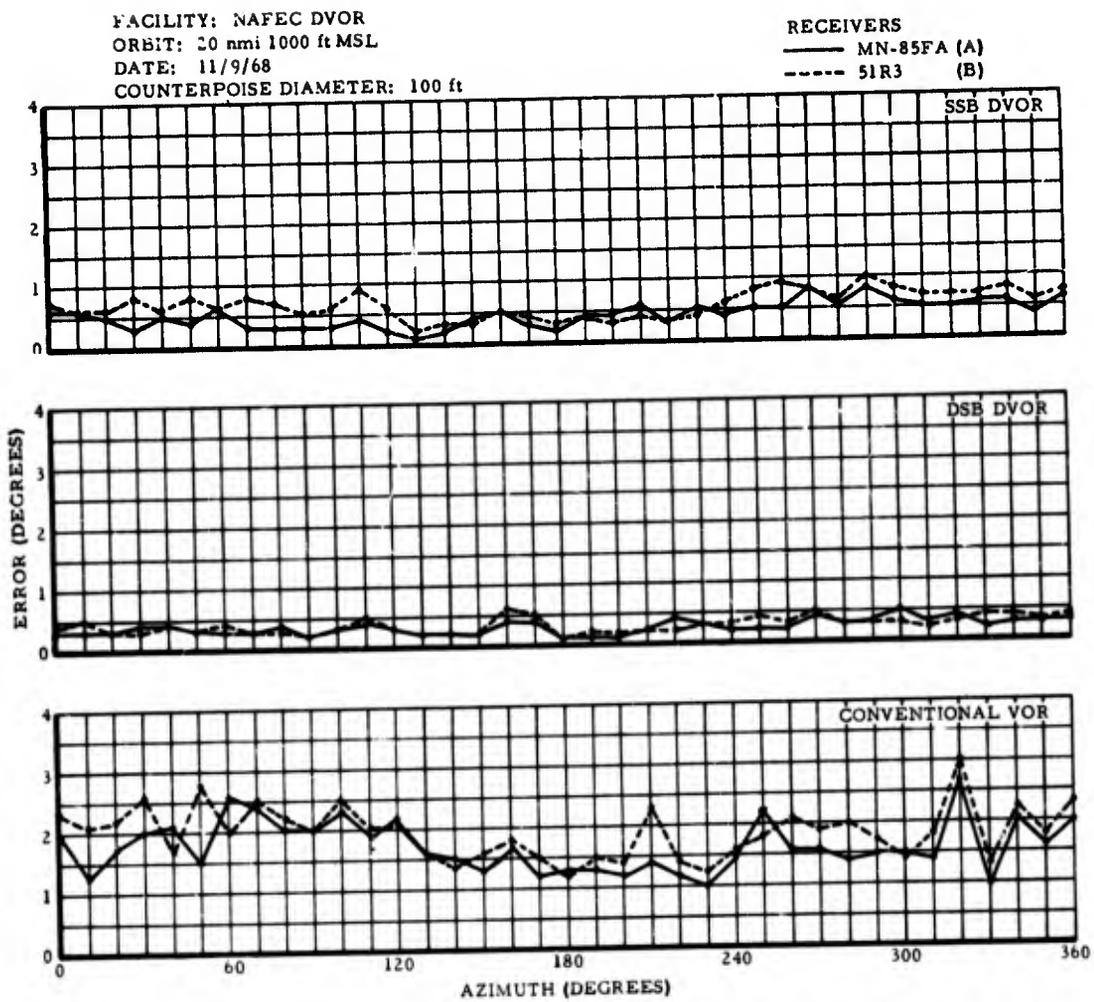
Figure 87. MAXIMUM SCALLOPING PER 10° SECTOR WITH TYPE MN-85FA (A) AND 51R3 (B) RECEIVERS, 100-FOOT COUNTERPOISE
