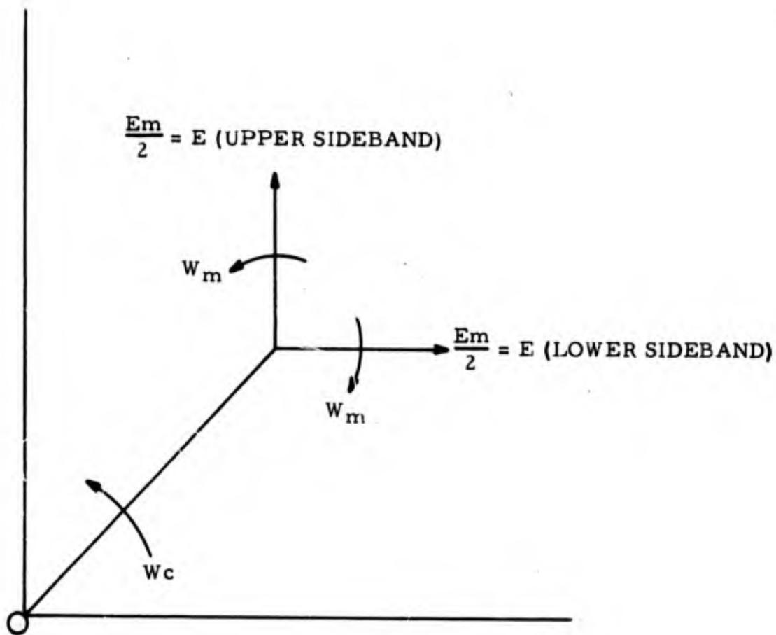
Figure 107. VECTOR DIAGRAM OF DSDVOR 9960 HZ AM MODULATION
