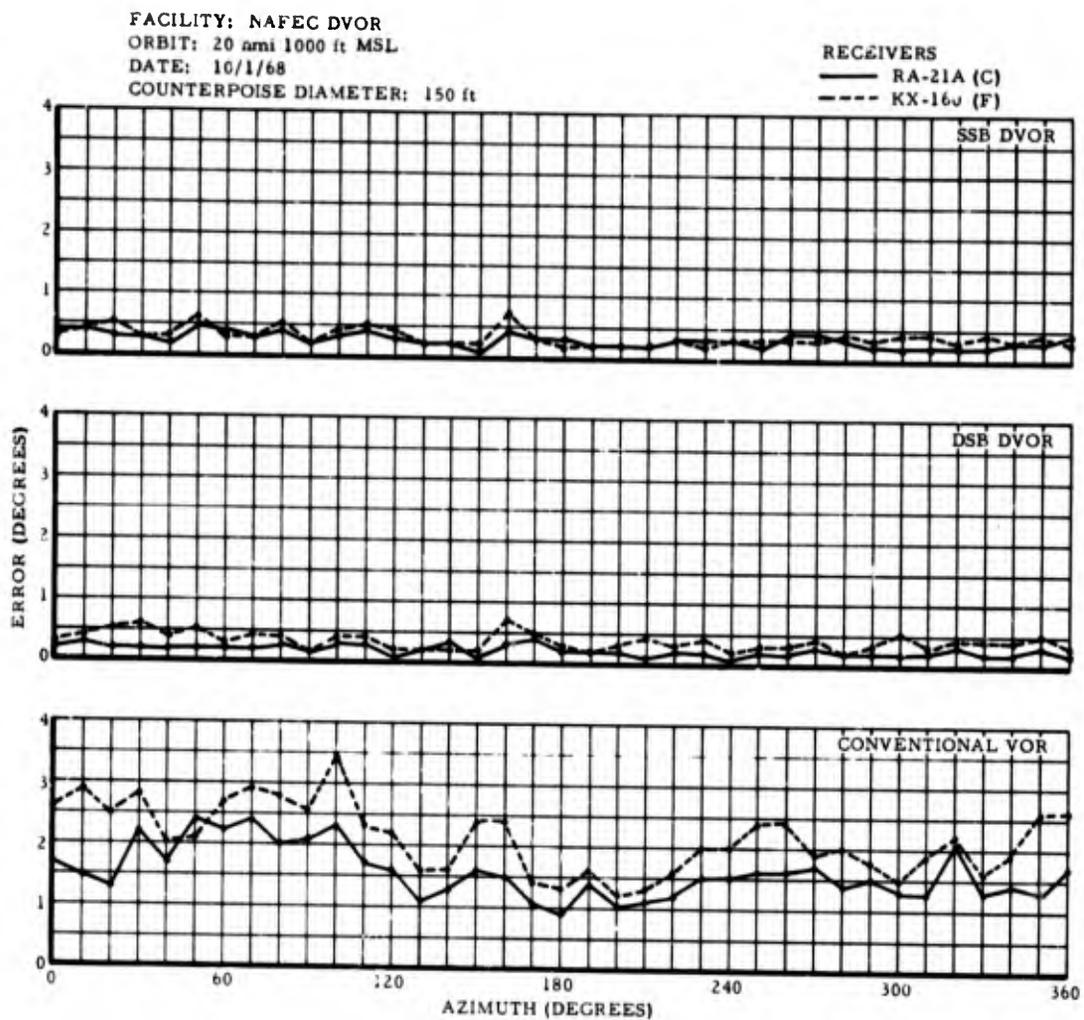
Figure 83. MAXIMUM SCALLOPING PER 10° SECTOR WITH TYPE RA-21A (C) AND KX-160 (F) RECEIVERS, 150-FOOT COUNTERPOISE
