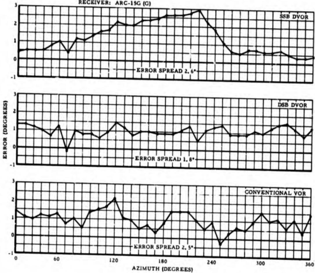
Figure 64. INDICATED STATION ERROR WITH TYPE ARC-15G (G)
