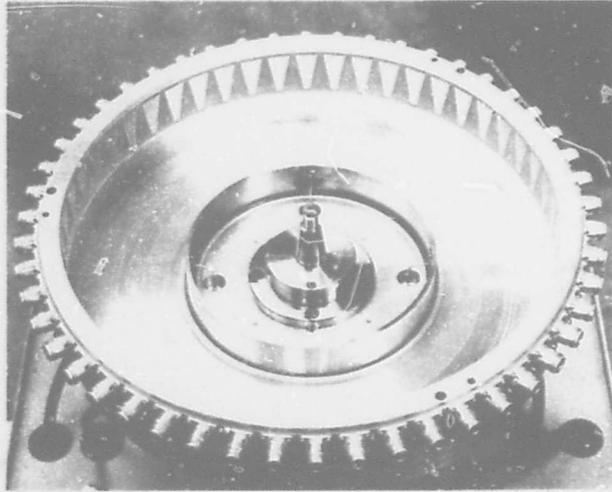
Figure 110. VOR DISTRIBUTOR, ROTOR REMOVED
