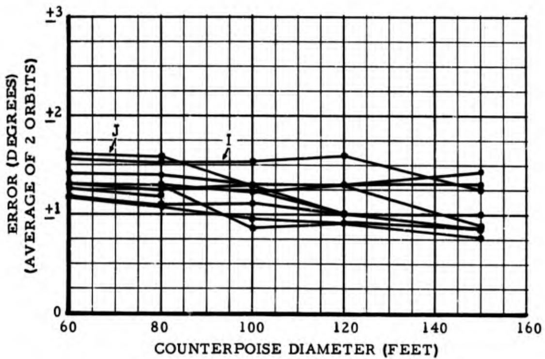
Figure 81. COMPOSITE INDICATED STATION ERROR WITH CONVENTIONAL VOR, VARIOUS COUNTERPOISE DIAMETERS
