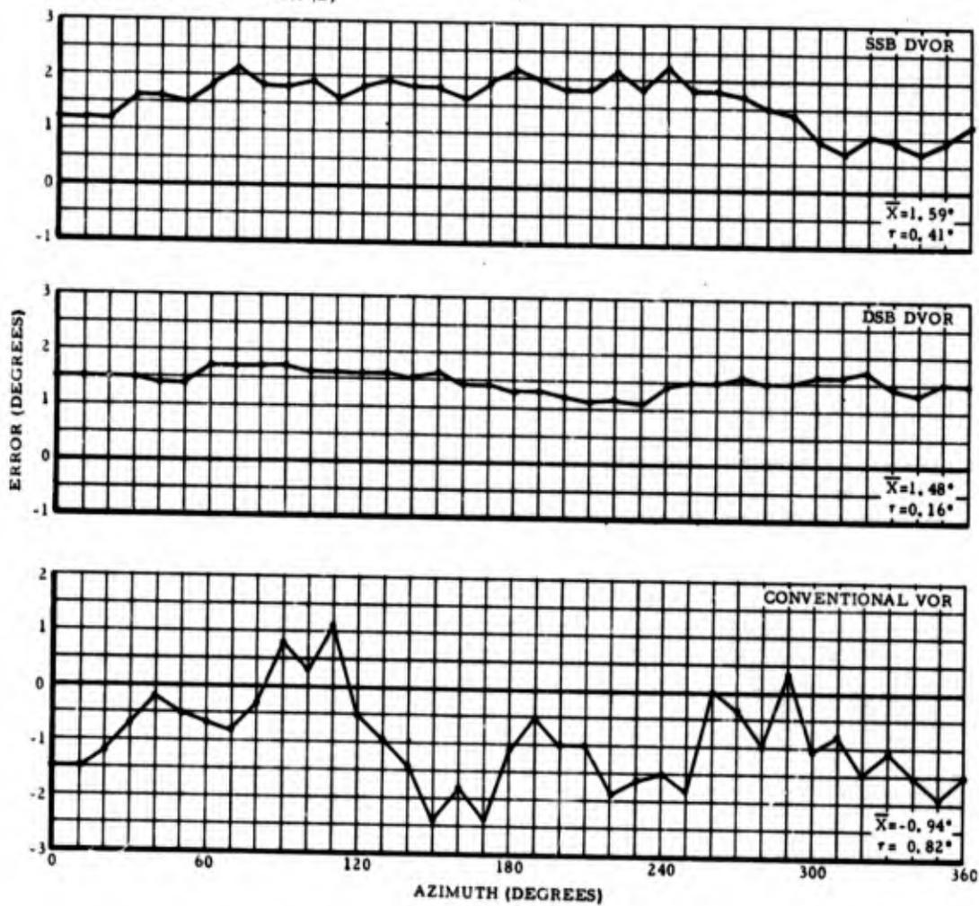
Figure 95. INDICATED STATION ERROR WITH TYPE 51R3 (B) RECEIVER, 150-FOOT COUNTERPOISE
