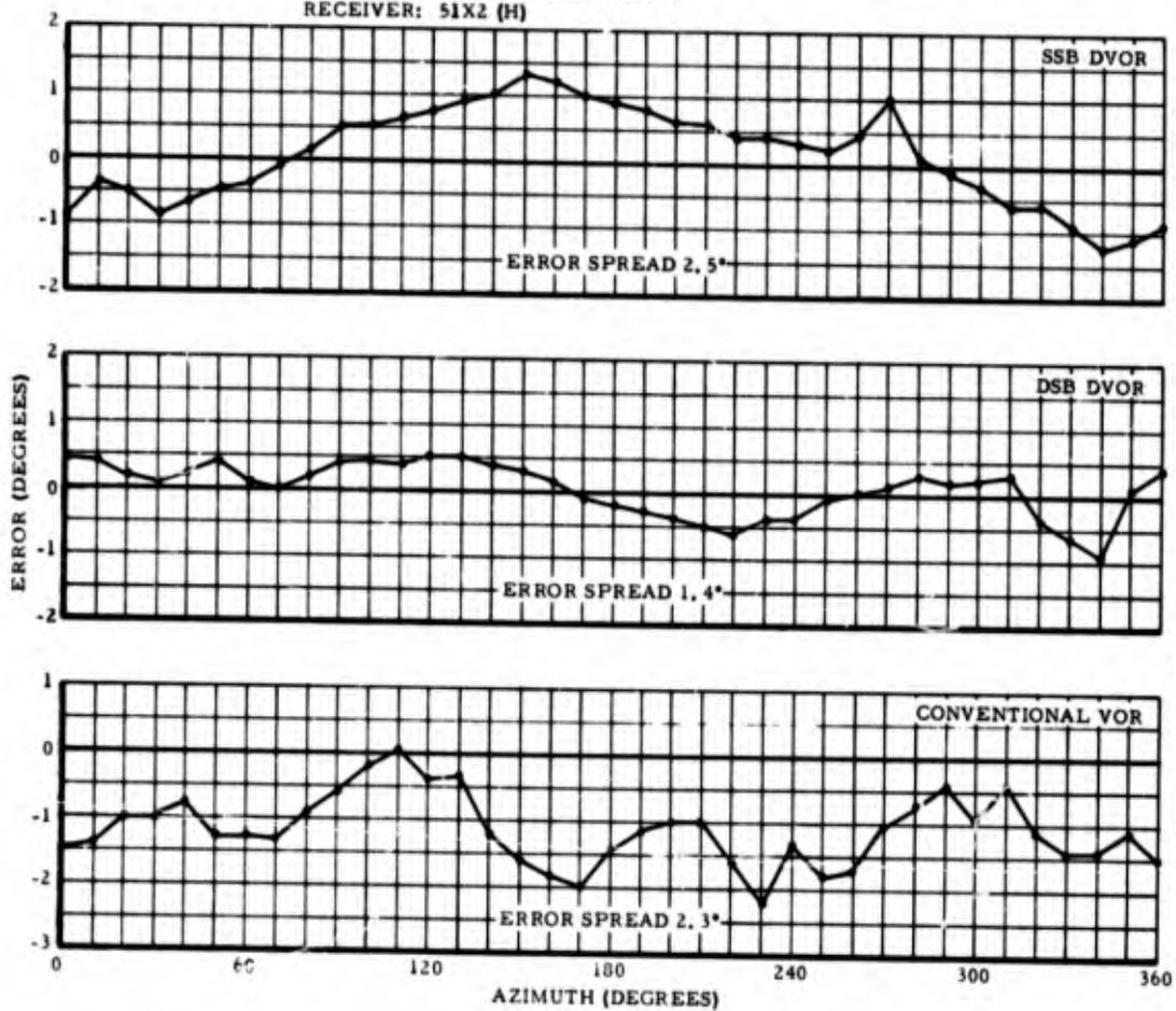
Figure 76. INDICATED STATION ERROR WITH TYPE 51X2 (H)
