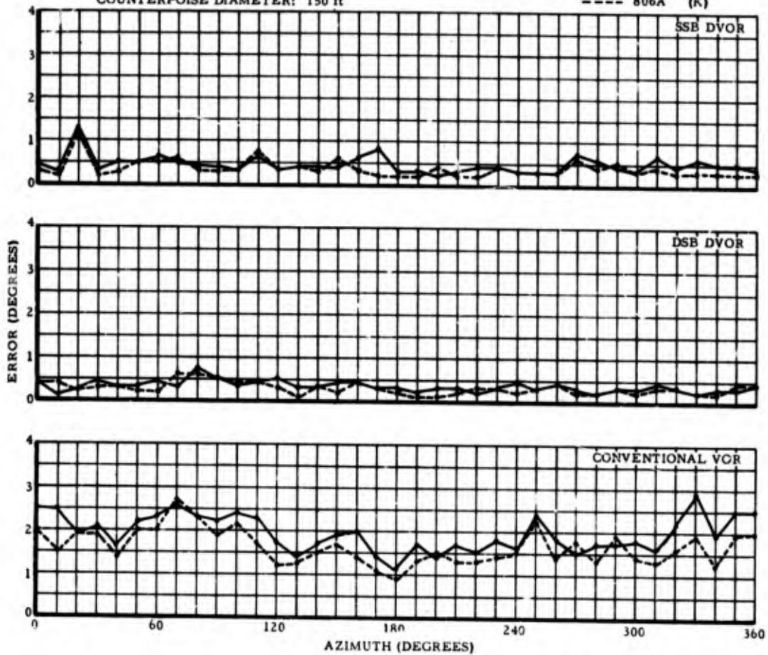
Figure 86. MAXIMUM SCALLOPING PER 10° SECTOR WITH TYPE 51RV1 (D) AND 806A (K) RECEIVERS, 150-FOOT COUNTERPOISE
