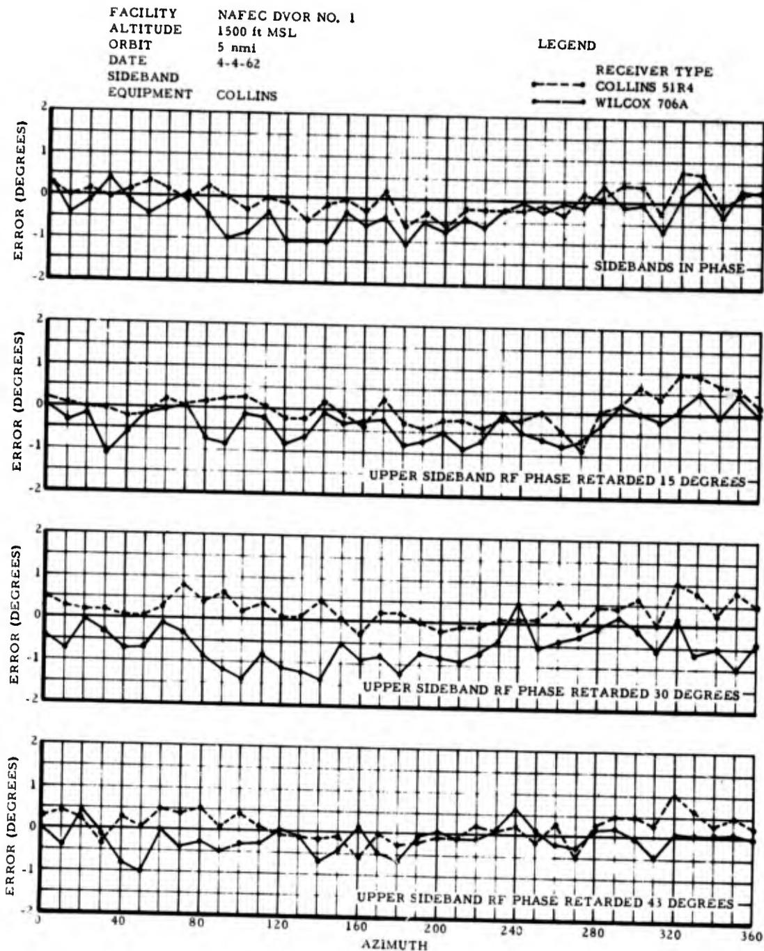
Figure 23. COMPARISON OF INDICATED STATION ERROR AS RF PHASE OF THE UPPER SIDE BAND IS RETARDED (COLLINS 51R4 AND WILCOX 706A)
