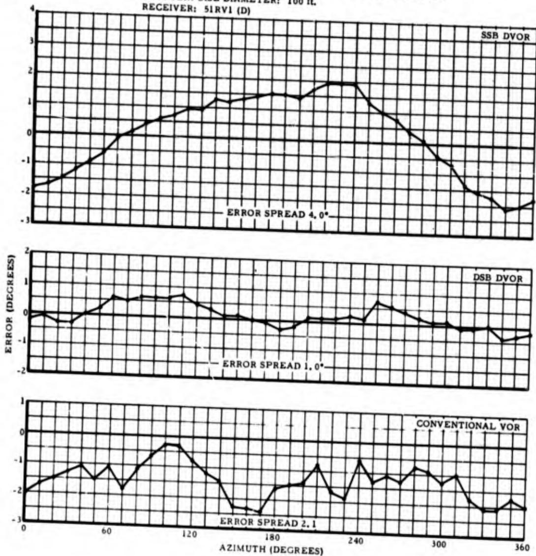
Figure 72. INDICATED STATION ERROR WITH TYPE 51RV1 (D) RECEIVER, 100-FOOT COUNTERPOISE
