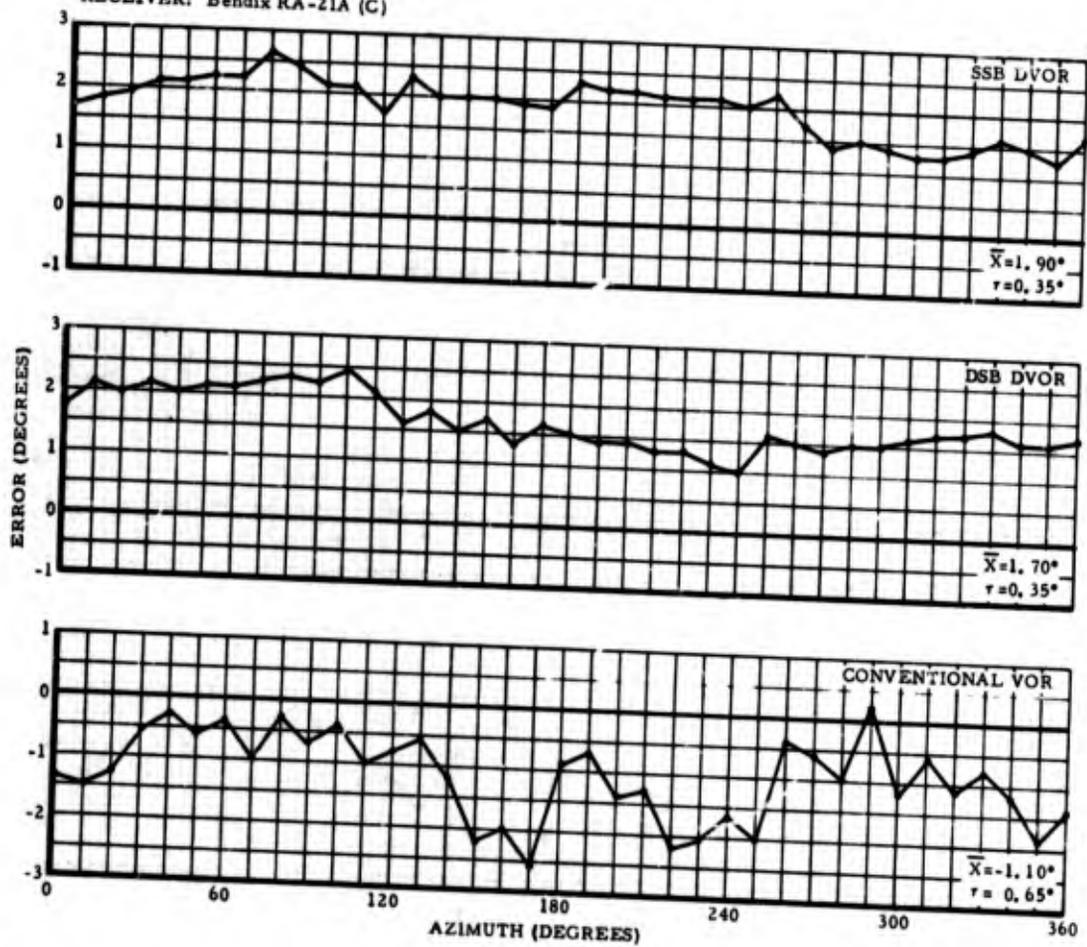
Figure 96. INDICATED STATION ERROR WITH TYPE RA-21A (C) RECEIVER, 150-FOOT COUNTERPOISE
