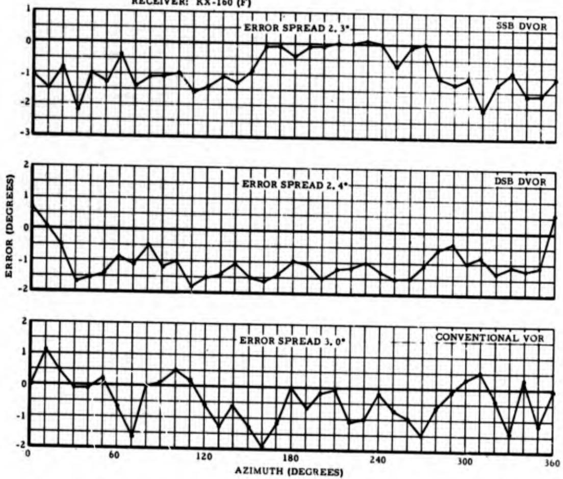
Figure 63. INDICATED STATION ERROR WITH TYPE KX-160 (F)
