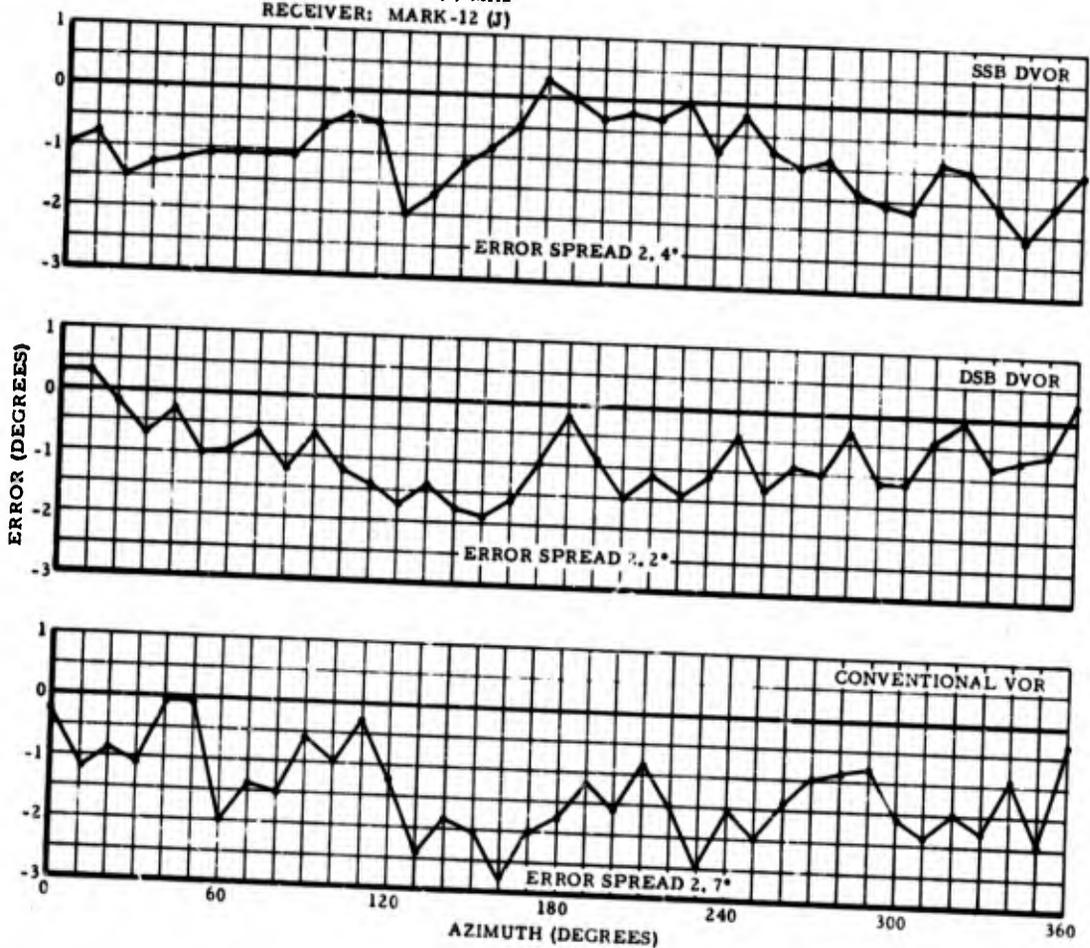
Figure 67. INDICATED STATION ERROR WITH TYPE MARK-12 (J)
