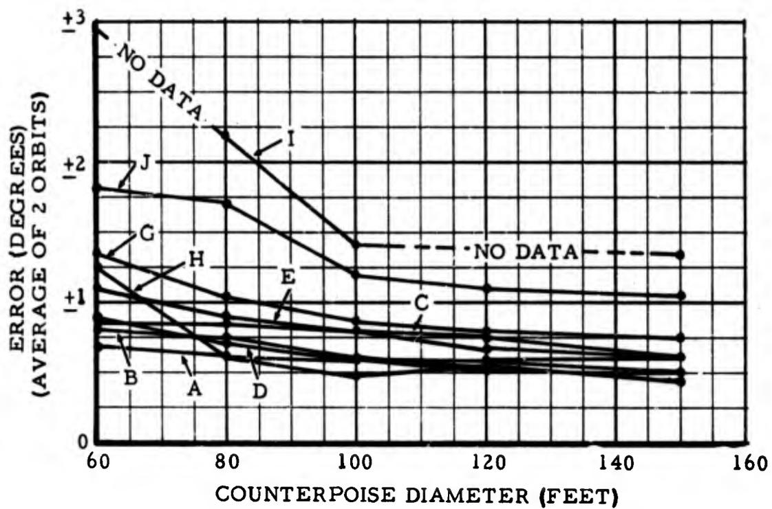
Figure 80. COMPOSITE INDICATED STATION ERROR WITH DSDVOR, VARIOUS COUNTERPOISE DIAMETERS
