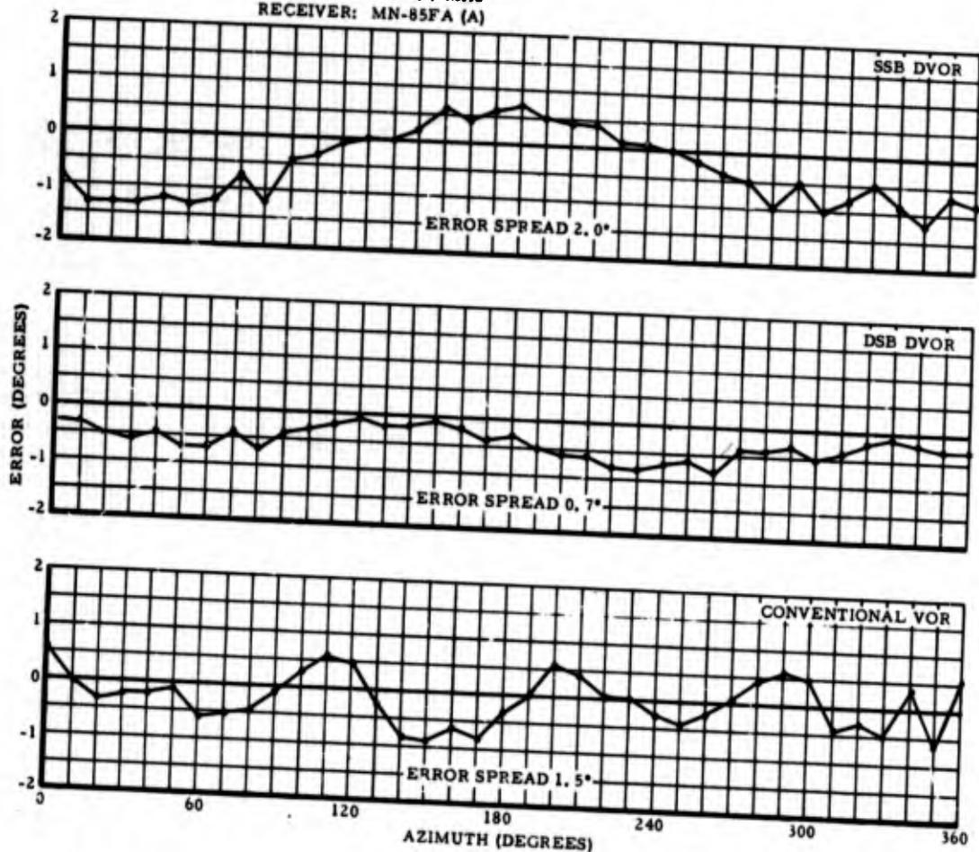
Figure 59. INDICATED STATION ERROR WITH TYPE MN-85FA (A)
