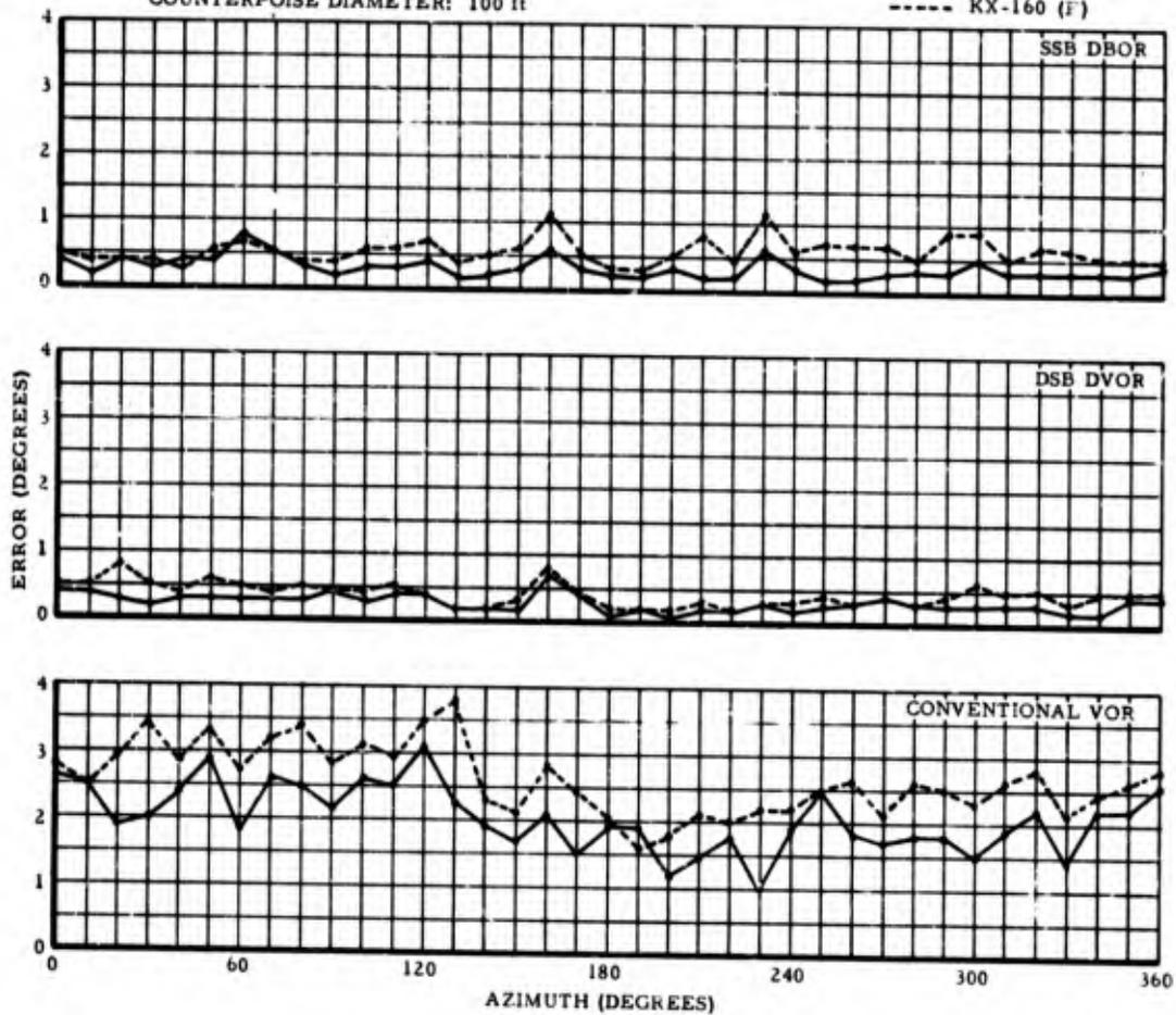
Figure 88. MAXIMUM SCALLOPING PER 10° SECTOR WITH TYPE RA-21A (C) AND KX-160 (F) RECEIVERS, 100-FOOT COUNTERPOISE
