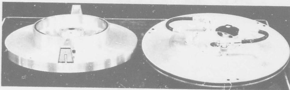
Figure 112. VOR DISTRIBUTOR, ROTOR ASSEMBLY AND TOP COVER
