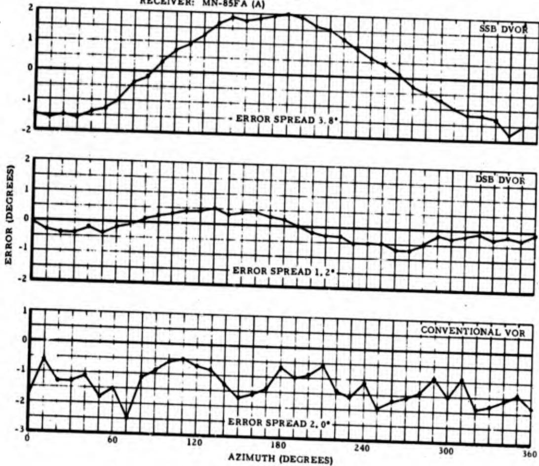
Figure 69. INDICATED STATION ERROR WITH TYPE MN-85FA (A)
