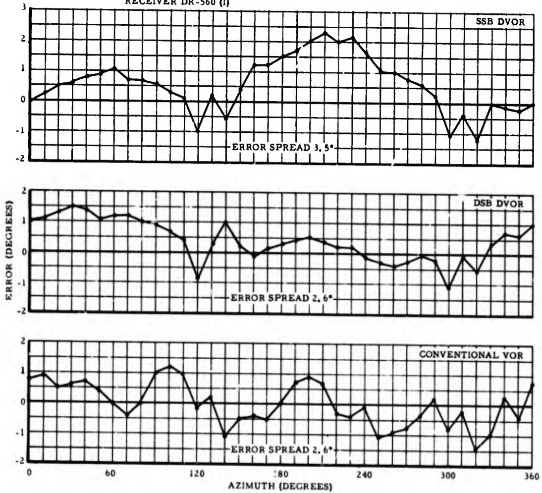
Figure 66. INDICATED STATION ERROR WITH TYPE DR-560 (I)
