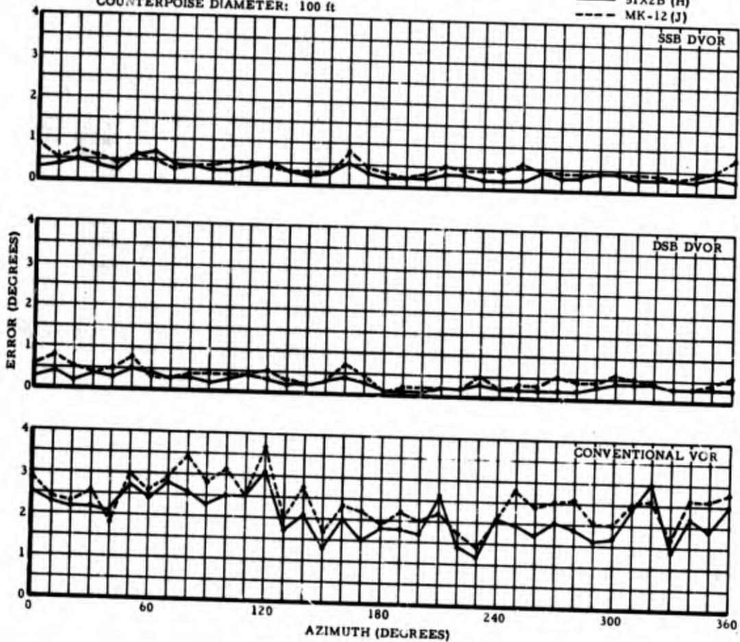
Figure 90. MAXIMUM SCALLOPING PER 10° SECTOR WITH TYPE 51X2B (H) AND MK-12 (J) RECEIVERS, 100-FOOT COUNTERPOISE
