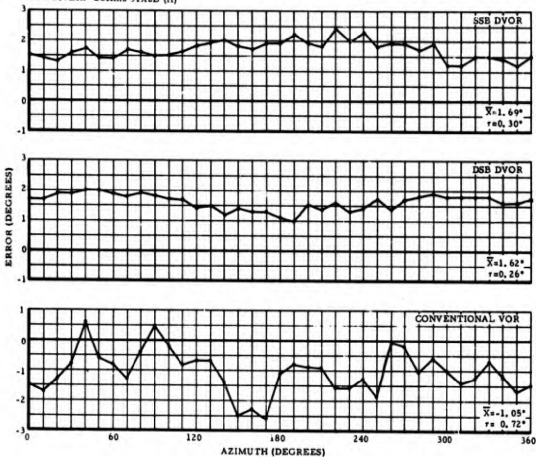
Figure 99. INDICATED STATION ERROR WITH TYPE 51X2B (H) RECEIVER, 150-FOOT COUNTERPOISE
