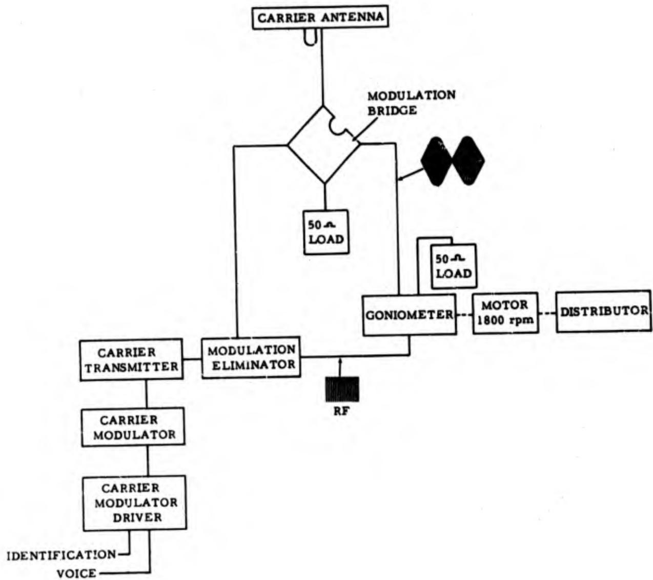
Figure 3. BLOCK DIAGRAM OF THE DVOR 30 HZ AM MODULATION SYSTEM
