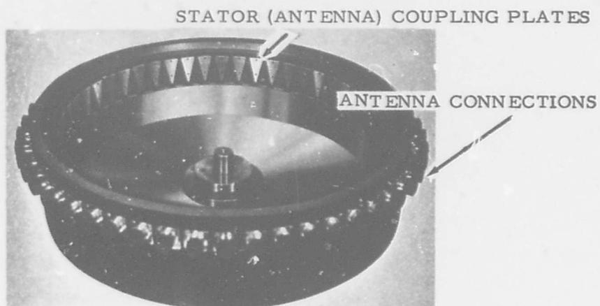
Figure 8. DISTRIBUTOR HEAD WITH COVER AND ROTOR REMOVED
