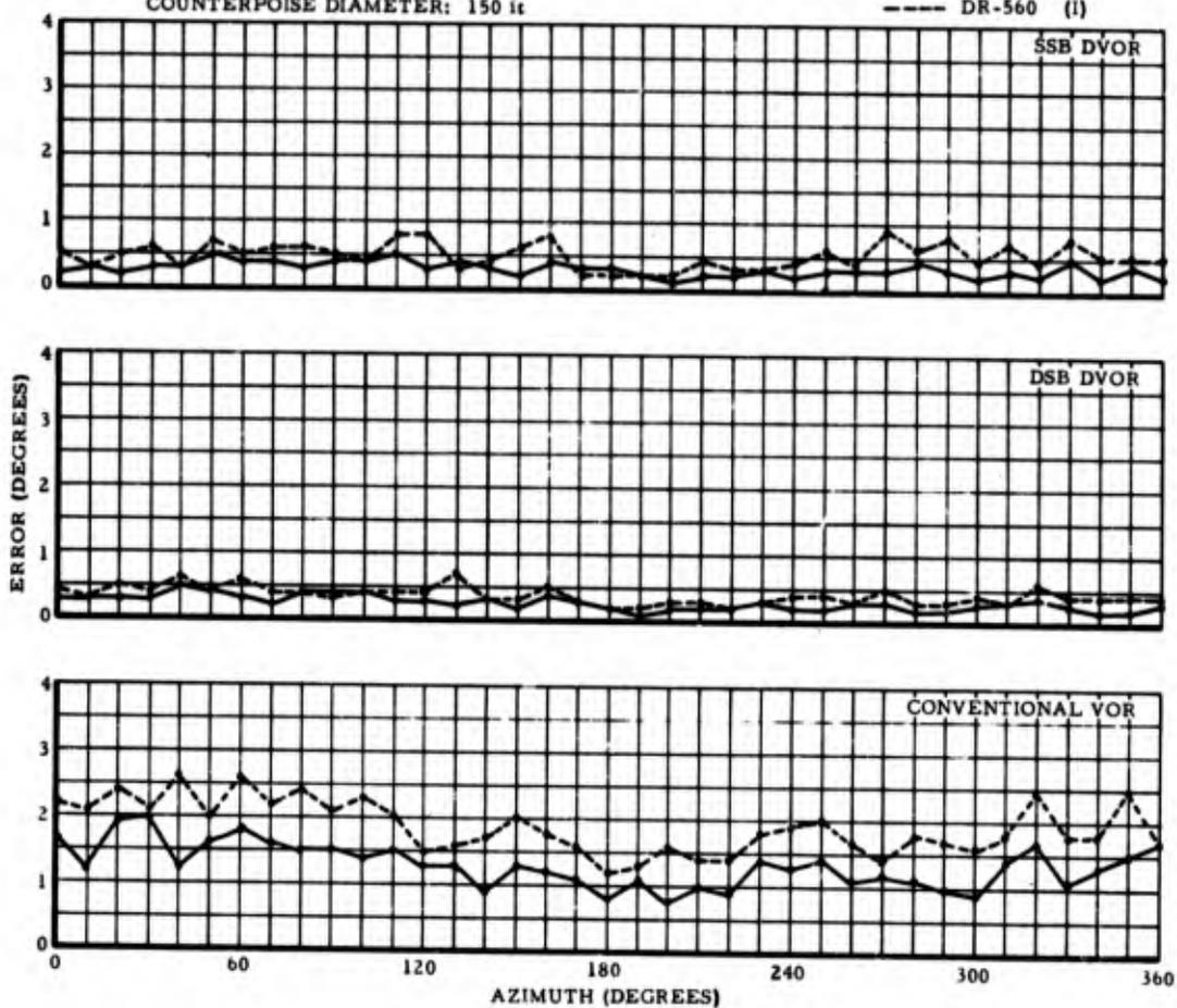
Figure 84. MAXIMUM SCALLOPING PER 10° SECTOR WITH TYPE ARC-15G (G) AND DR-560 (I) RECEIVERS, 150-FOOT COUNTERPOISE
