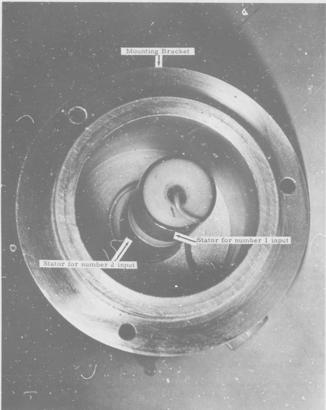
Figure 113. STATOR OF THE INPUT COUPLING CAPACITOR AND MOUNTING BRACKET OF THE JANSKY AND BAILEY DOUBLE SIDEBAND DISTRIBUTOR
