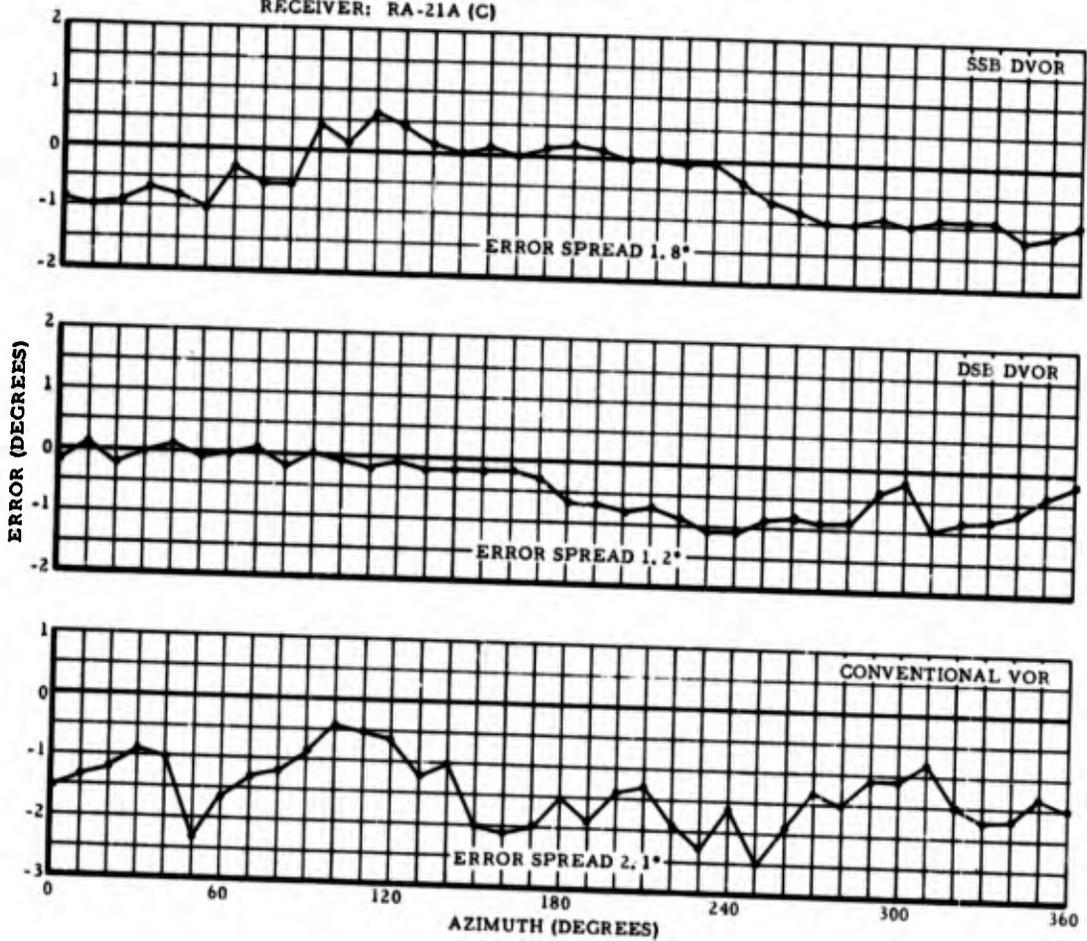
Figure 71. INDICATED STATION ERROR WITH TYPE RA-21A (C) RECEIVER, 100-FOOT COUNTERPOISE
