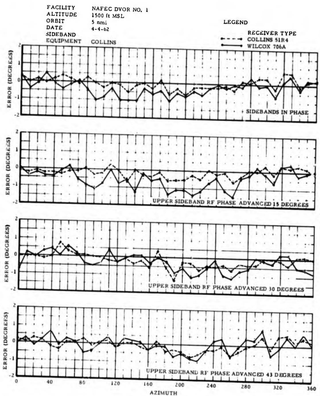
Figure 21. COMPARISON OF INDICATED STATION ERROR AS RF PHASE OF UPPER SIDEBAND IS ADVANCED (COLLINS 51R4 AND WILCOX 706A)
