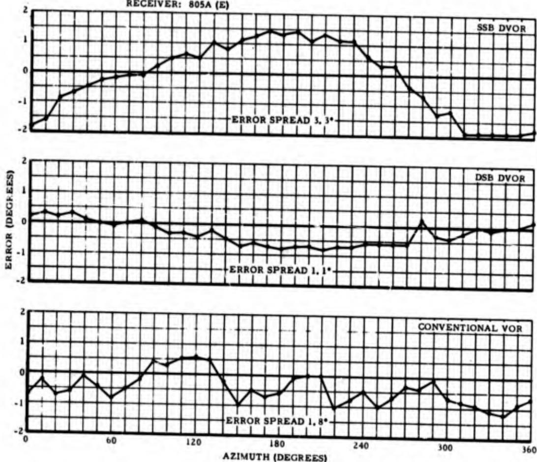
Figure 73. INDICATED STATION ERROR WITH TYPE 805A (E) RECEIVER, 100-FOOT COUNTERPOISE
