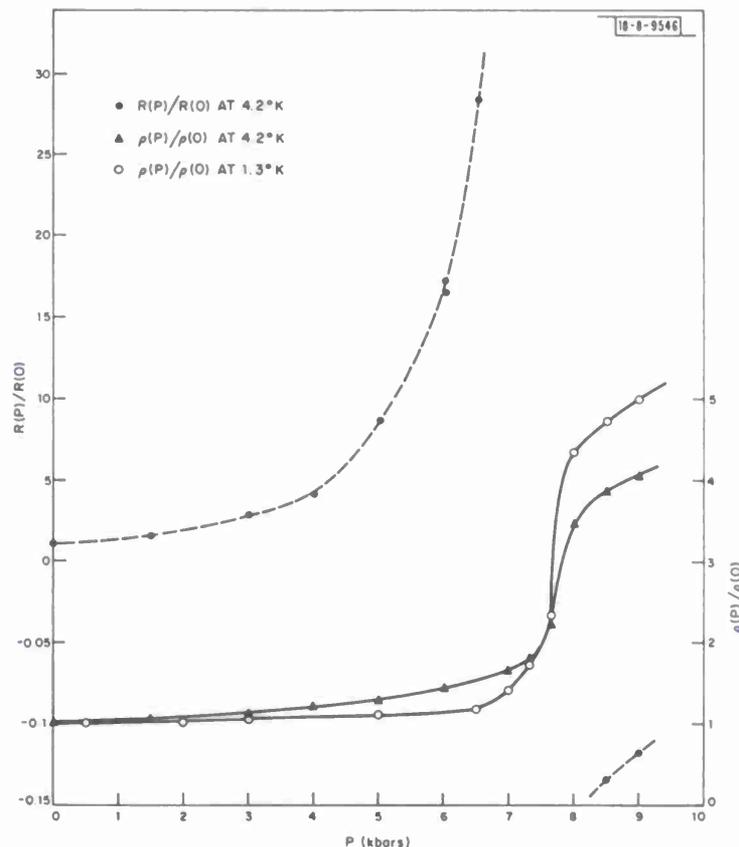
Fig. III-1. Relative variation of zero field Hall coefficient and resistivity of  $\text{Hg}_{0.86}\text{Cd}_{0.14}\text{Te}$  as a function of pressure. Scale for  $R(P)/R(0)$ , which is on the left, changes for negative values. Hall coefficient rises sharply to 8 kbars and changes sign between 8 and 8.5 kbars. Relative resistivity  $\rho(P)/\rho(0)$  increases sharply between 7 and 8 kbars.
