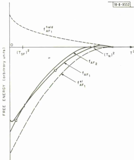
Fig. III-9. Schematic representations of the free energies of the magnetic configurations versus temperature squared. The stable configuration is indicated by the arrows. Detailed description of the symbols used is given in the text.
