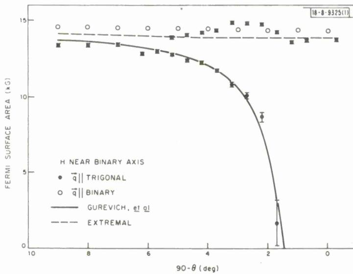
Fig. III-5. Fermi surface areas (in kilogauss). Solid dots are for  $\vec{q}$  along trigonal axis,  $\vec{H}$  in binary-trigonal plane;  $\theta$  is angle between  $\vec{H}$  and  $\vec{q}$ . Open dots are for  $\vec{q}$  along binary axis,  $\vec{H}$  in binary-trigonal plane;  $(90^\circ - \theta)$  is angle between  $\vec{H}$  and  $\vec{q}$ . Solid line gives predicted nonextremal area, and dashed line gives predicted extremal area.
