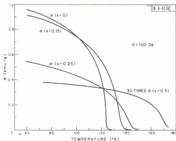
Fig. II-5. Magnetic moment versus temperature in  $\text{Ca}_{1-x}\text{Sr}_x\text{MnO}_3$  at atmospheric pressure.
