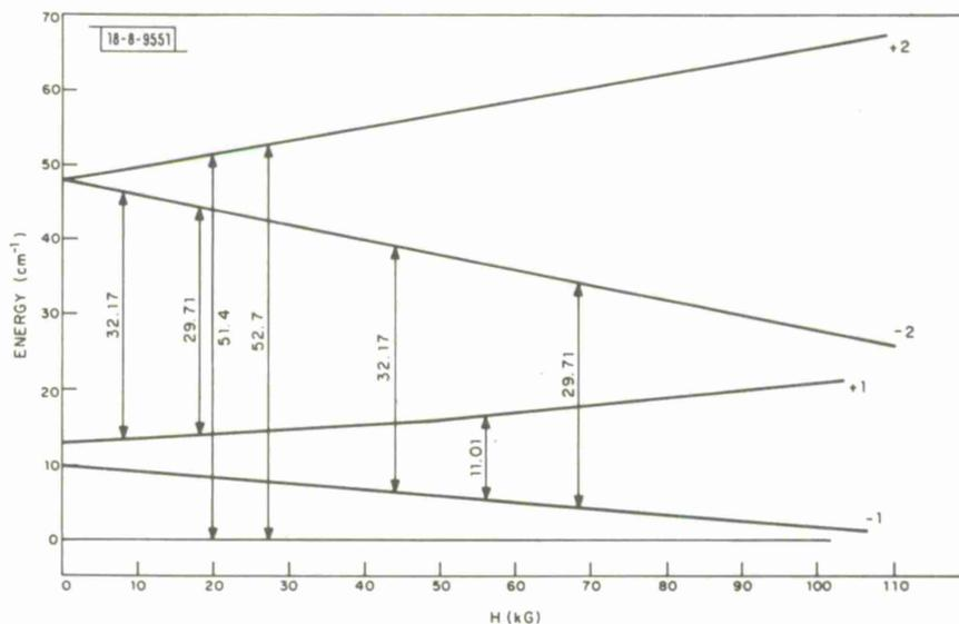
Fig. III-8. Approximate energy level diagram showing observed transitions. The  $11.01\text{-cm}^{-1}$  radiation was generated using a CSF carcinotron.
