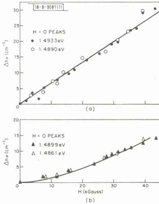
Fig. I-6. (a) Behavior of the 1.4933- and 1.4890-eV peaks in a magnetic field. Both peaks move linearly in H. (b) Shifts of 1.4861- and 1.4899-eV transitions in H are shown. As in Fig. I-6(a), both transitions move at same rate.
