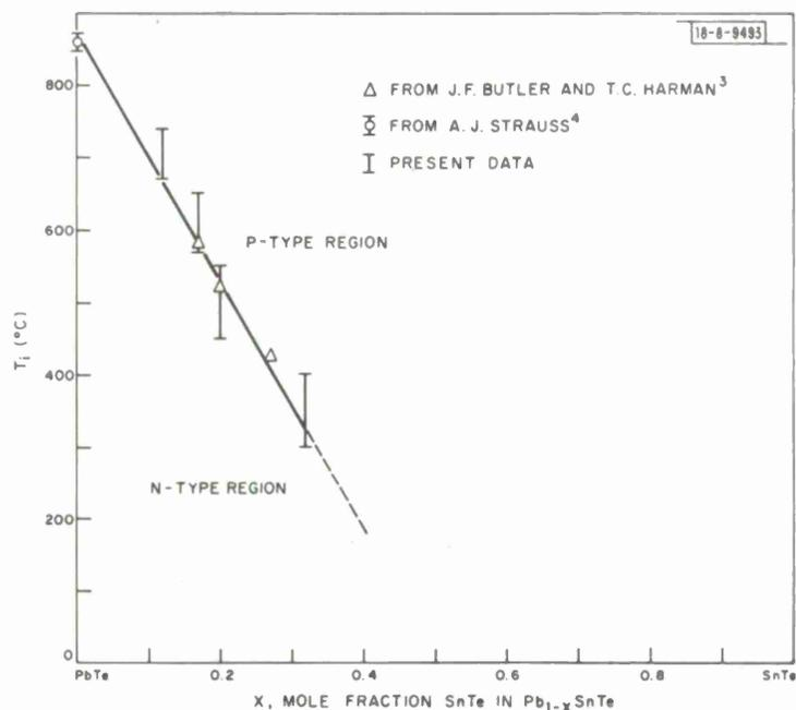
Fig. I-3. P-n crossover temperature  $T_i$  versus mole fraction SnTe for metal-saturated  $Pb_{1-x}Sn_xTe$ .
