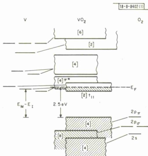
Fig. II-7. One-electron band structure for tetragonal  $\text{VO}_2$ .
