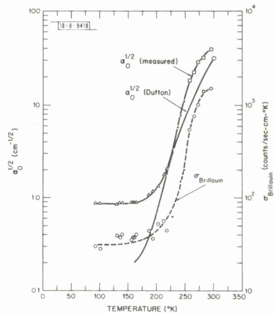
Fig. III-11. Resonant Brillouin scattering in CdS.
