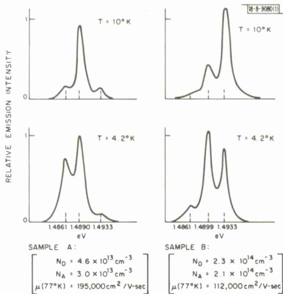
Fig. 1-5. Pertinent photoluminescence spectra from two GaAs epitaxial layers. Bottom two traces were taken with each sample at  $4.2^\circ K$ , upper two at  $10^\circ K$ .
