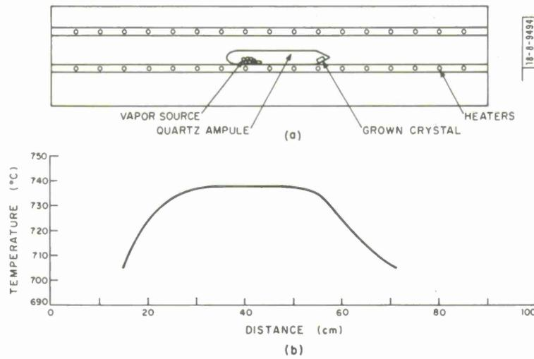
Fig. 1-4. (a) Schematic diagram of closed-tube horizontal crystal growth apparatus for  $Pb_{1-x}Sn_xTe$ . (b) Temperature profile for growing crystals by closed-tube horizontal growth technique.
