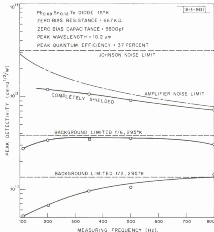
Fig. I-2. Peak detectivity ( $\lambda = 10.2 \mu\text{m}$ ) of 15-mil-square  $\text{Pb}_{0.88}\text{Sn}_{0.12}\text{Te}$  diode at 15°K as a function of frequency and background.
