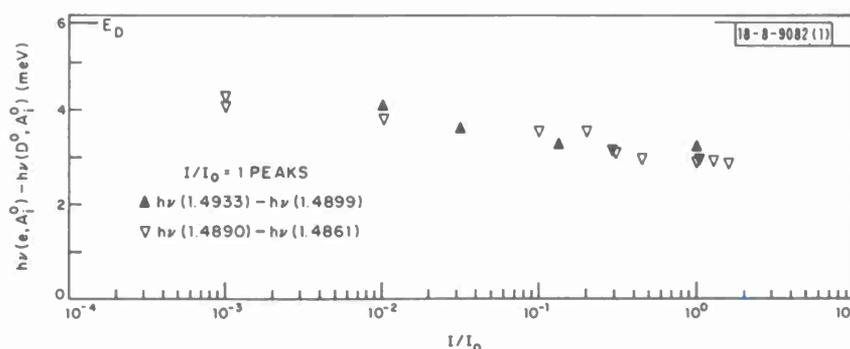
Fig. I-7. Solid triangles are separation in energy (meV) between 1.4933- and 1.4899-eV transitions as  $I/I_0$  is varied. Open triangles represent same data for pair 1.4890 and 1.4861 eV. As  $I/I_0$  is decreased, 1.4899- and 1.4861-eV transitions shift to lower energies causing increase in separation. Data in Figs. I-5 and I-6 were taken at  $I/I_0 = 1$ .
