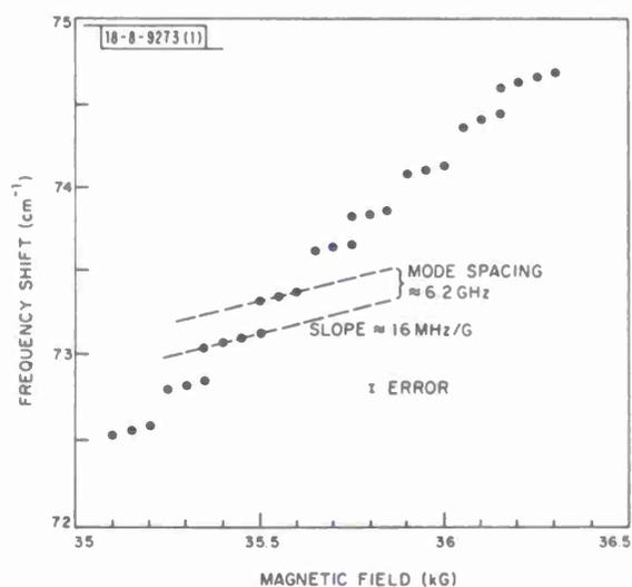
Fig. I-9. Variation of collinear geometry spin-flip Raman laser output frequency with magnetic field ( $\lambda_{\text{pump}} = 5.32 \mu\text{m}$ ,  $T \sim 30^\circ\text{K}$ , concentration  $\sim 1 \times 10^{16} \text{ cm}^{-3}$ , sample length = 4.8 mm).
