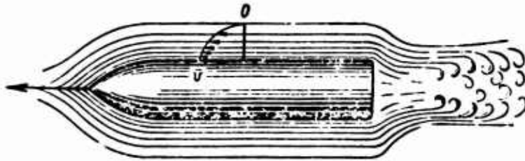
Figure 24. The Boundary Layer and Formation of Vortexes.
