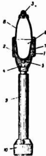
Figure 94. A Shaped Charge Rocket: 1, Casing; 2, Explosive charge; 3, Fuze; 4, Detonator; 5, Central Tube; 6, Cumulative Recess; 7, Metal Cone; 8, Nose; 9, Jet Chamber; 10, Stabilizer.
