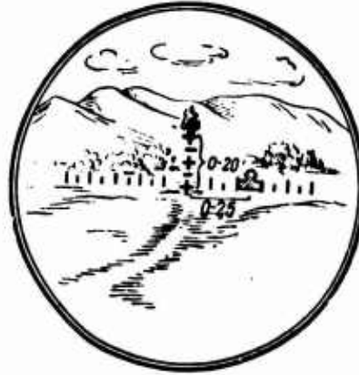
Figure 50. Measuring Angles Using Binoculars.
