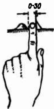
Figure 51. Measuring Angles Using a Finger.
