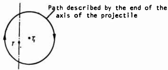
Figure 36. Slow Conical Movement on the Curvilinear Section of the Trajectory. View from the rear.
