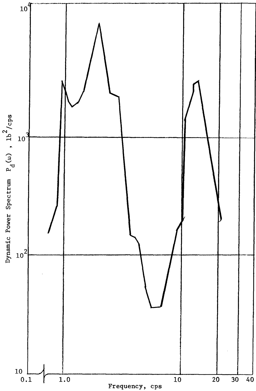
Figure 7. Vehicle Response-Frequency Relation
