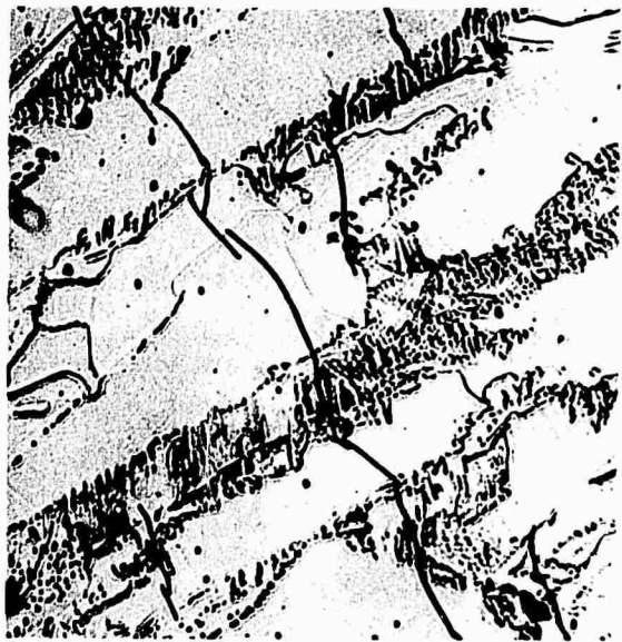
Figure 8. Arc melted Pr-89 at. %Co alloy. This alloy is primarily \text{Pr}_2\text{Co}_{17} with some \text{PrCo}_5 and just detectable amounts of free cobalt. 250 X
