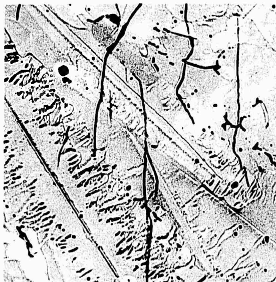
Figure 9. Arc melted Nd-89 at. %Co alloy. This alloy is essentially single phase \text{Nd}_2\text{Co}_{17} even though \text{Nd}_2\text{Co}_{17} forms by peritectic reaction. 250 X
