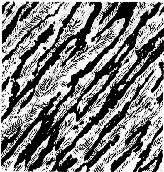
Figure 7. Arc melted Ce-89.5 at. %Co alloy. Cobalt dendrites peritectically surrounded by \text{Ce}_2\text{Co}_{17} . The dark phase is \text{CeCo}_5 . 250 X
