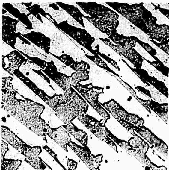
Figure 12. Pr-89 at. %Co homogenized 50 hours at 1100°C. Single phase \text{Pr}_2\text{Co}_{17} , light and dark regions are annealing twins. 250 X
