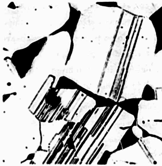
Figure 17. Pr-87 at. %Fe homogenized 8 hours at 1000°C. Large grains of \text{Pr}_2\text{Fe}_{17} , some heavily twinned, with dark voids which originally contained Pr + \text{Pr}_2\text{Fe}_{17} eutectic. 250 X
