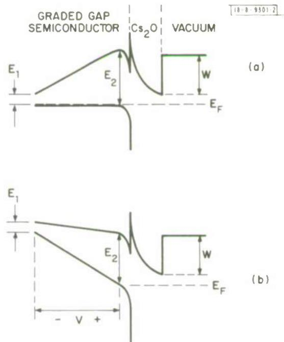
Fig. 2. Energy level diagram of a Cs<sub>2</sub>O coated graded-gap semiconductor photoemitter with (a) no bias applied and (b) a bias voltage  $V$  applied to the graded gap region.
