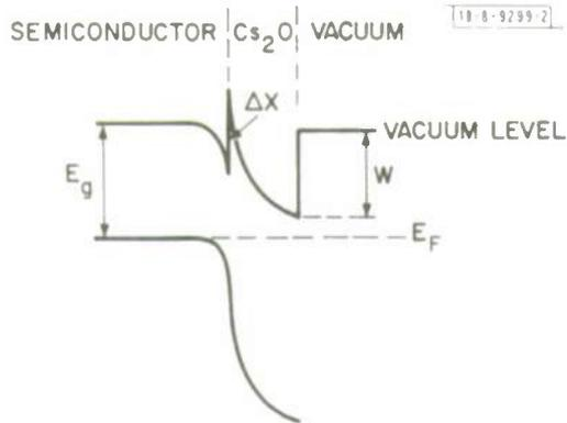
Fig. 1. Energy level diagram of a Cs<sub>2</sub>O coated semiconductor photoemitter.  $W$  is the work function of the Cs<sub>2</sub>O coating and  $\Delta X$  is the difference in electron affinities of the semiconductor and the Cs<sub>2</sub>O coating.
