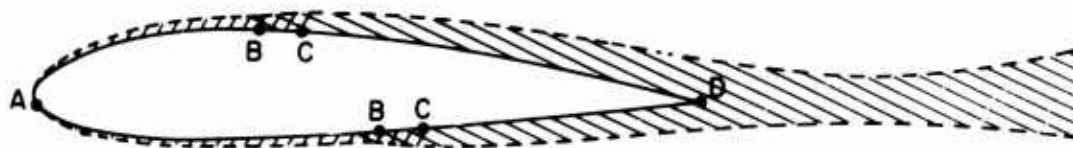
Figure 1. Boundary-layer flow along an airfoil.
