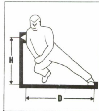
Figure 5. Lateral push with the preferred shoulder. Reaction force provided by a footrest. (D measured from the leading edge of the footrest.)
