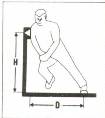
Figure 4. Lateral push with the preferred shoulder. Reaction force provided by friction. (D measured from the center of the shoe.)
