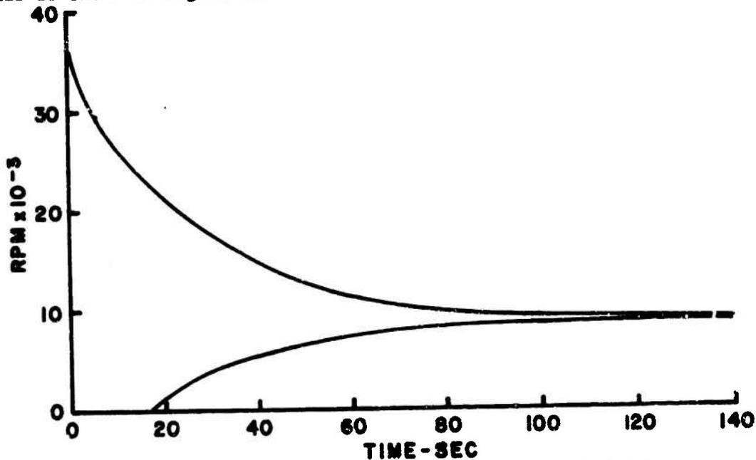
Figure 21. Roll Damping, Free Spinning Serrated Model
