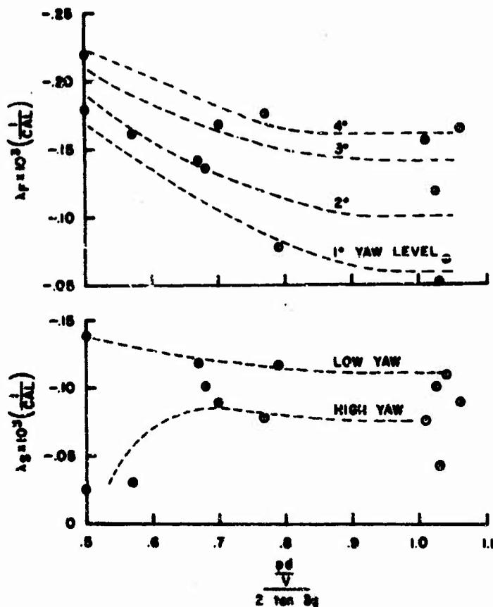
Figure 23. The Exponential Damping Coefficients, Sarp 1B Models
