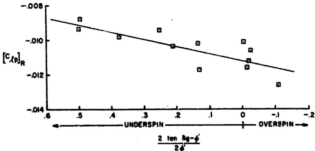
Figure 22. Rolling Moments, Caliber .30 Sarp 1B Model, Mach 1.42
