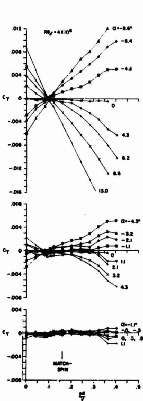
Figure 6. Serrated A-N Spinner Yaw Force Coefficient Data Trends for Several Angle of Attack Ranges at a Reynolds Number of  $4 \times 10^6$
