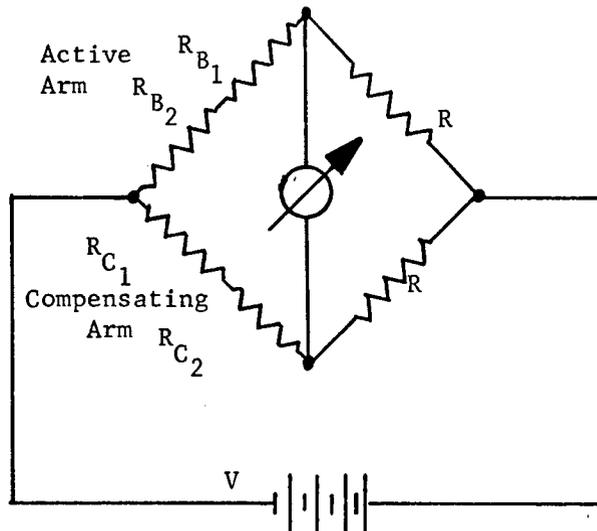
FIGURE B-2. Typical Strain Gage Bridge Circuit
