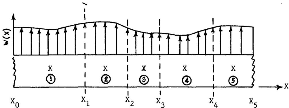
FIGURE C-5. Missile Station Load Application
