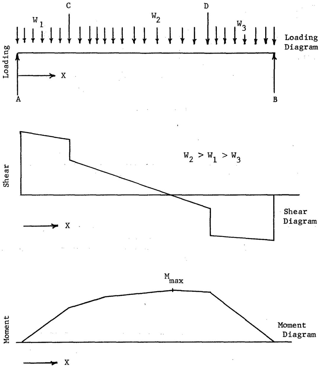
FIGURE C-1. Typical Loading, Shear, and Moment Diagrams
