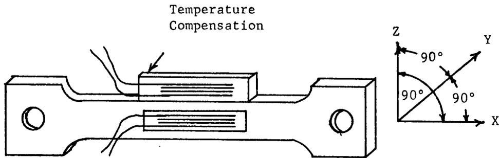
FIGURE B-1. Typical Strain Bar Design
