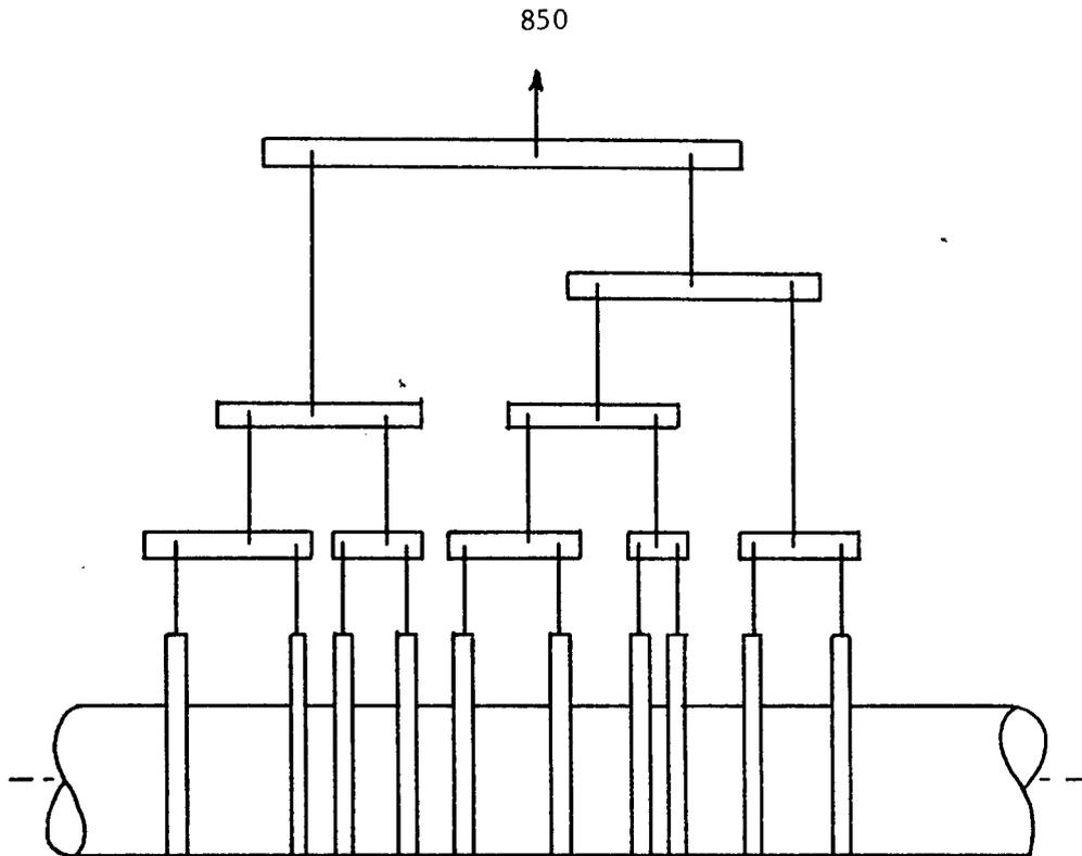
FIGURE A-4. Physical Arrangement of Whiffletree
