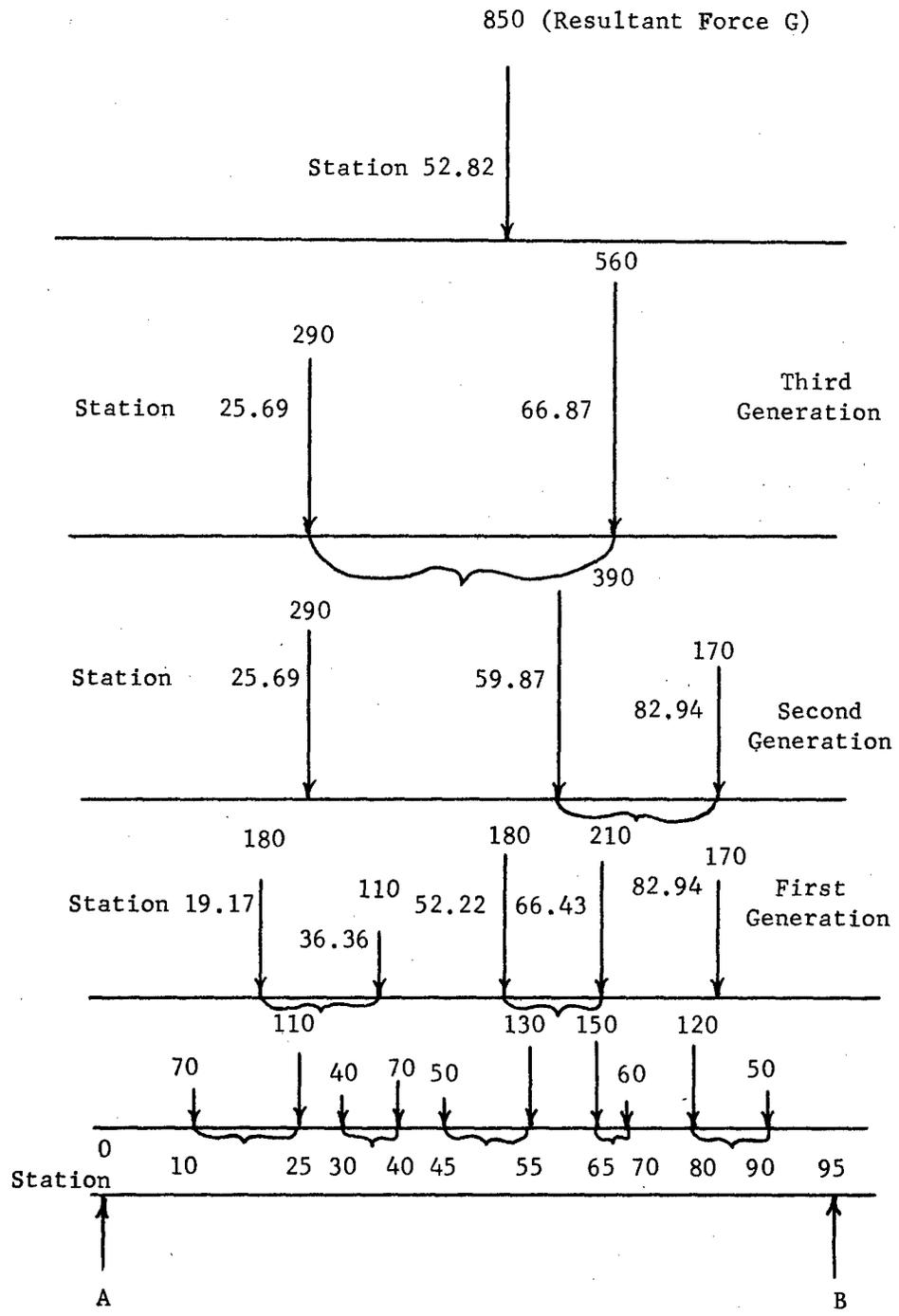
FIGURE A-3. Whiffletree Load Distribution
