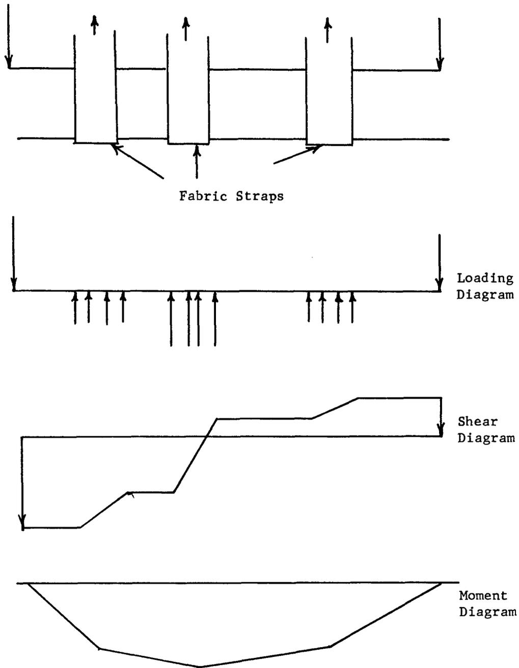
FIGURE C-2. Fabric Straps on Test Specimen and Resultant Diagrams
