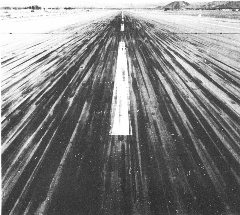
Figure 17. Sections of test paints at NAS, Point Mugu after 26-1/2 months.
