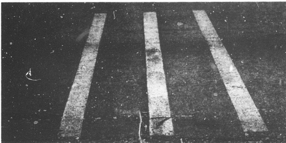
Figure 14. Set of stripes of Formulation 114 at USNS, Guam 1 year after application. Left to right: single-thickness, reflectorized; double-thickness, reflectorized; single-thickness, unreflectorized.
