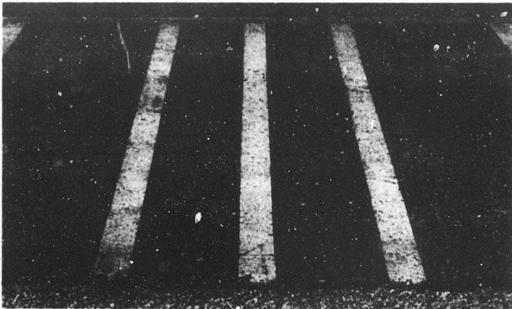
Figure 13. Set of stripes of Formulation 101 at USNS, Guam 1 year after application. Left to right: single-thickness, reflectorized; double-thickness, reflectorized; single-thickness, unreflectorized.
