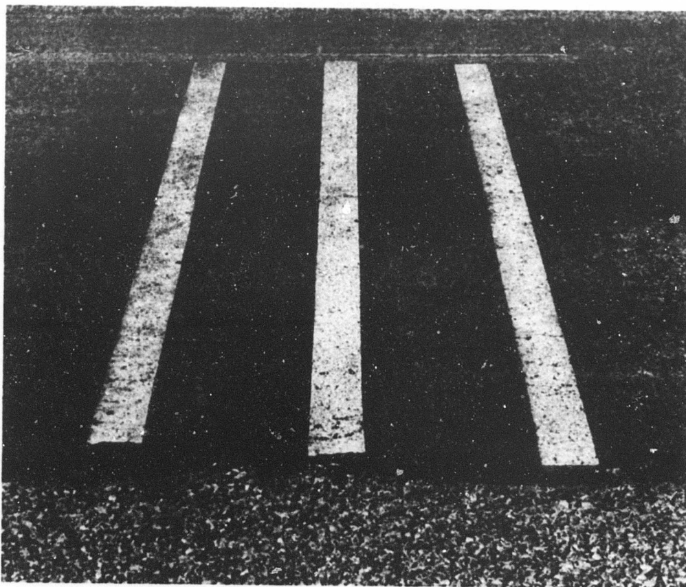
Figure 10. Set of stripes of Formulation 110 at USNS, Guam 1 year after application. Left to right: single-thickness, reflectorized; double-thickness, reflectorized; single-thickness, unreflectorized.
