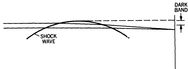
8.9 Two rays intersecting film at a common point
