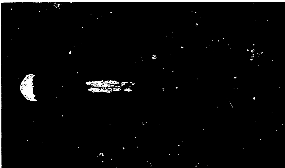
8.2 Self-luminous photograph of an ablating polycarbonate round-nosed, large-angle cone at a velocity of 7 km/sec, ambient density of 0.066 atmospheres
