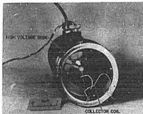
Figure 8. Pipe mounted ion drift sensor.
