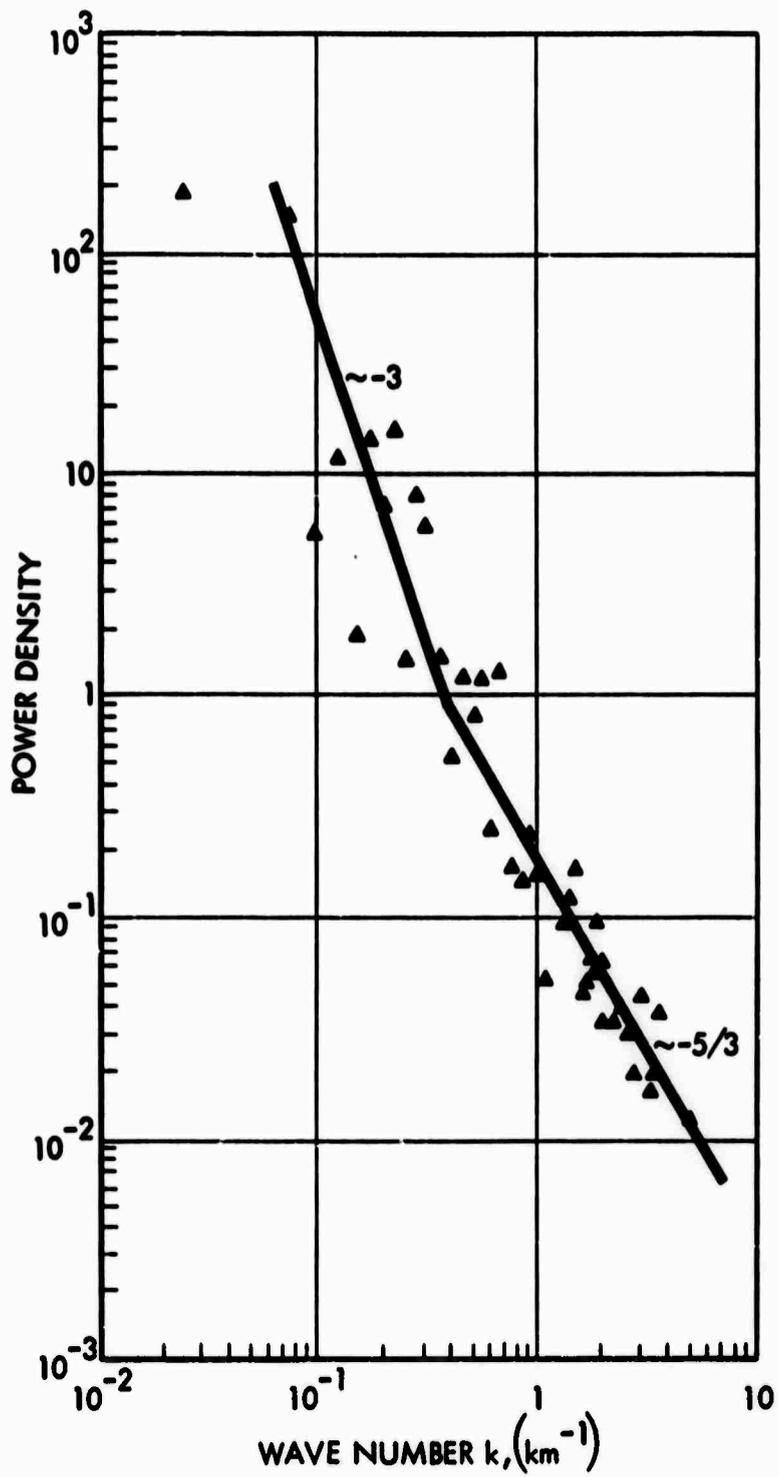
FIGURE 3-7. Transversal Component of Power Spectrum  $h = 50$  km
