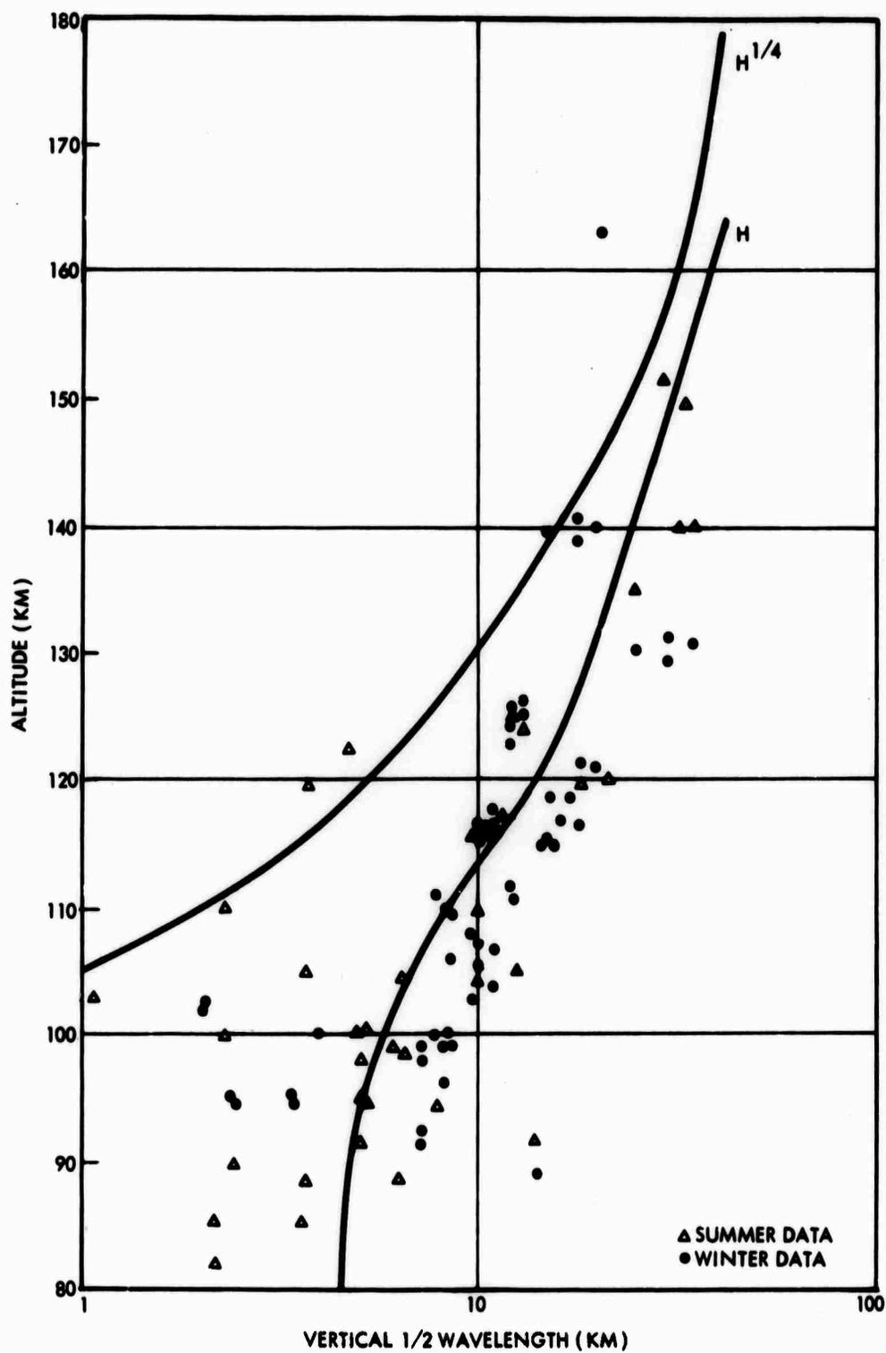
FIGURE 2-1. Minimum Vertical Scale of Internal Gravity Waves. (The curve  $H^{1/4}$  is drawn according to Hines (1964) following Eq. 2-11, and the curve  $H$  represents the result of the turbulent theory in Eq. 2-13.)
