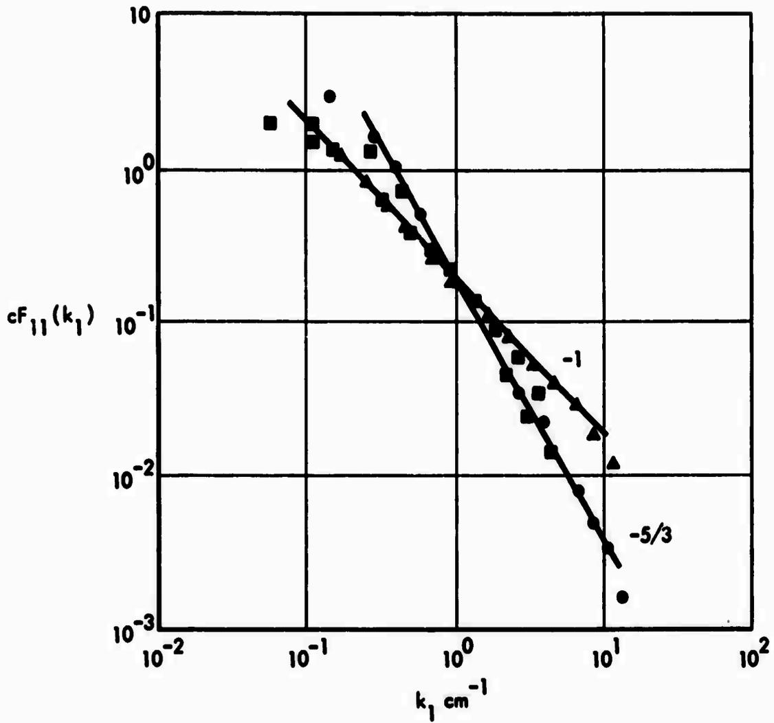
FIGURE 3-1. Longitudinal Energy Spectrum in a Boundary Layer and in a Pipe (For Data See Table 3-2, for discussions on experiments, see Tchen 1954)
