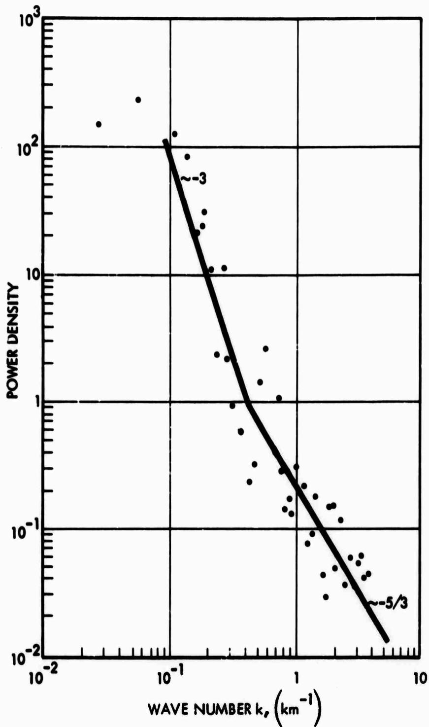
FIGURE 3-6. Longitudinal Component of Power Spectrum at  $h = 50$  km (Zimmerman et al., 1969)
