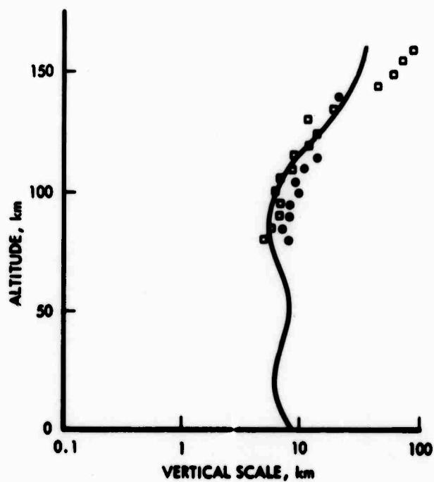
**FIGURE 4-5. Vertical Scale of Turbulence. Data From the Structure Function (●) and From the Correlation Function (□). The Smooth Line is the Scale Height Based Upon the 1962 U.S. Standard Atmosphere Variation. (Data are drawn from Elford and Roper, 1966)**
