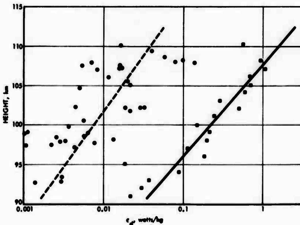
FIGURE 4-10. Dissipation of Energy by Molecular Motions. The Solid Line Represents  $\epsilon_d$  from the Viscous Dissipation and the Dotted Line Represents  $\epsilon_d$  from the Globule Diffusion (Justus, 1966)
