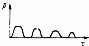
Fig. 22.19. Nature of the diagram pressure - time during anomalous combustion.
