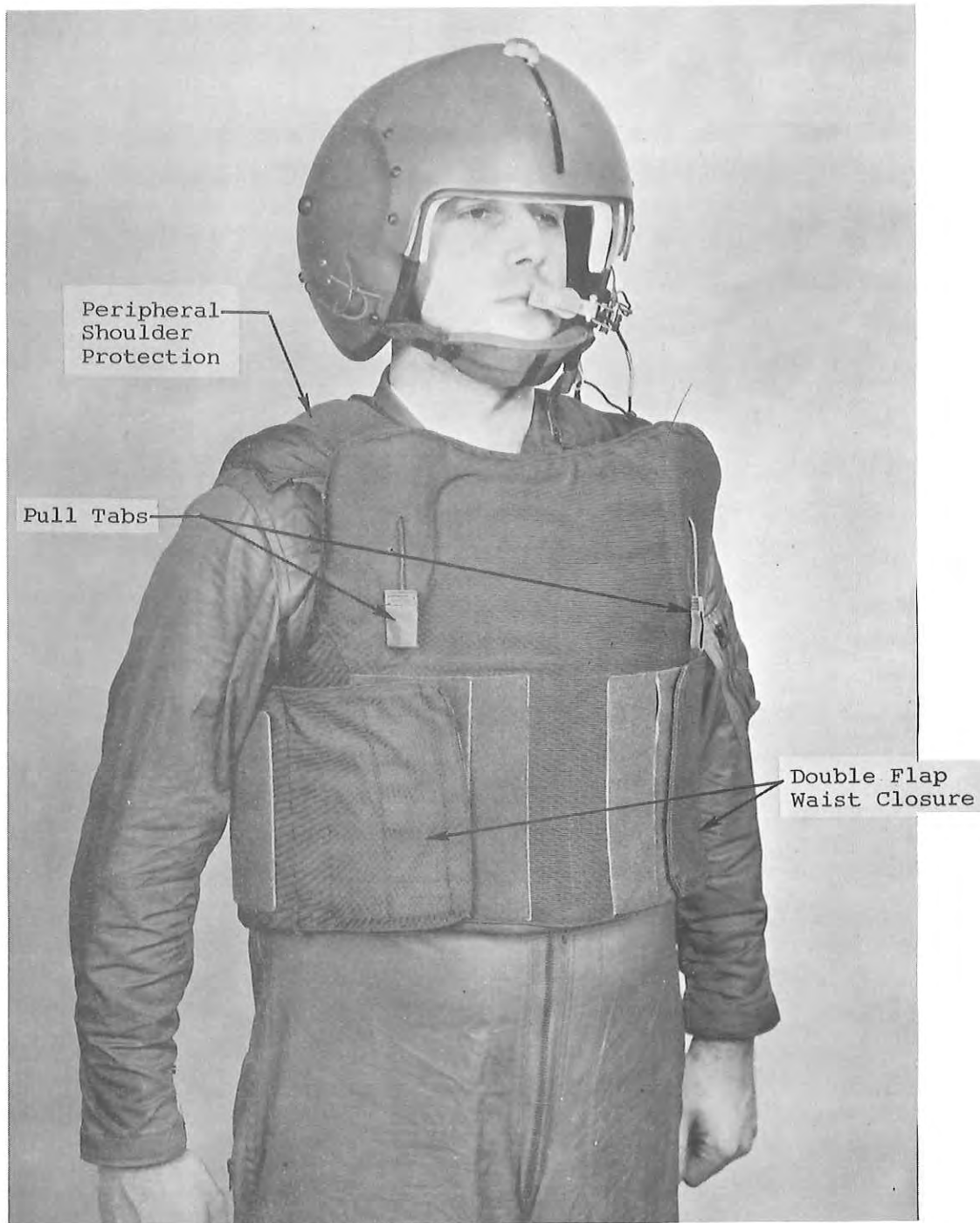
Figure 2. Prototype #1 Front View - Over-the-Shoulder Raschel Knit, Tension-Web Suspension - Quick-Release Buckle Shoulder Breaks
