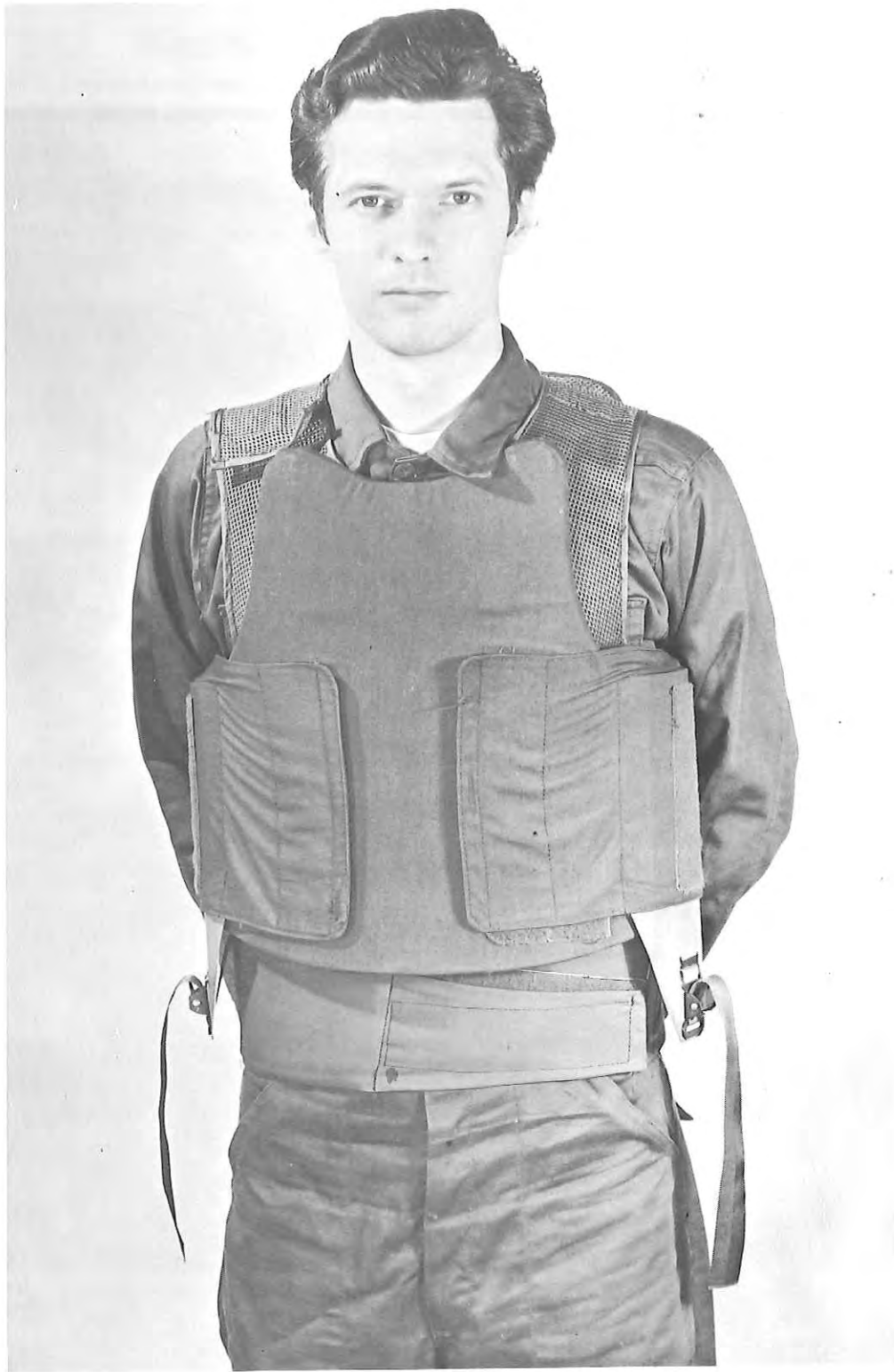
Figure 25. Approach #4 - Waist Augmentation Belt - Load Transferred to Waist and Hips
