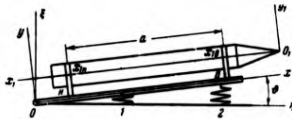
Fig. 5.3. Simplified dynamic model of a vehicle-erector system.
