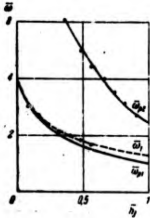
Fig. 12.10. Effect of the level of liquid in tanks on frequencies of natural oscillations of the system (points show experimental values of frequencies).
