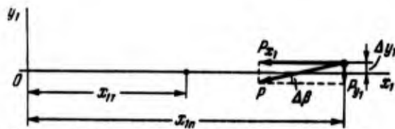
Fig. 1.6. Component forces of thrust in a connected system of coordinates.
