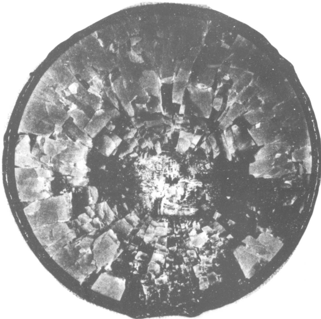
Figure 1c. FRACTURE PATTERNS OF GLASS-CERAMICS FOLLOWING BALLISTIC IMPACT BY CALIBER .30 M2 PROJECTILES
