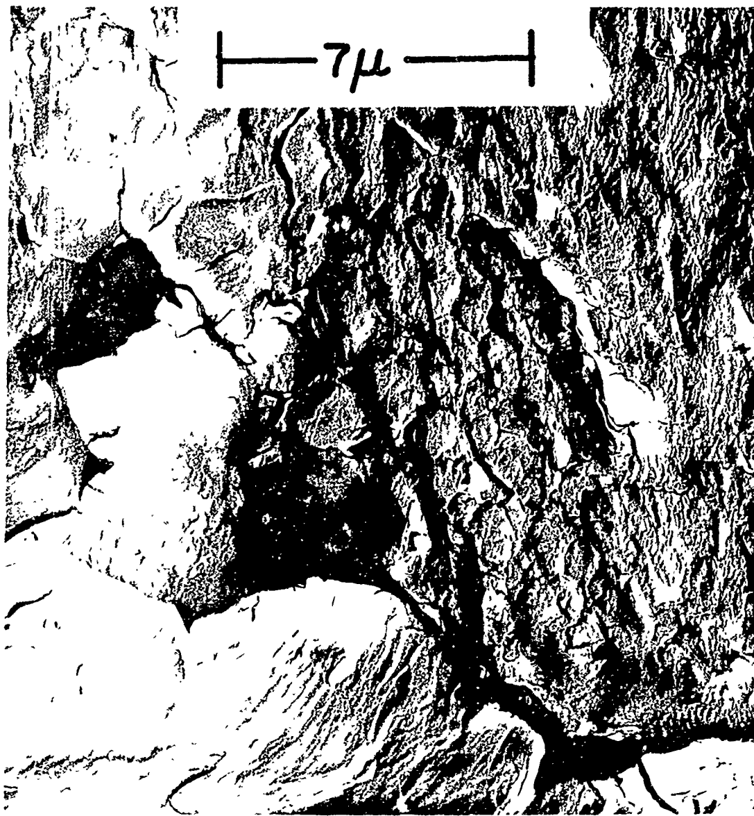
Fig. 9 - Typical combination of striations and microvoid coalescence seen on the fatigue surfaces of Ti-7Al-2.5Mo (T94) cycled in air at low stress-intensity ( \Delta K = 30 \text{ ksi } \sqrt{\text{in.}} ). Two-stage cellulose acetate replica.
