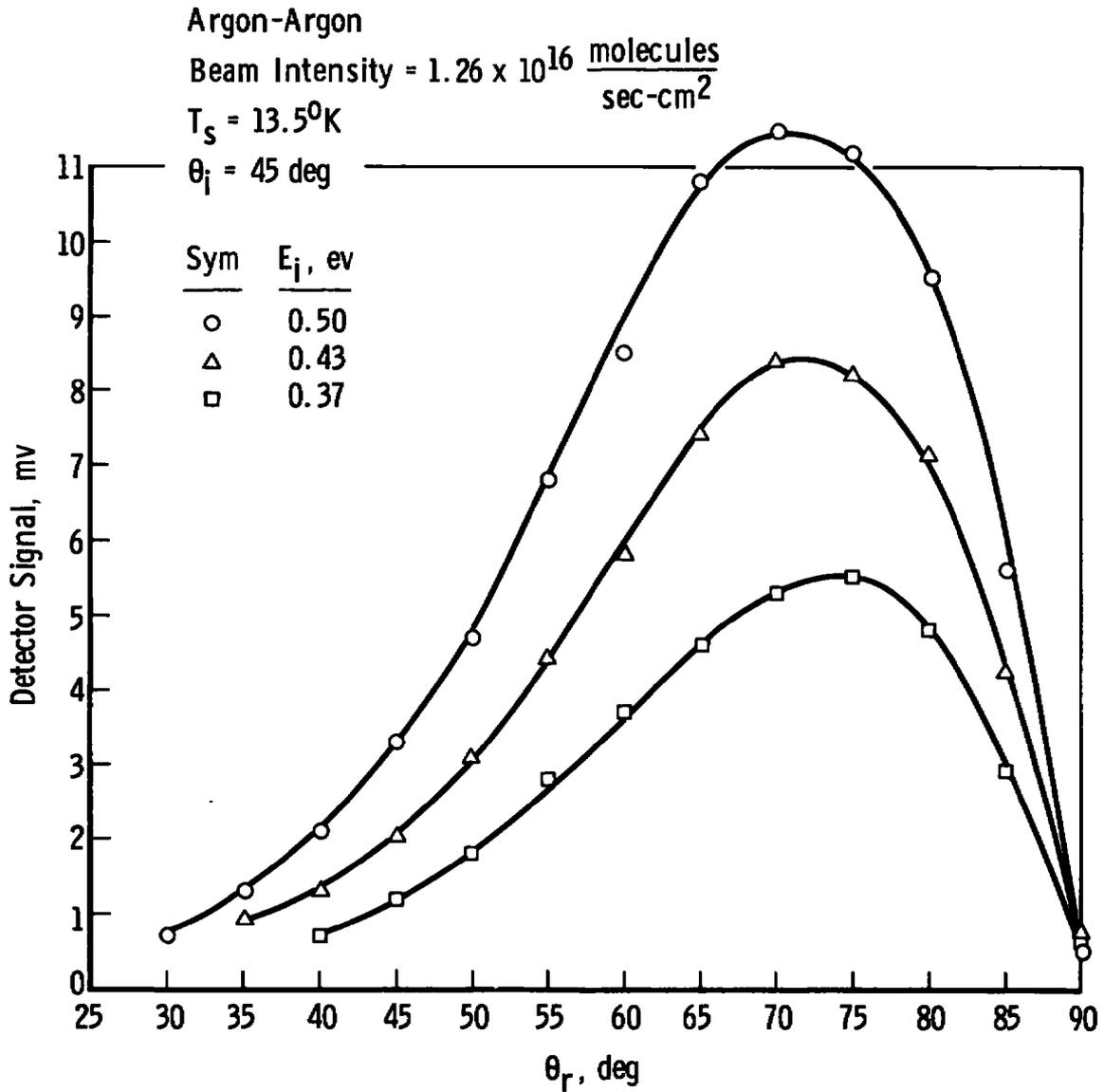
Fig. 24 In-Plane Scattering Distributions for Various Beam Energies ( $\theta_i = 45$  deg)
