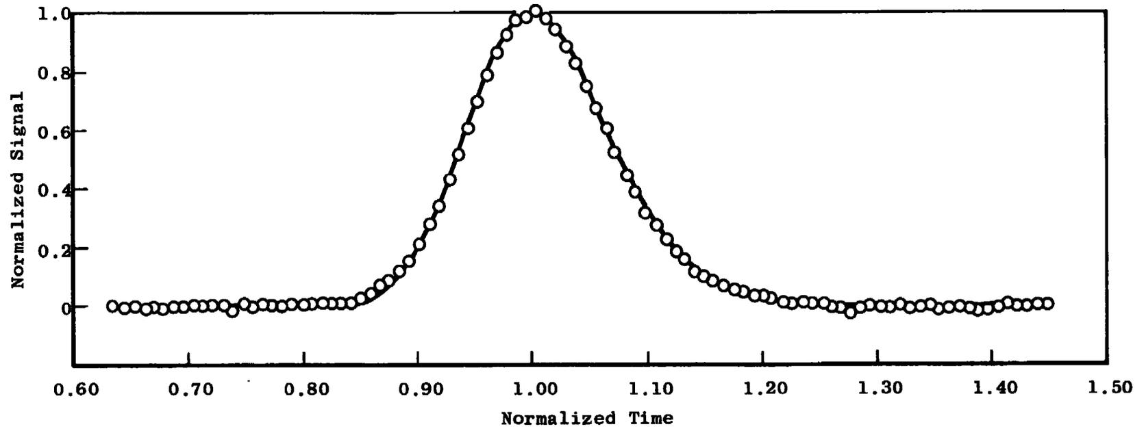
Fig. 10 Time-of-Flight Distribution of a 0.43-eV Argon Beam
