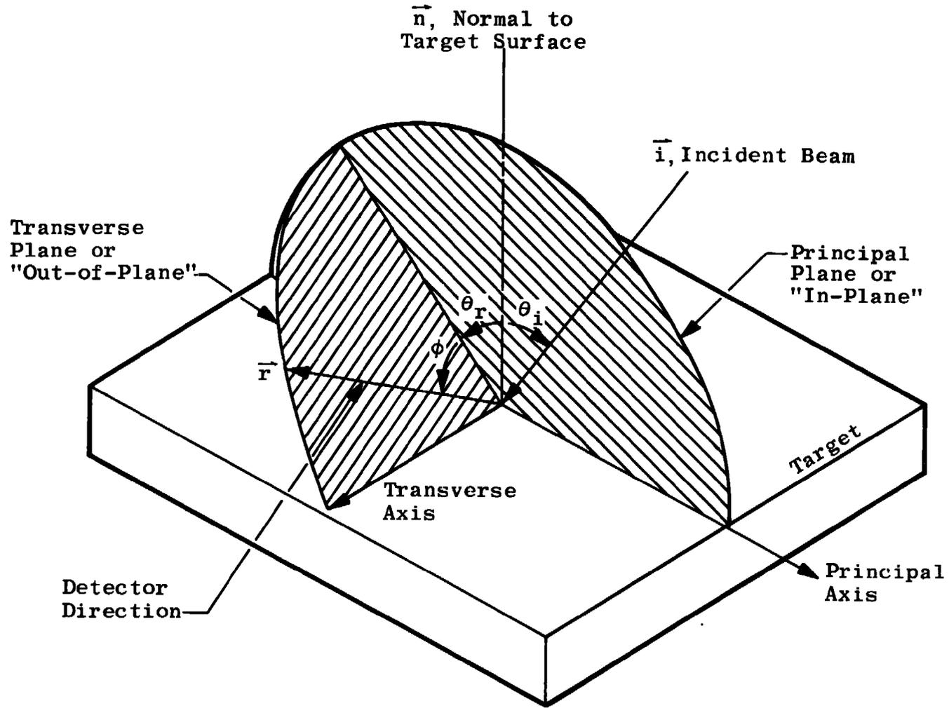
Fig. 8 Orientation Parameters for the Reflected Beam
