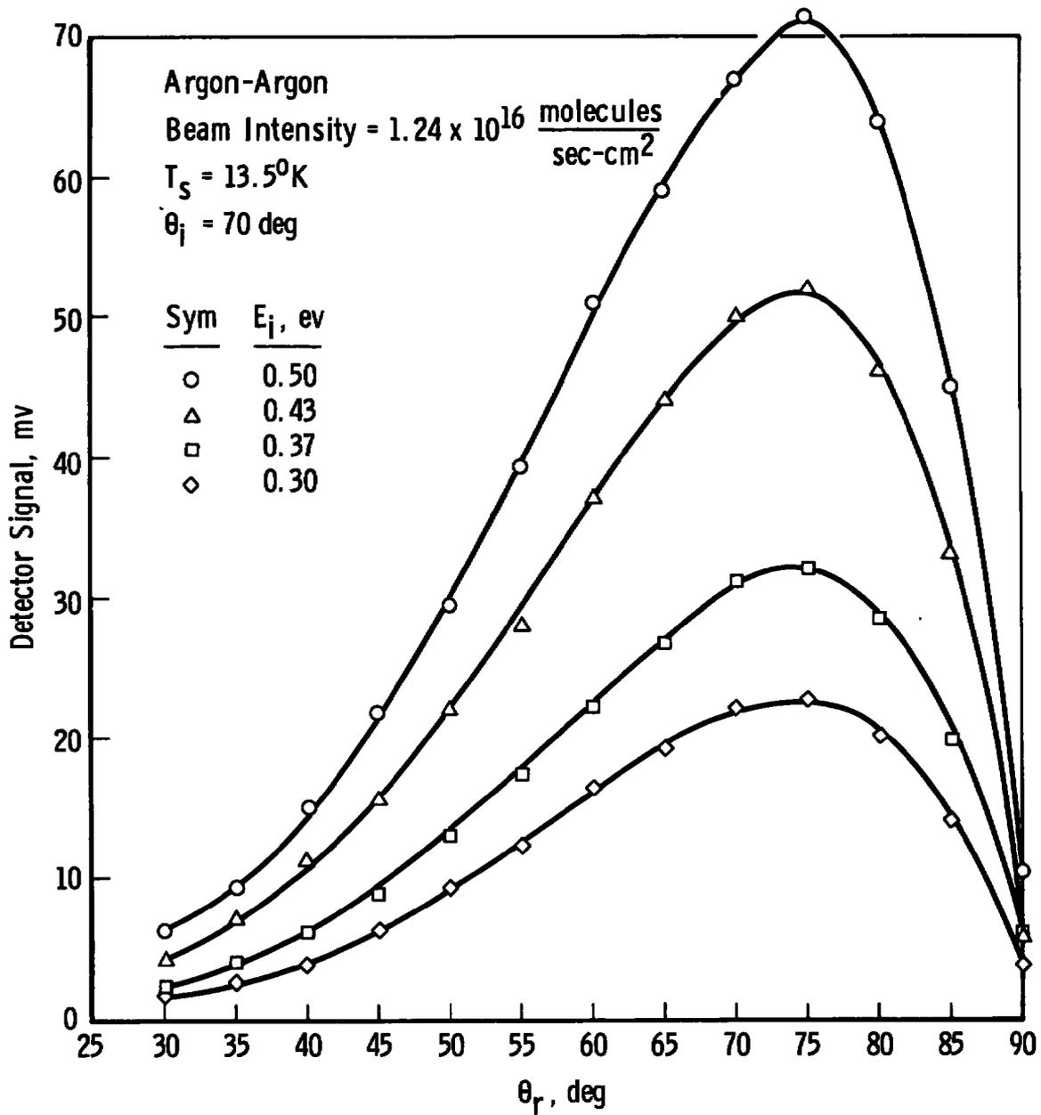
Fig. 22 In-Plane Scattering Distributions for Various Beam Energies ( $\theta_i = 70 \text{ deg}$ )
