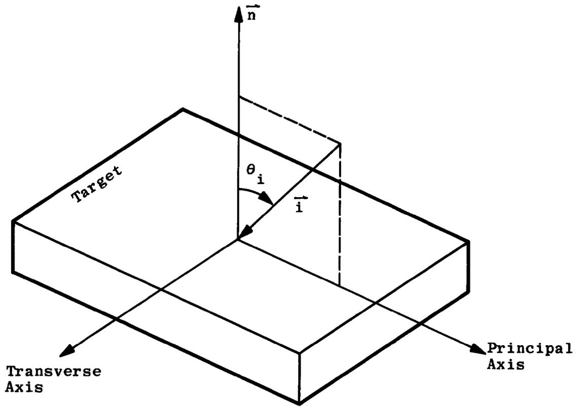
Fig. 7 Orientation Parameters for the Incident Beam
