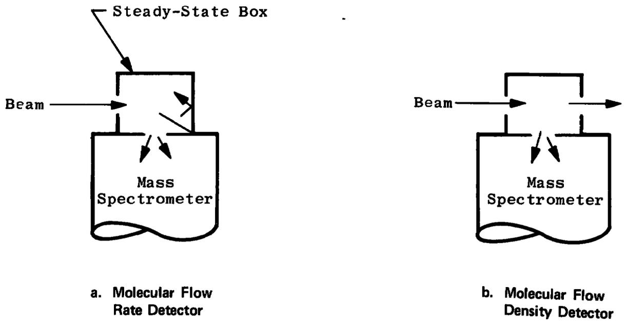
Fig. 5 Operational Modes of the Detector
