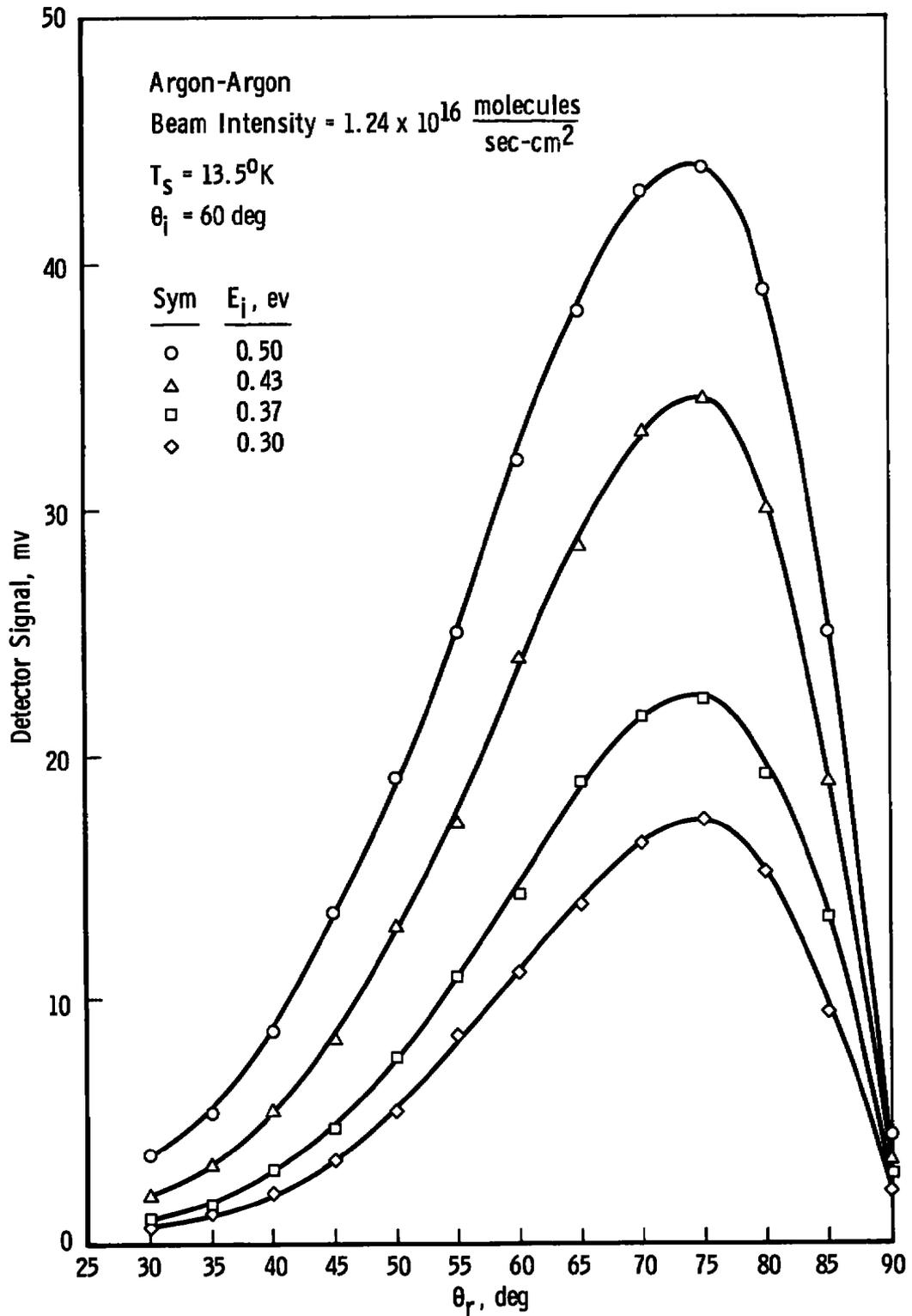
Fig. 23 In-Plane Scattering Distributions for Various Beam Energies ( $\theta_i = 60 \text{ deg}$ )
