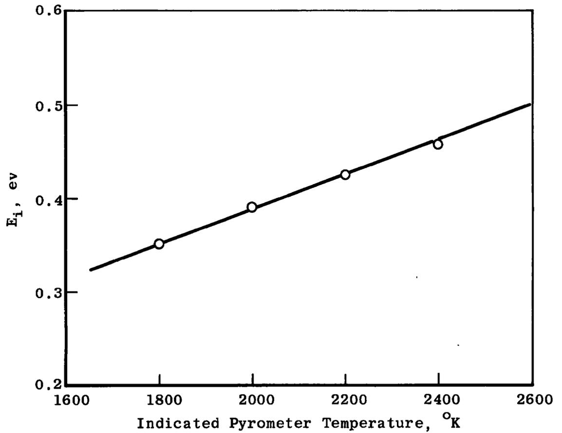
**Fig. 11 Argon Beam Energy for Corresponding Source Temperatures**
