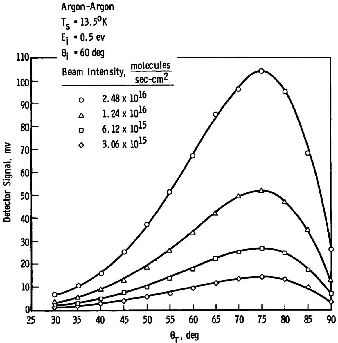
Fig. 16 In-Plane Scattering Distributions for Various Beam Intensities
