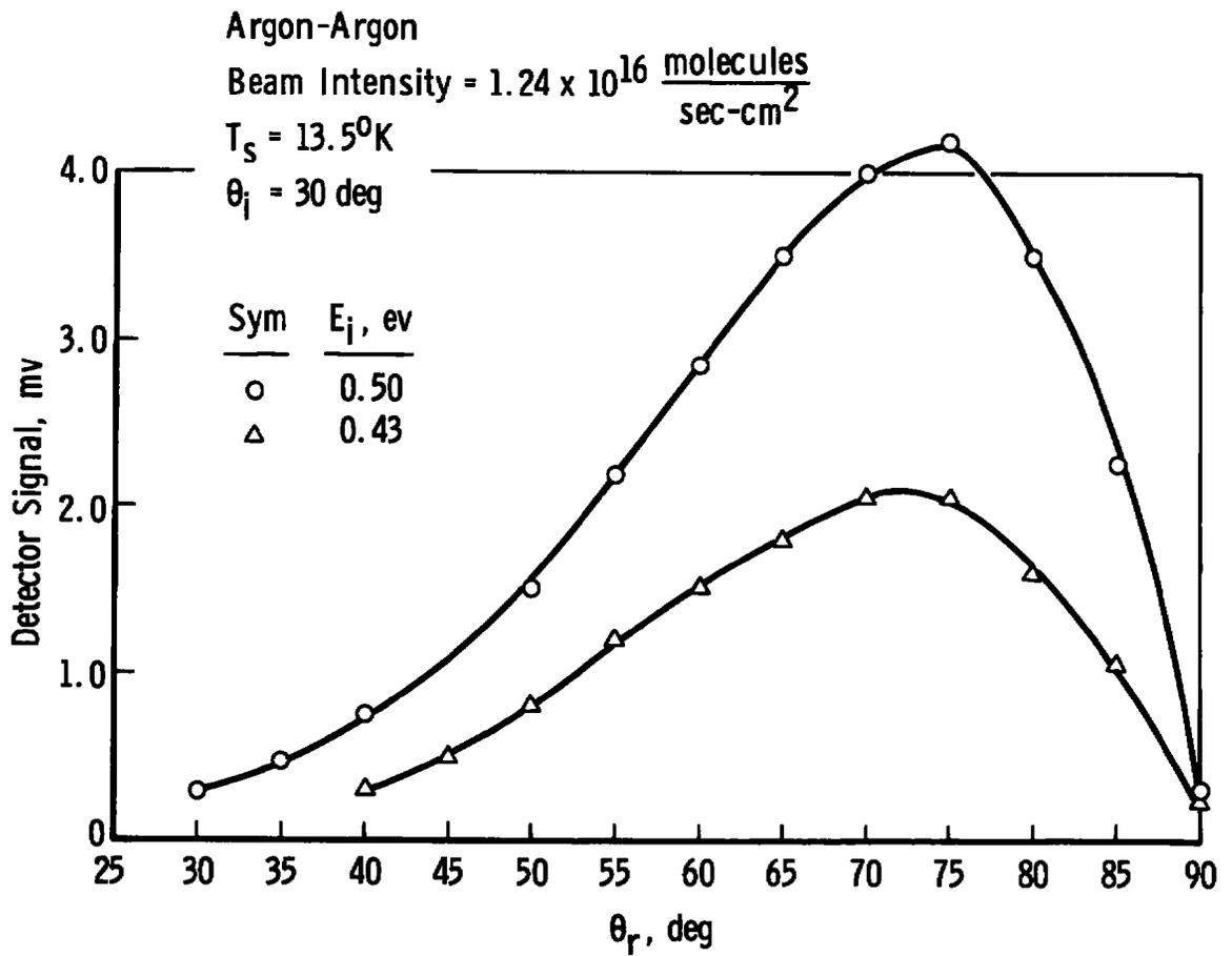
Fig. 25 In-Plane Scattering Distributions for Various Beam Energies
