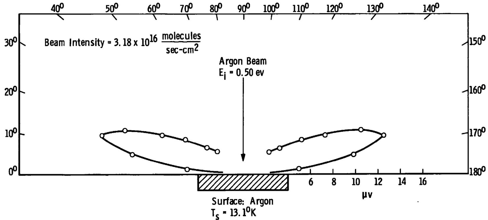
Fig. 26 In-Plane Scattering Distribution for a 0.5-eV Argon Beam at  $\theta = 0$  deg
