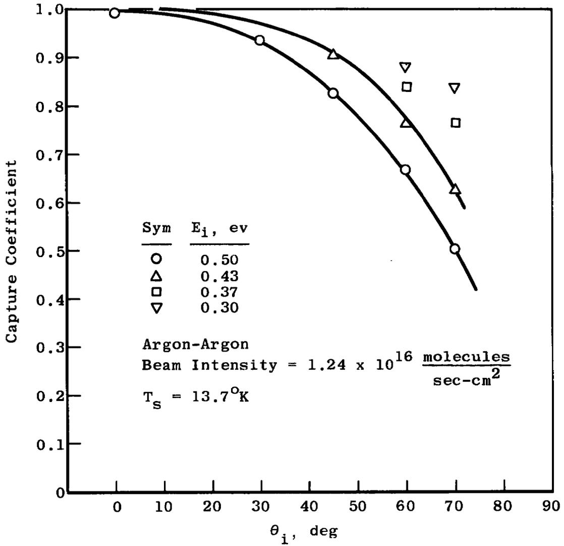
Fig. 30 Beam Capture Coefficient for Various Beam Incidence Angles
