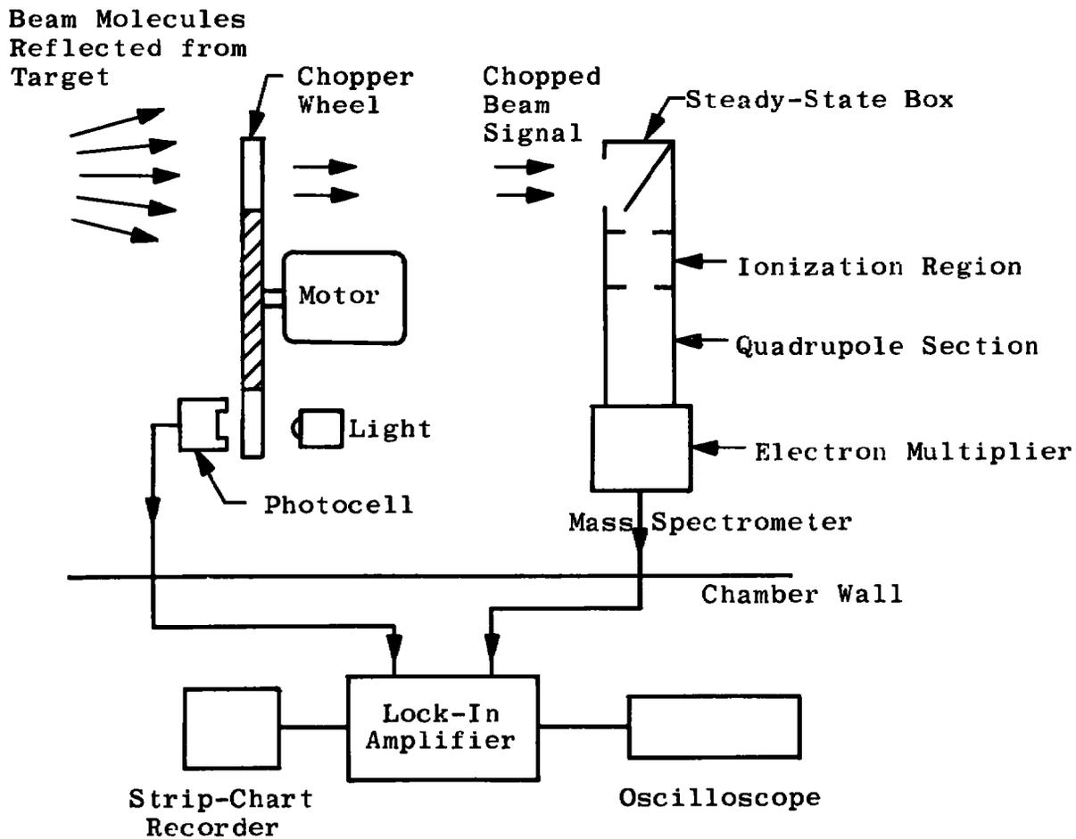
Fig. 4 Mass-Spectrometric Modulated Beam Detector
