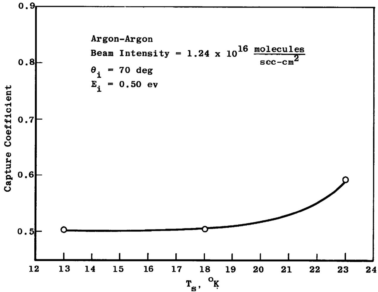
Fig. 32 Beam Capture Coefficient for Various Surface Temperatures
