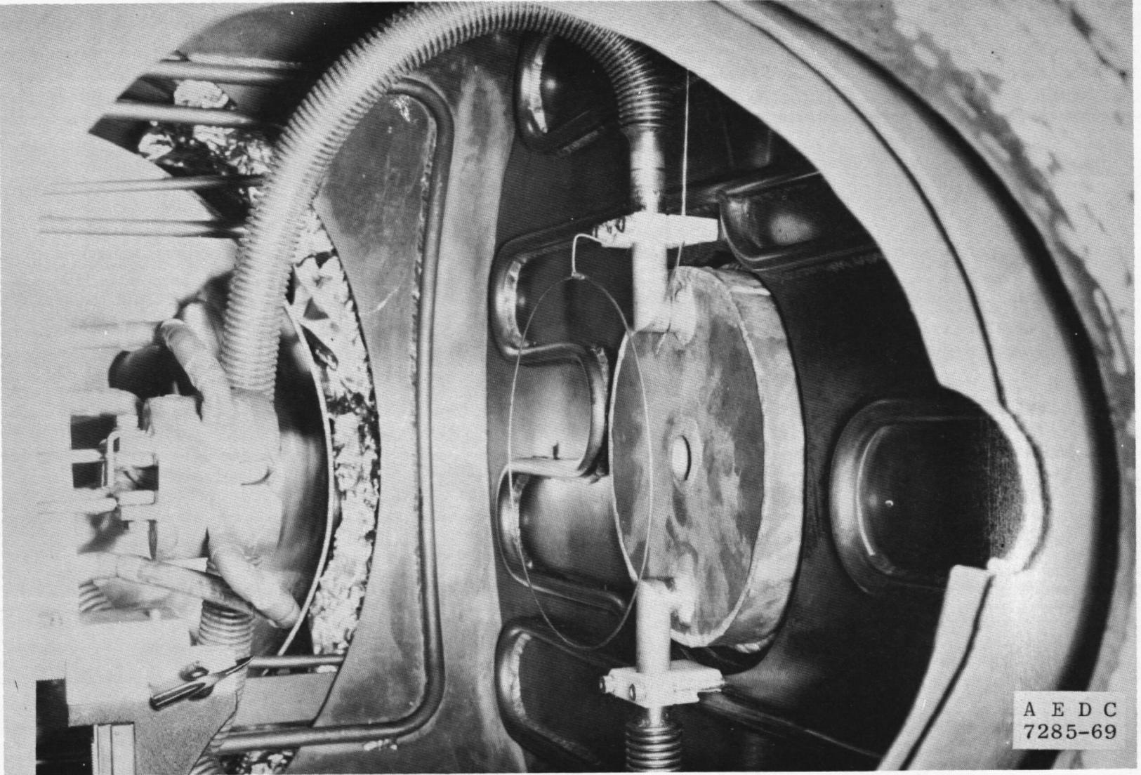
Fig. 3 Tantalum Gas Source and Cryogenically Cooled Skimmer
