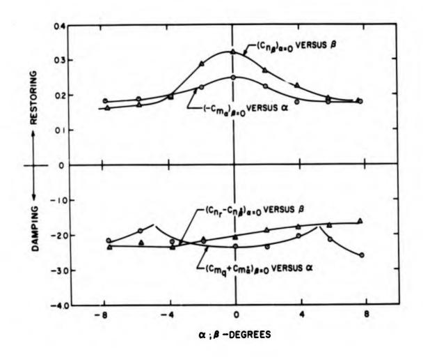
Figure 5 Restoring and Damping Derivatives, Nose 3
