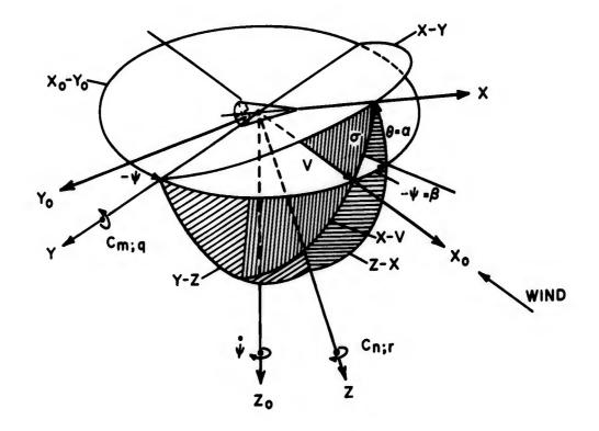
Figure 1 Coordinate System and Nomenclature for Non-Rolling Body in Rectilinear Flight (Wind Tunnel Simulation)
