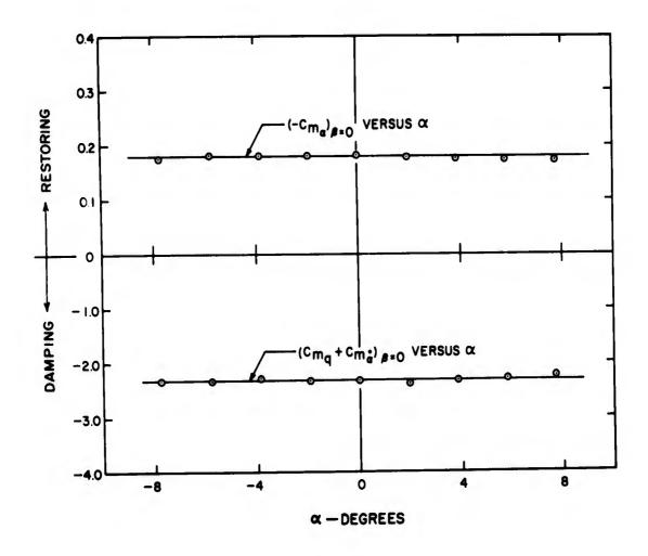
Figure 3 Restoring and Damping Derivatives, Nose 1
