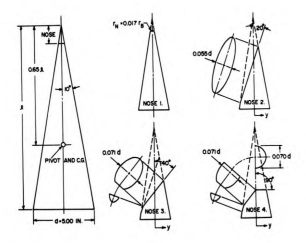
Figure 2 Model Configurations
