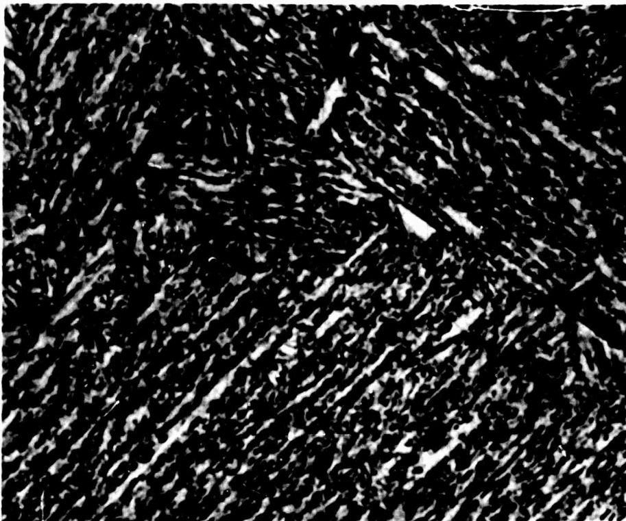
FIGURE 6 AFC SHEET AUSTENITIZED 1 HR AT 2200 o F FOLLOWED BY 100 HRS AT 1900 o F. THE DELTA FERRITE SHOWN IN FIGURE 5 HAS BEEN REMOVED AND THE AUSTENITE GRAIN SIZE HAS INCREASED. (x 800).
