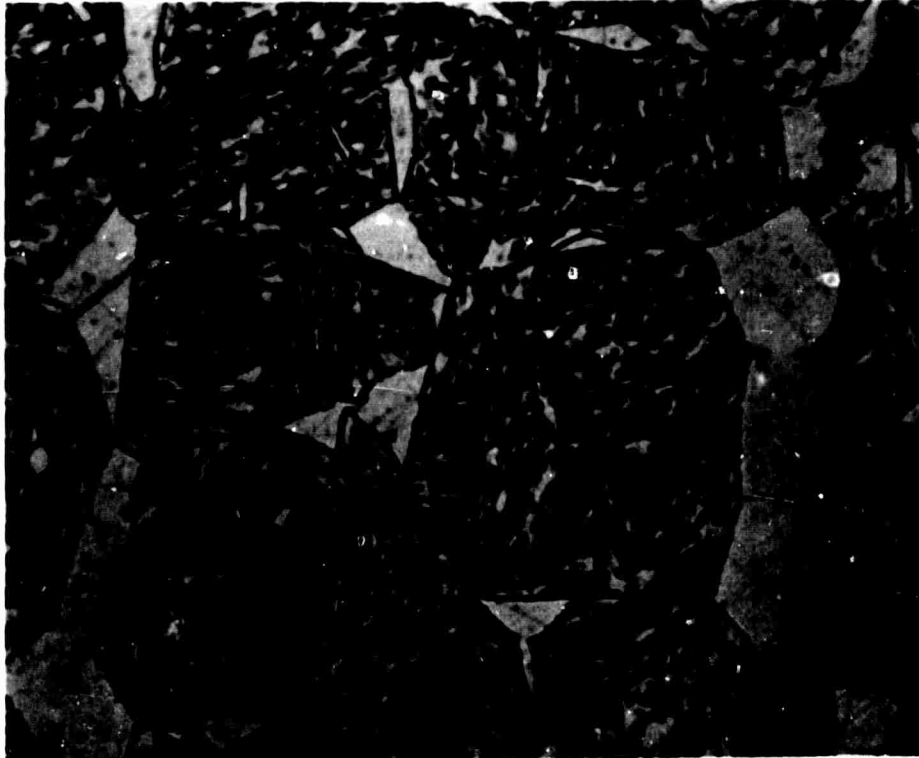
FIGURE 5 AFC 77 SHEET AUSTENITIZED 1 HR AT 2200 o F AND WATER QUENCHED, SHOWING DELTA FERRITE (x 800)
