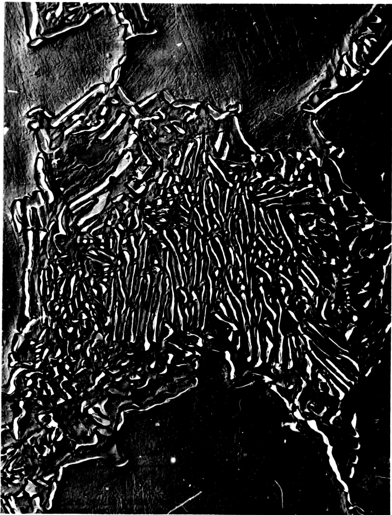
FIGURE 7 EUTECTIC-LIKE REMAINS OF A LARGE BLOCK OF DELTA FERRITE IN AFC 77 SHEET AT 1600°F (x 6000).
