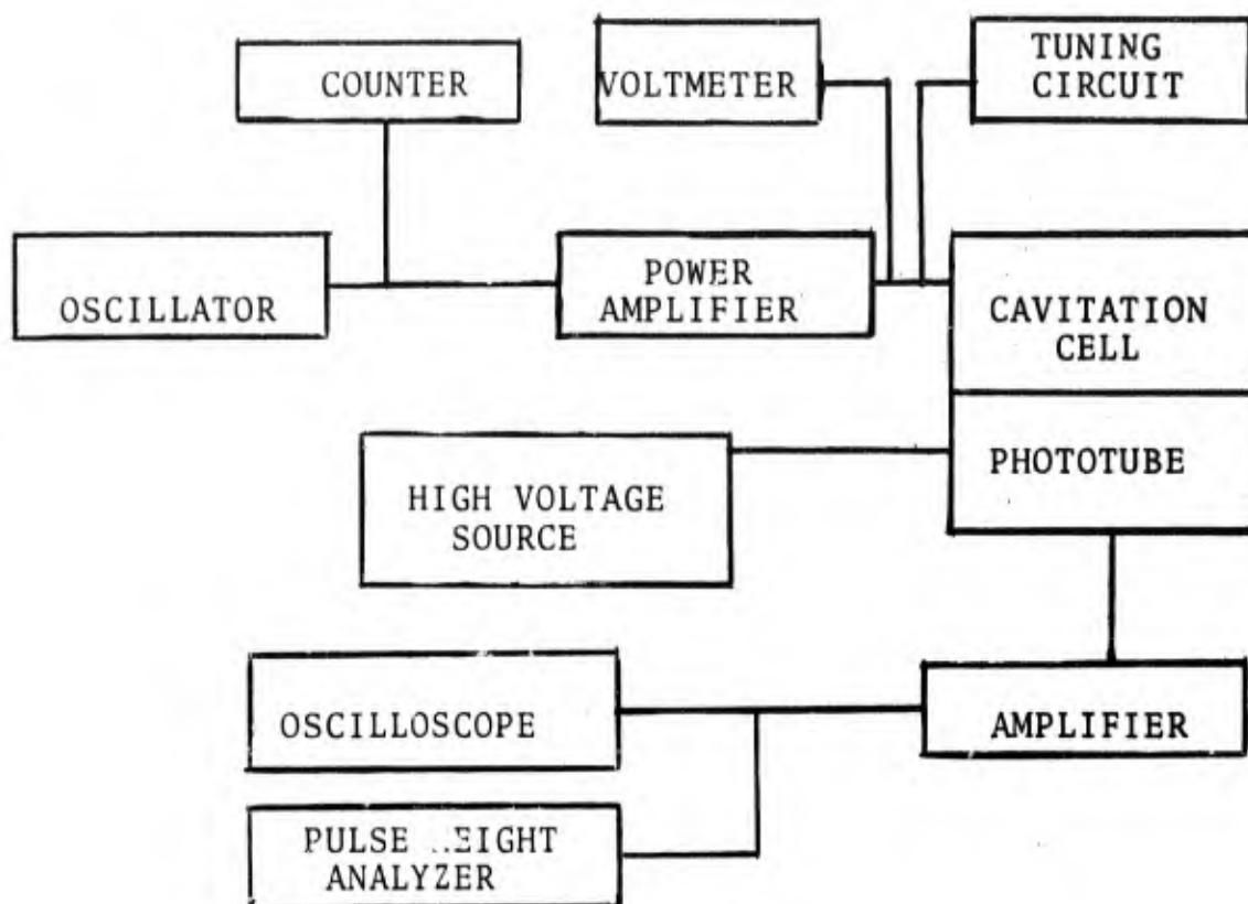
Figure 5, Schematic Block Diagram of the Experimental Apparatus
