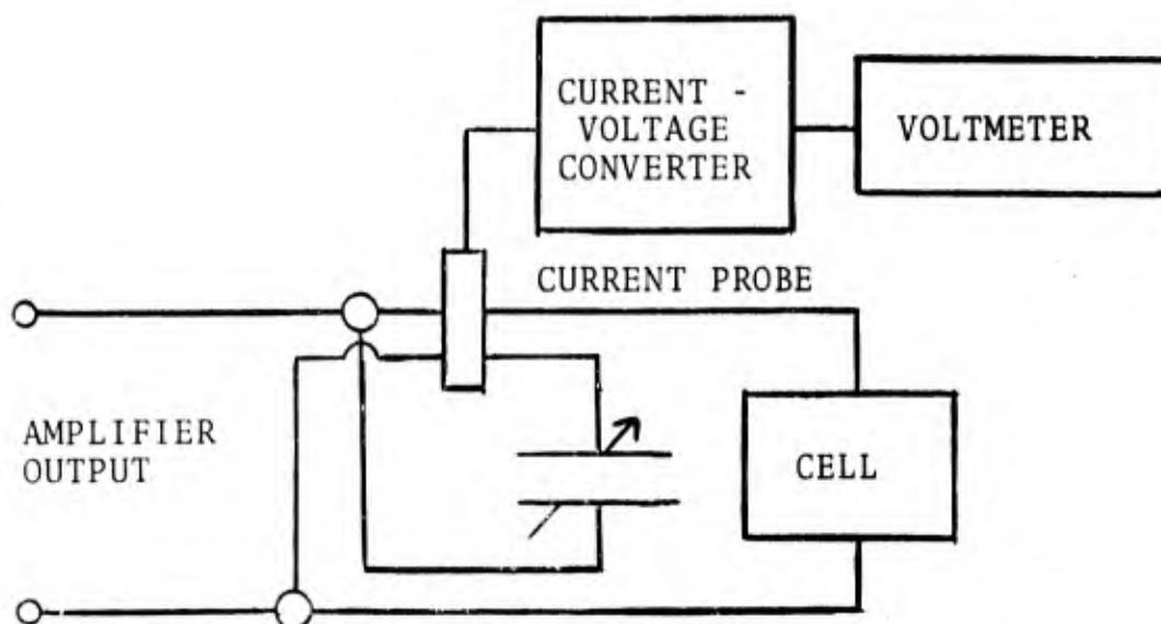
Figure 6, Schematic, Tuning Circuit
