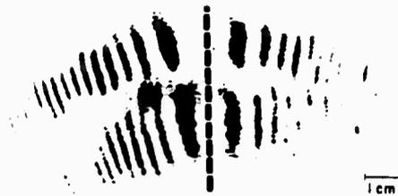
Figure 4. Actual Hologram of a Long Hole in an Aluminum Block
