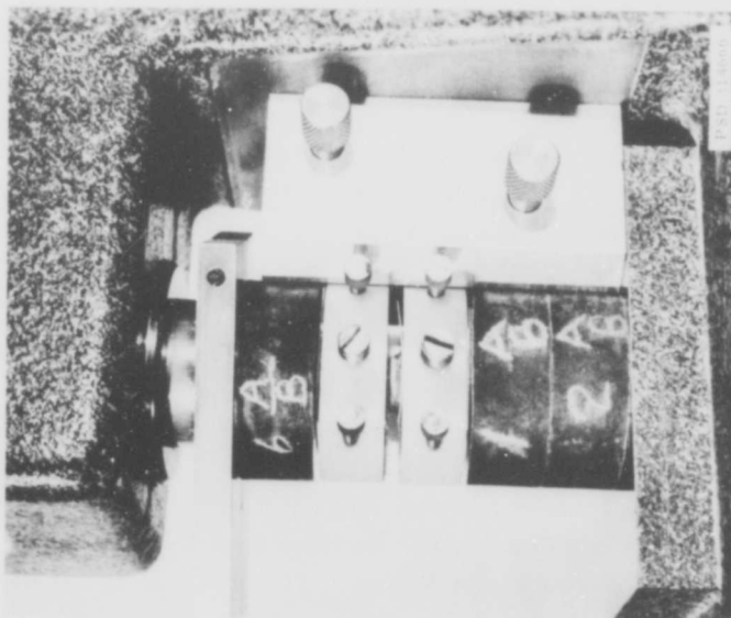
Figure A8 – Separable Precision Alignment Blocks and Specimen Alignment Jig under Center of Compression Subpress
