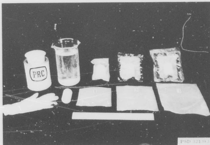
Figure A20 -- Triple Plastic Bag Filled with Artificial Sea Water
