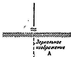
Figure V.20.1. Unbalanced vertical dipole with mirror image.
