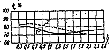
Figure XIII.10.22. Dependence of the efficiency of the RGD 65/4 1 antenna on the wavelength. W_r = 700 ohms.
