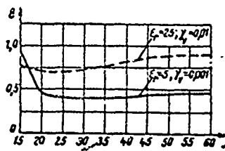
Figure X.3.2. Dependence of the gain factor for an unbalanced dipole ( l = 10 m) on the wavelength for wet ( \epsilon_r = 25 ; \gamma_v = 0.01 ) and dry ( \epsilon_r = 5 ; \gamma_v = 0.001 ) soil.
