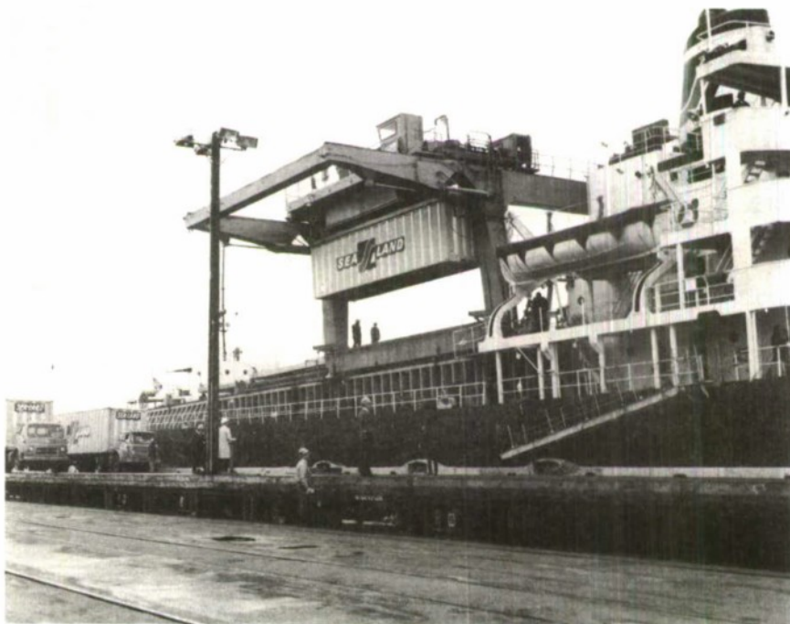
Figure 20. Container Being Moved Inboard to Hatch Cell.
