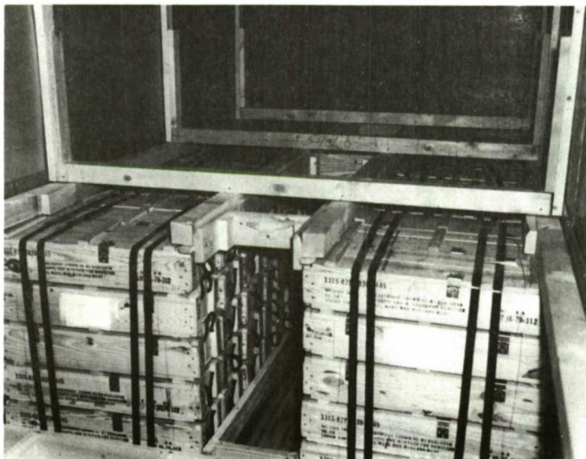
Figure 14. Container Number 59762, 2- by 6-Inch Spreader Missing.
