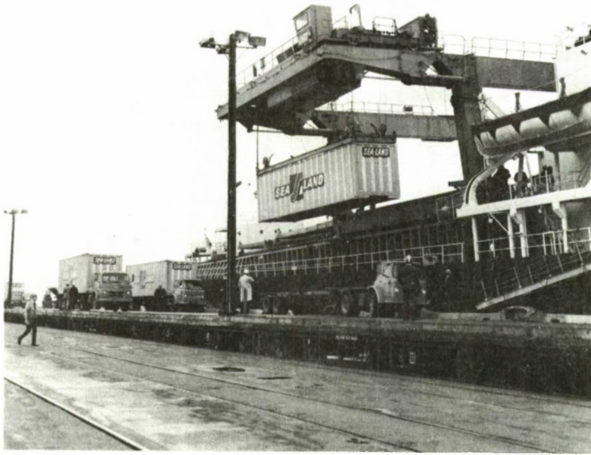
Figure 17. Aft Gantry Crane Lifting Container Aboard; Other Containers Being Moved Forward by Truck Tractor for Loading.
