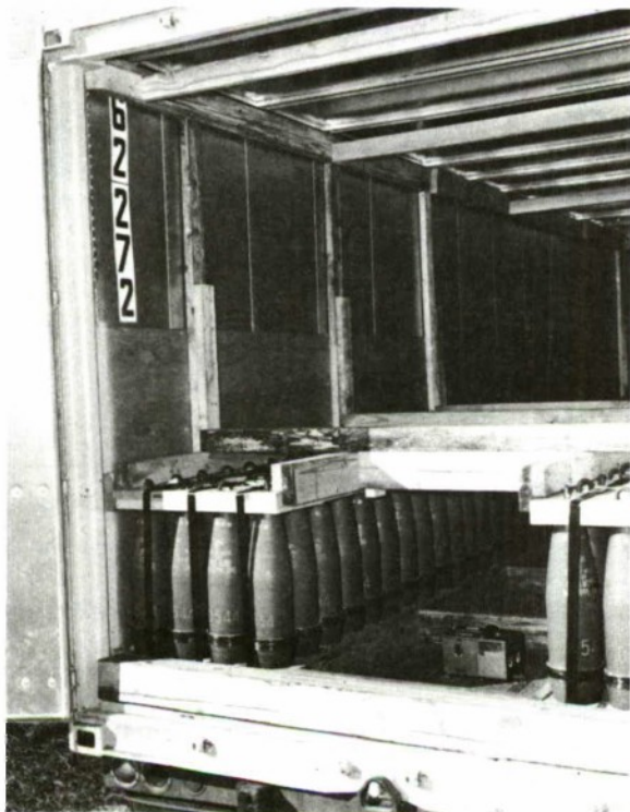
Figure 29. A Mechanical, Three-Directional Accelerometer Mounted Near Door Opening in Container Number 62272, Which Was Stuffed With 155-Millimeter Ammunition.
