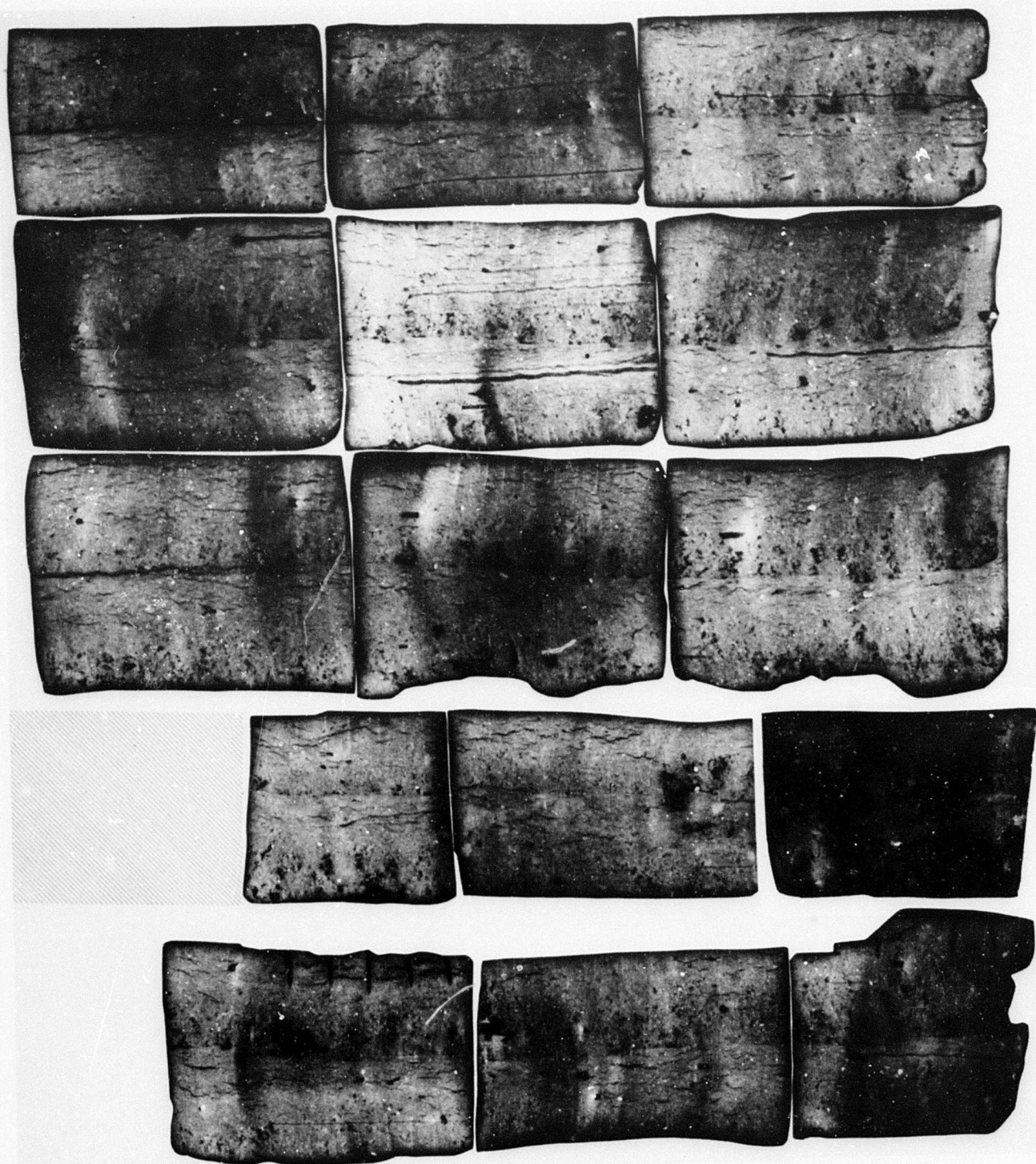
Fig. 44. Radiograph of soil deformation pattern, Test 3; H/B = 3, P_s = 37.5 \text{ psi}
