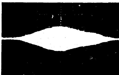
FIG. 24 OSCILLOGRAMS OF PRESSURE PROBE TRACES IN CATHODE COLUMN AT z = 2 CM AND VARIOUS LATERAL POSITIONS (ARGON, 1 ATM)
