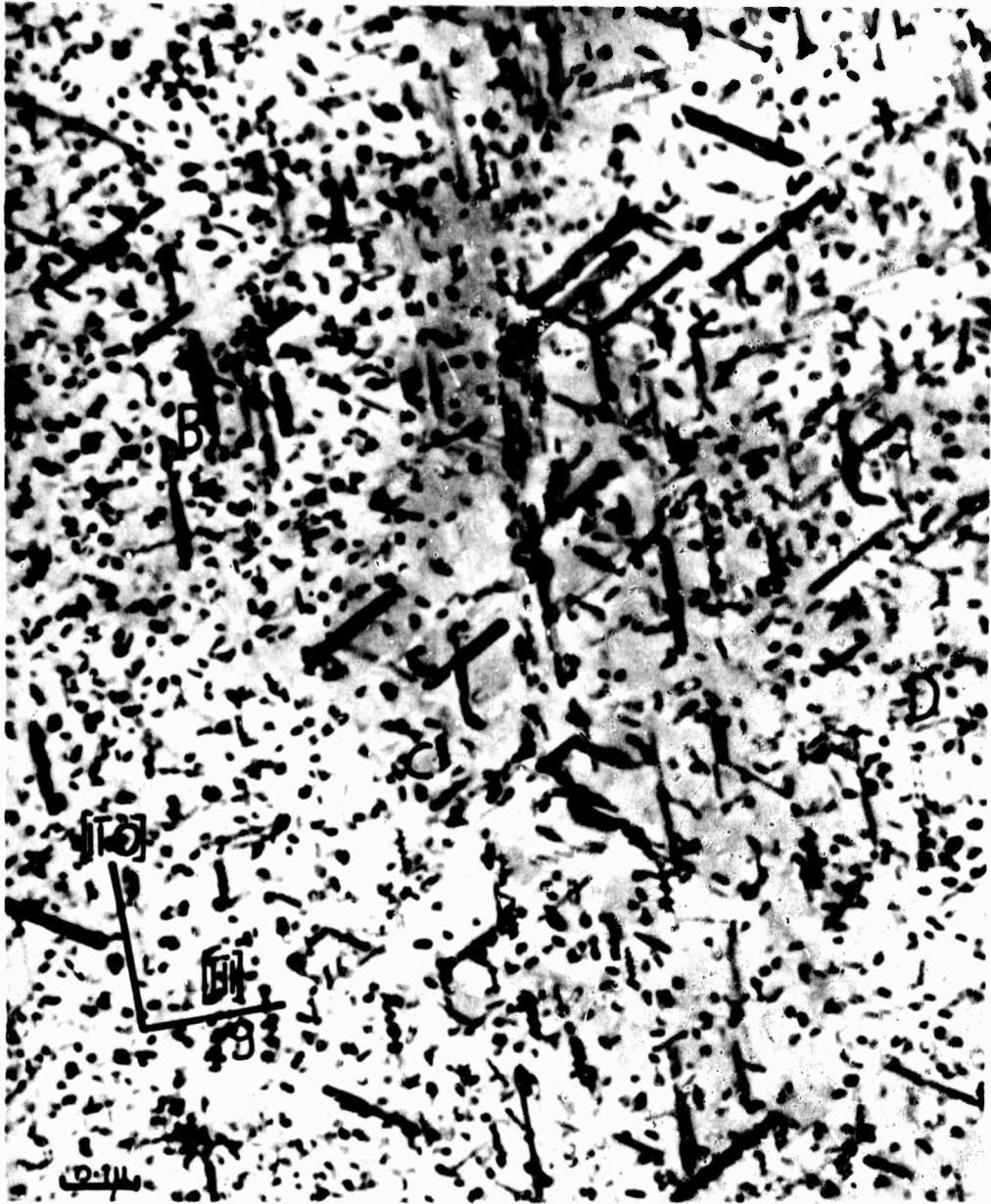
C. Displacement fringe contrast of type 1 precipitates
