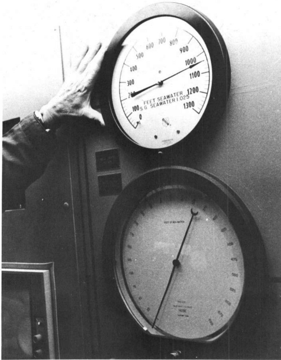
Depth gauge showing chamber pressure in feet of sea water during excursion dive to 1050 feet.
