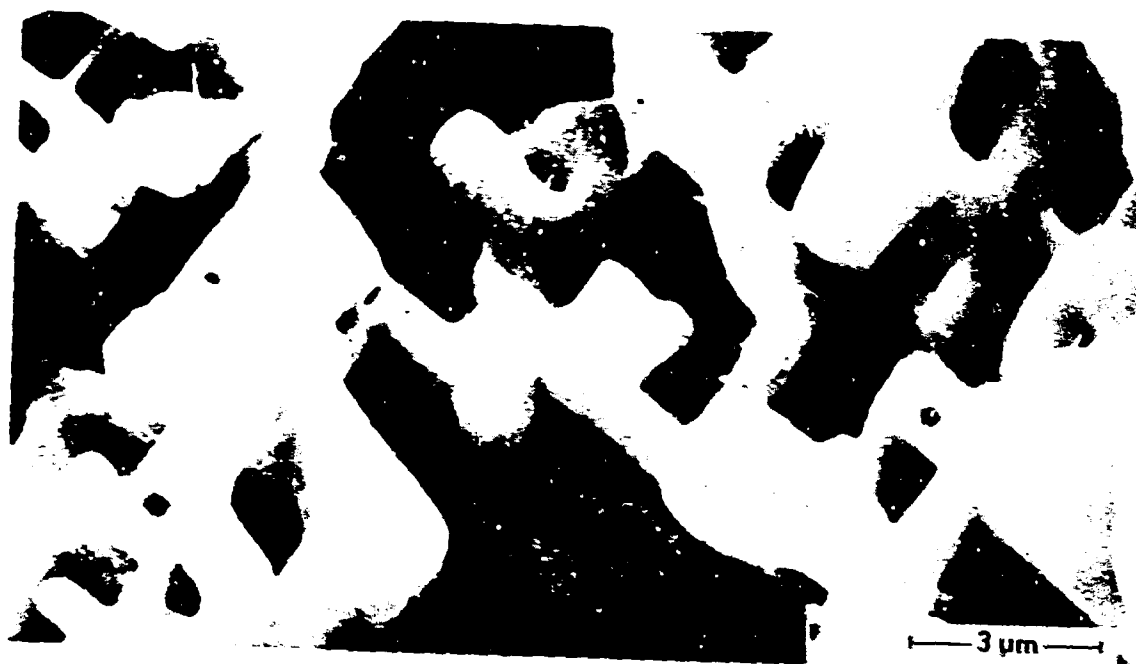
Low temperature decomposition at 230°C for 500 h
